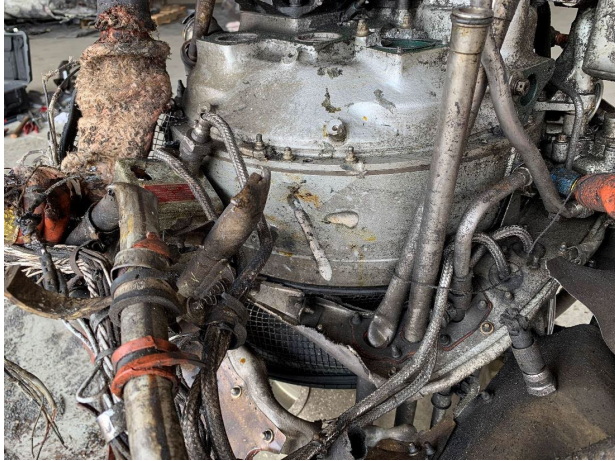
Figure 34. Damage to inlet case and engine externals
