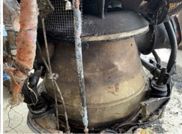
Figure 35. Gas generator case distortion
