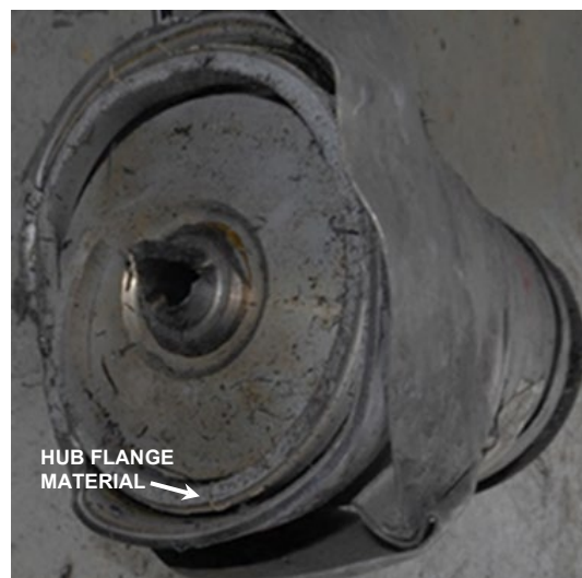
Figure 26. Hydraulic unit with liberated hub attachment flange
