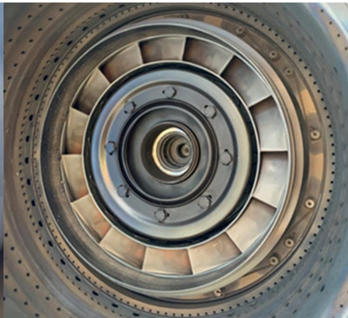
Figure 16. View of CT vane assembly downstream side after CT disk removal
