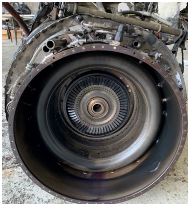
Figure 36. Left engine hot section showing combustor and CT disk assembly downstream face
