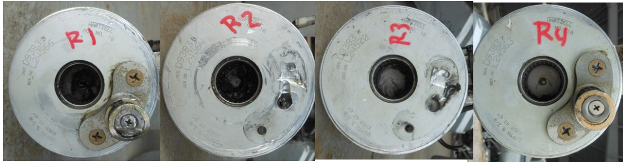
Figure 31. Right propeller blade butts, showing condition of pitch change knobs and bracket attachments
