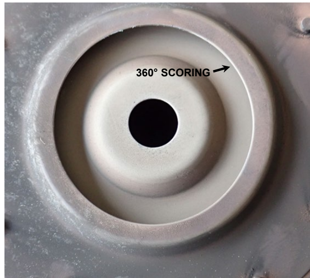
Figure 20. Upstream PT S1 vane ring 360° center baffle lip scoring
