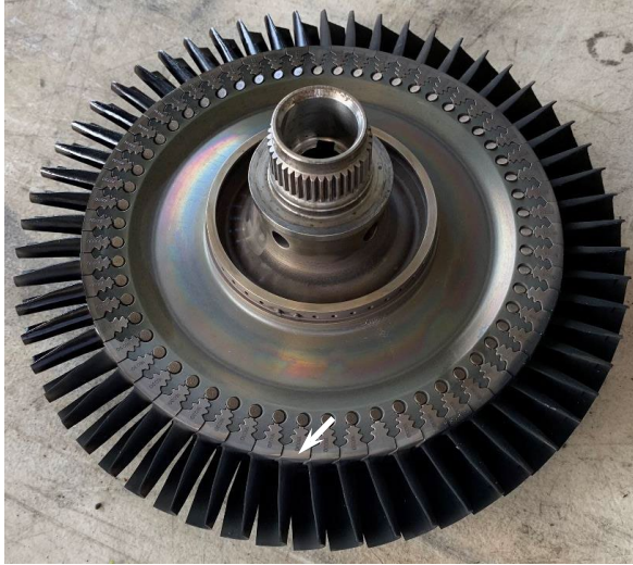
Figure 38. CT disk upstream face showing intermittent rub
