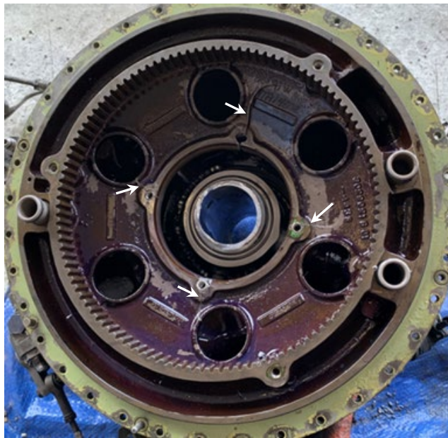
Figure 46. RGB front case with S2 planetary gear carrier removed showing cracked bearing retention bolt holes and propeller shaft fracture
