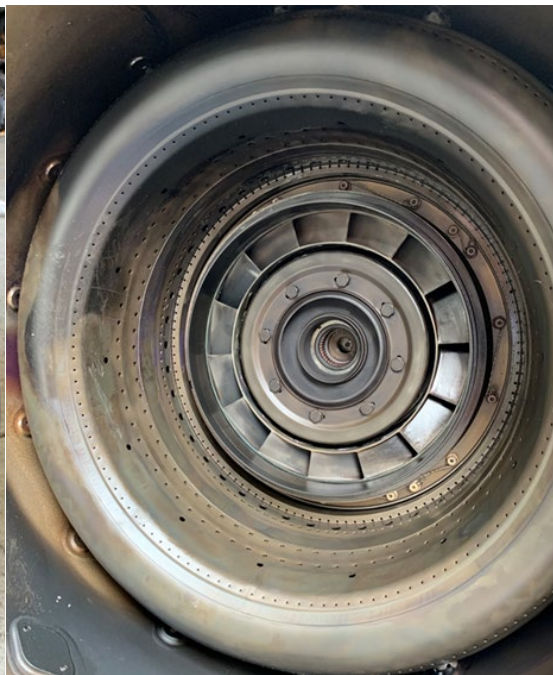
Figure 37. CT disk removed, exposing CT vane assembly downstream side
