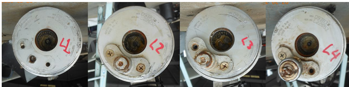
Figure 10. Left propeller blade butts, showing pitch change knob/bracket damage
