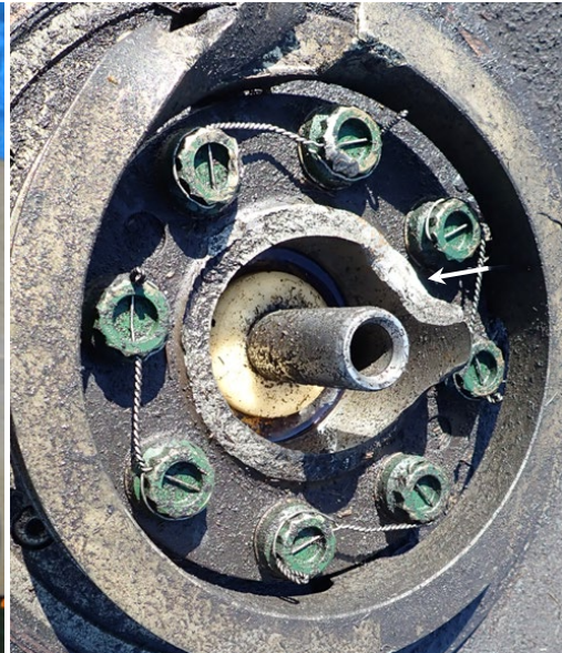
Figure 2. Engine propeller shaft, forward fracture surface
