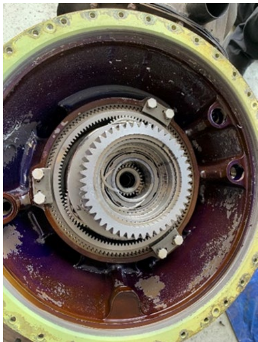
Figure 44. S1 planetary gearing showing S1 and S2 sun gears
