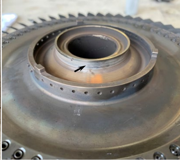
Figure 39. CT disk assembly downstream face bore lip scoring
