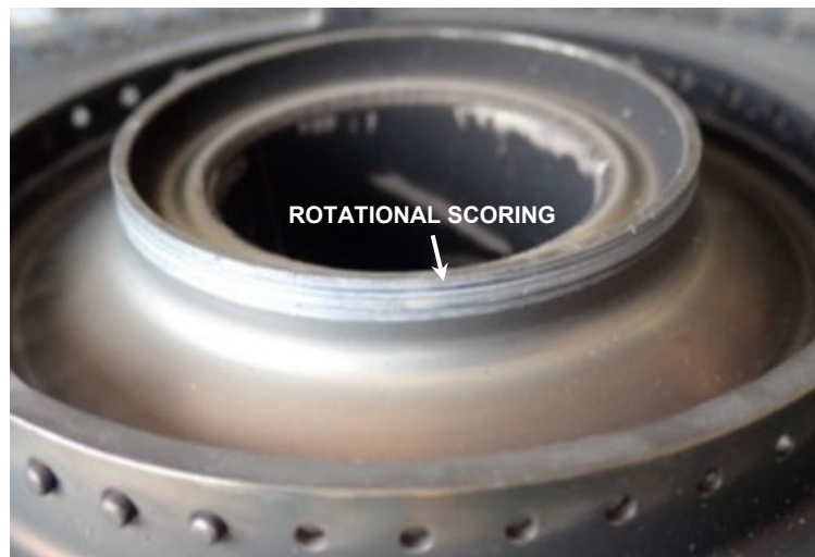
Figure 18. CT disk downstream face showing circumferential scoring to retaining bolt bore lip
