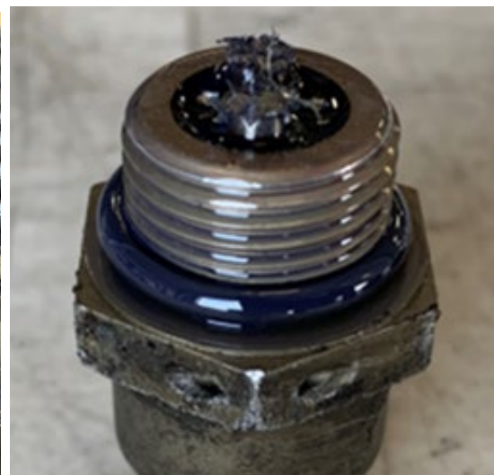
Figure 43. Ferrous debris on RGB plug
