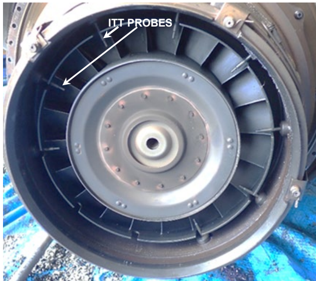
Figure 19. Upstream side of PT S1 vane assembly in PT stator housing. ITT probes are shown.
