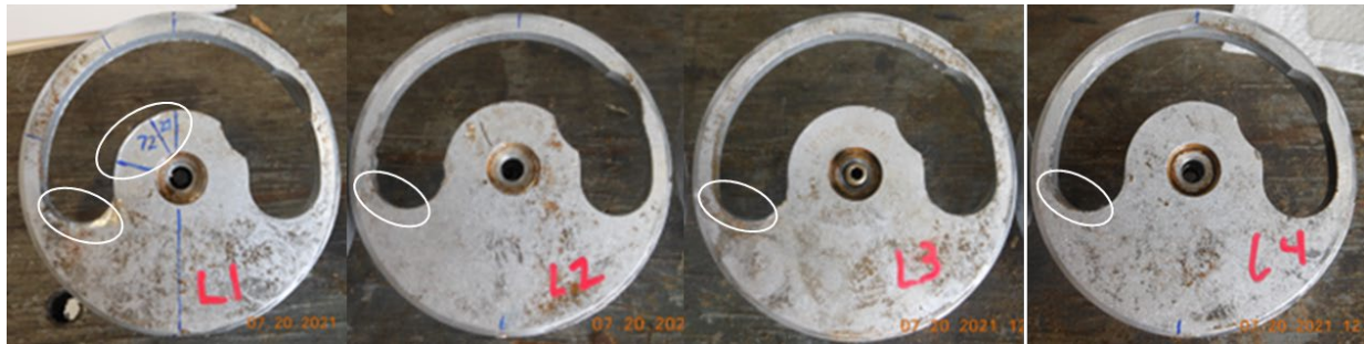
Figure 11. Left propeller preload plates showing knob impact marks at the low pitch slot ends and L1 fork/bracket impact marks
