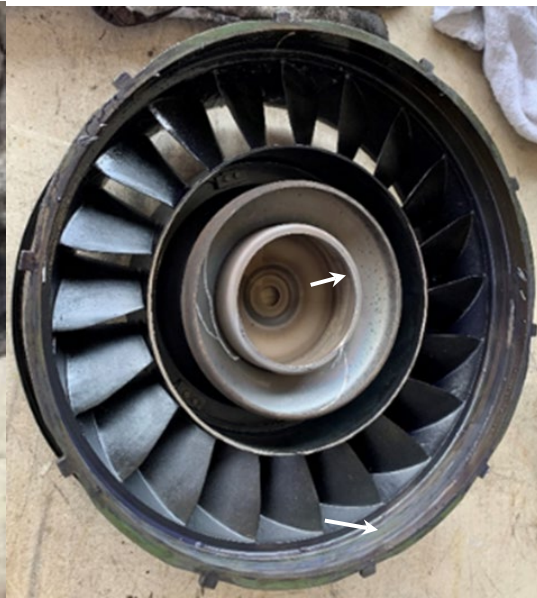
Figure 41. PT S1 vane ring downstream side showing rub along the center baffle edge and arc or scoring along the shroud/blade path
