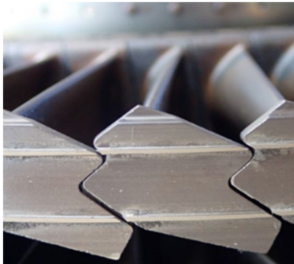
Figure 23. PT S1 blade tip knife edge wear
