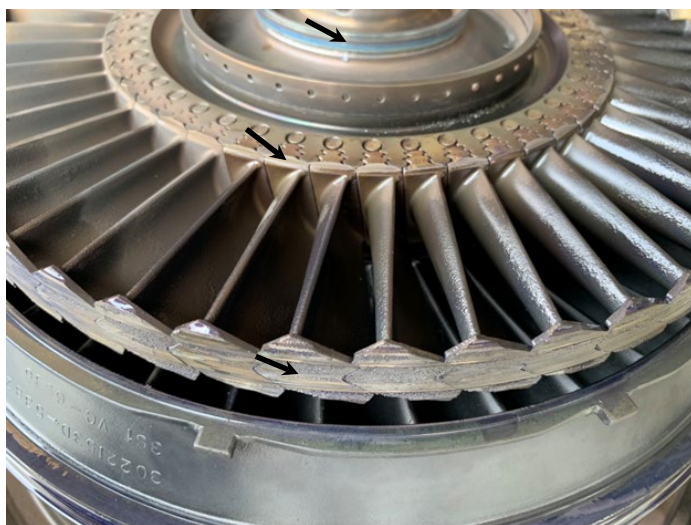
Figure 42. PT S1 disk assembly showing 360° scoring
