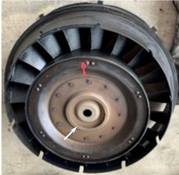
Figure 40. PT S1 vane ring upstream side showing inner baffle rub
