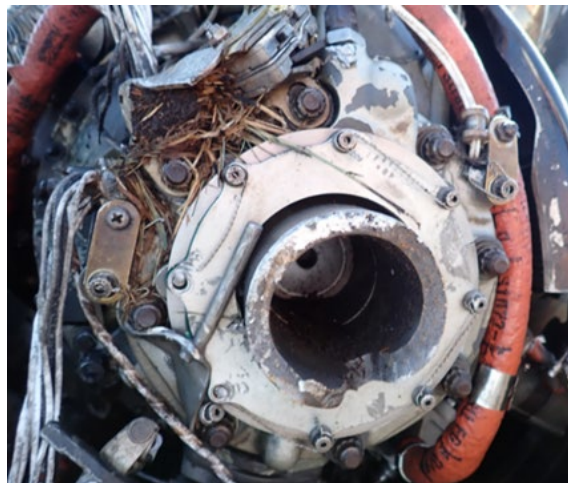
Figure 14. Engine propeller shaft fracture surface
