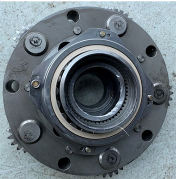
Figure 47. Forward side of S2 planetary gear carrier showing flanged bearing assembly and propeller shaft separation fracture
