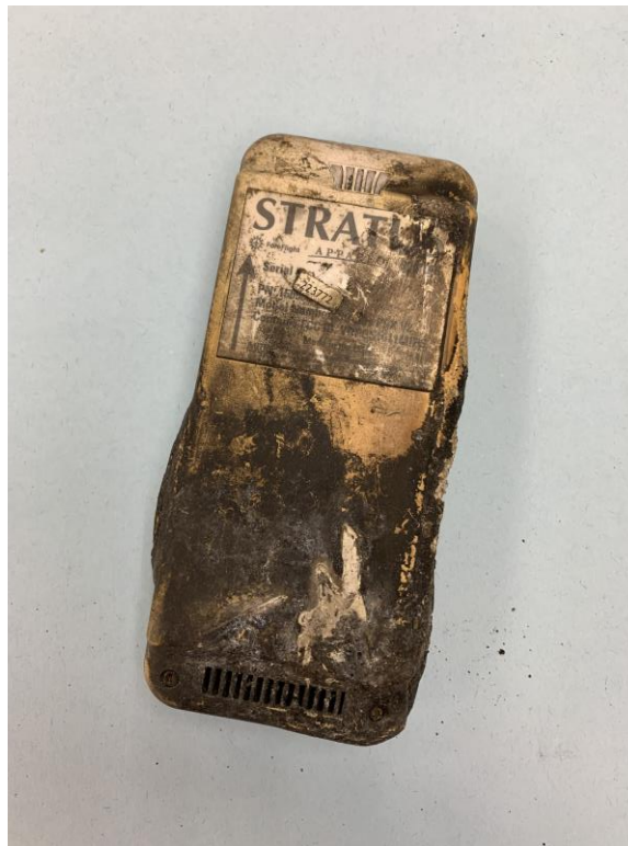
Figure 1. Photo of fire damaged Appareo Stratus unit, as received.
