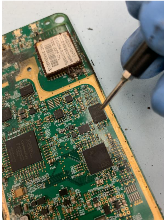
Figure 2. Photo of the device's internal NVM memory prior to being removed and read.
