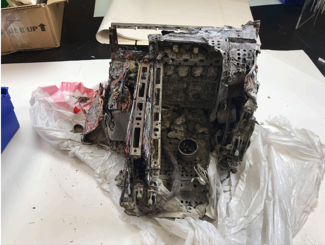
Figure 3. As received condition of Avidyne PFD.
