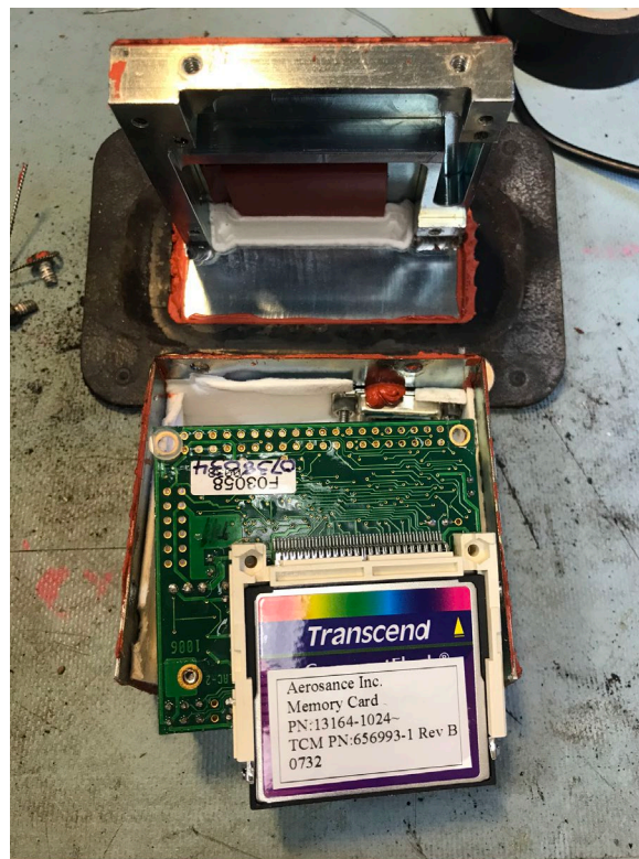
Figure 2. Internal circuit board of RDM showing undamaged CF card.
