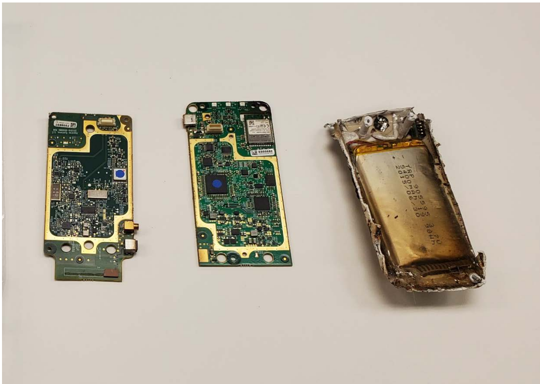
Figure 2. Appareo Stratus 2S disassembled revealing undamaged silicon components.
