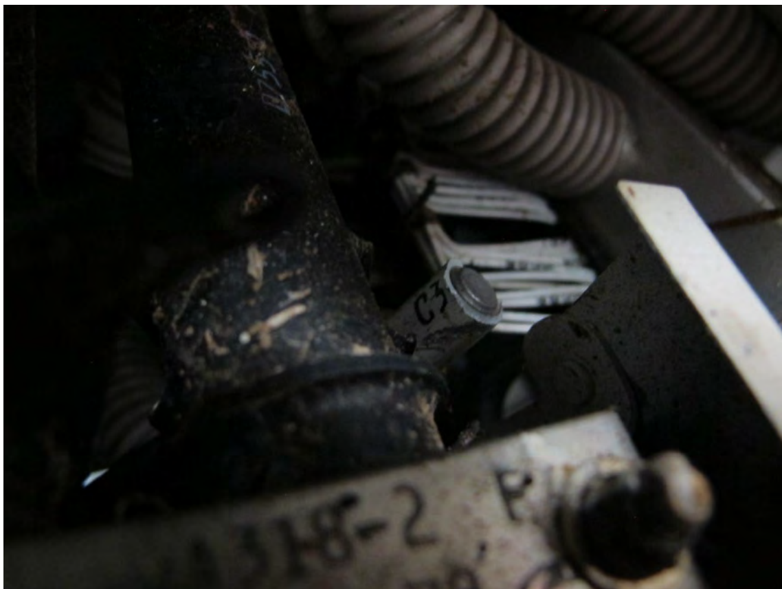
Disconnect TA at forward end of C343-9 push pull tube.
