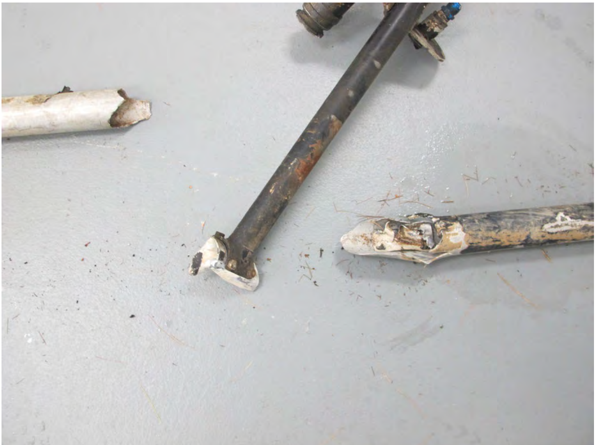
Disconnects at right skid and front right strut.
