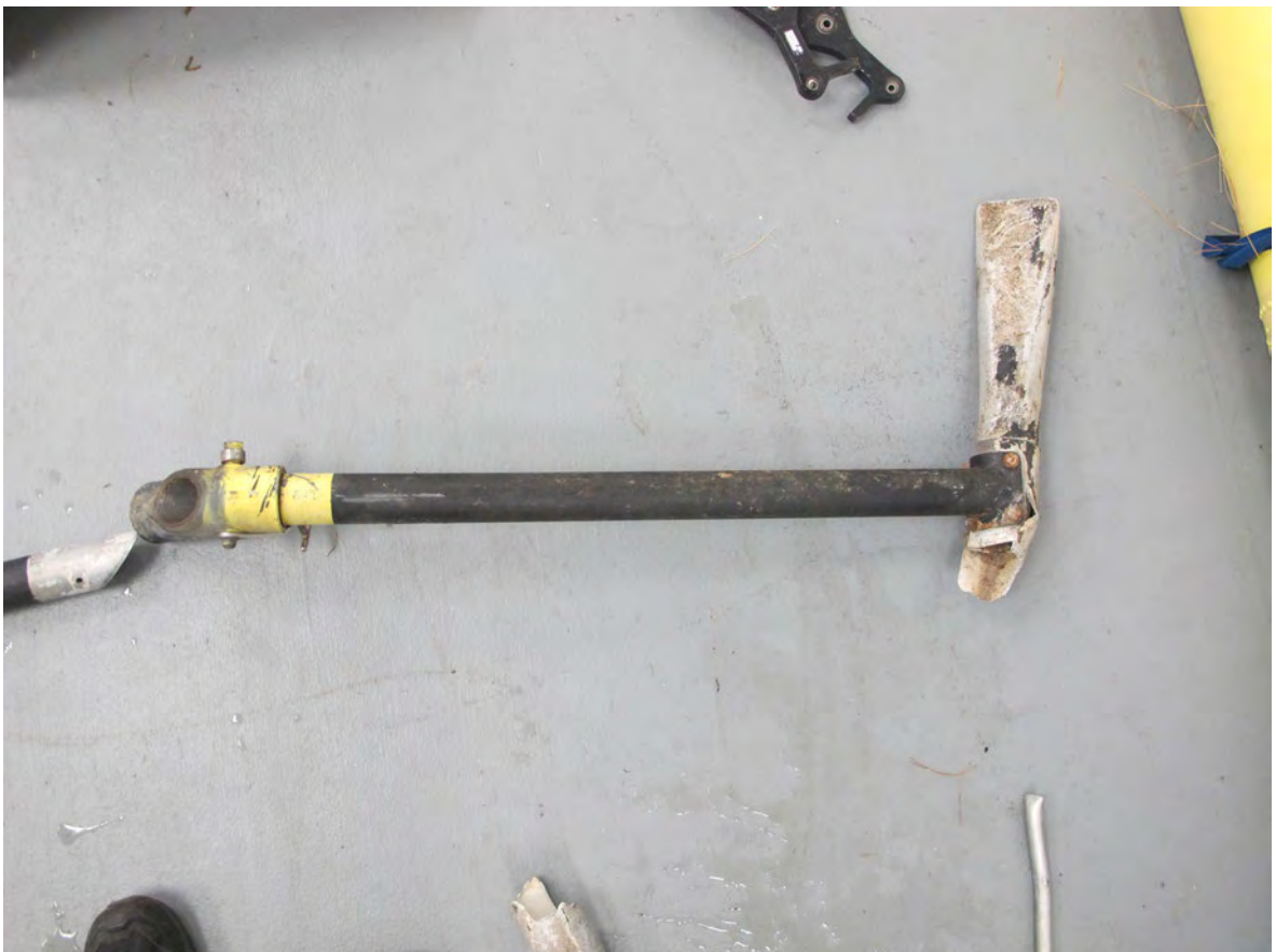
Aft left strut and left skid heel.
