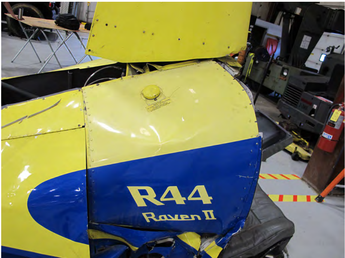
The auxiliary fuel tank.
