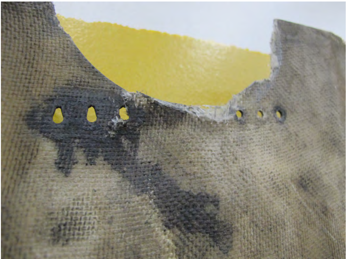
Mounting area on inside of scroll for lower bracket.
