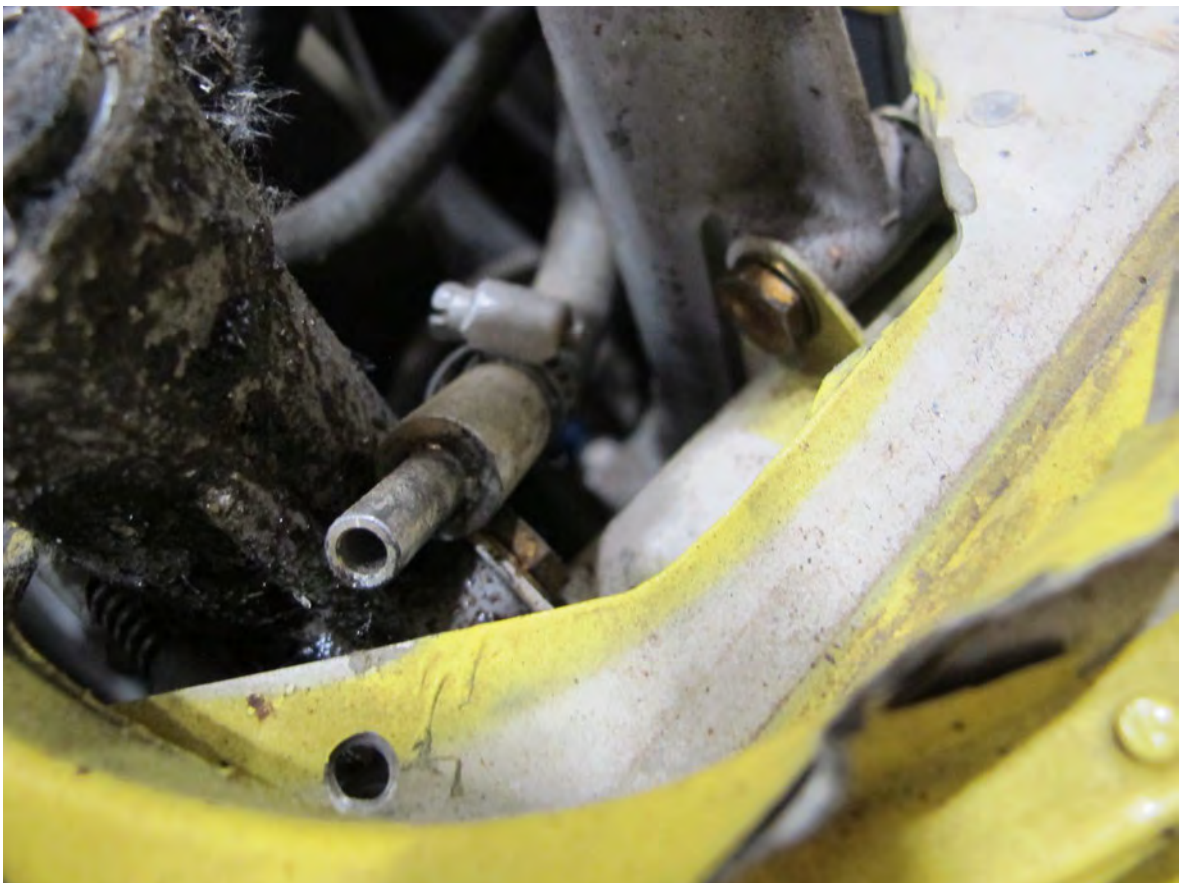
Main fuel tank fuel tank rollover valve.
