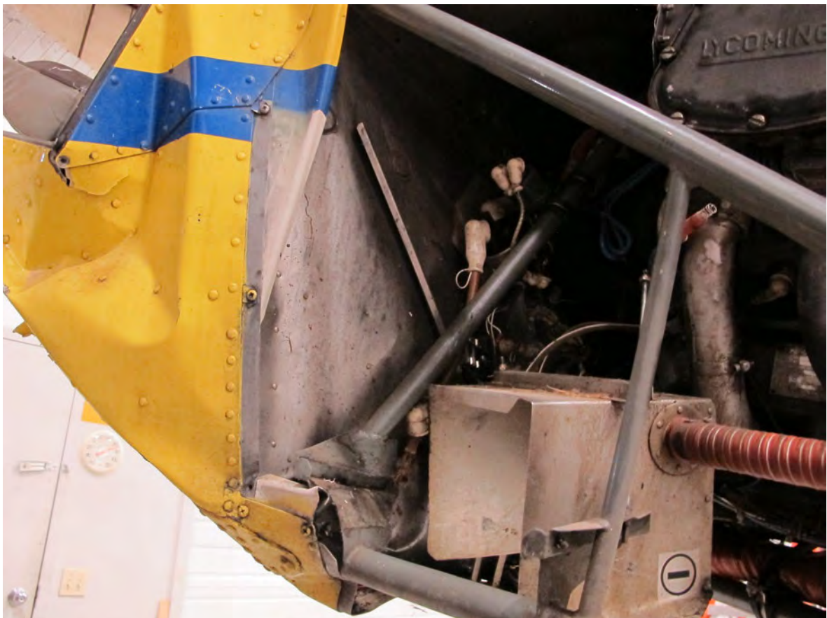
Vertical firewall, left side.
