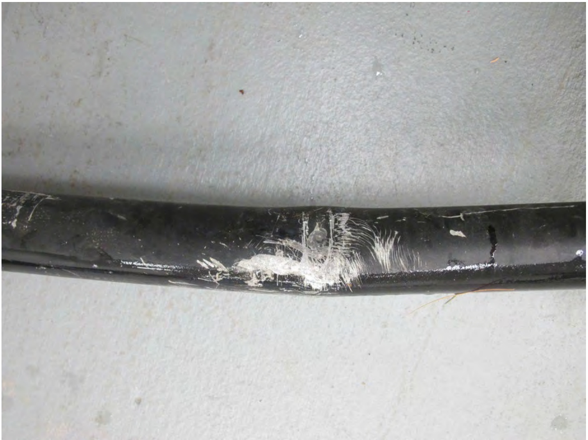
Damage to aft cross tube.
