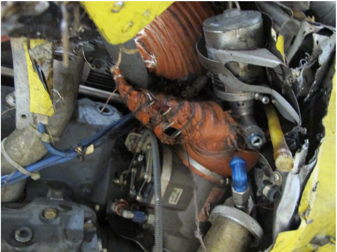
Fuel control unit. Note orange intake duct.
