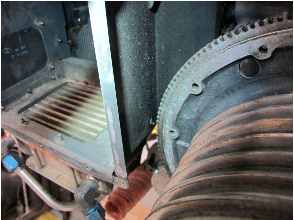
No contact between starter ring gear and cooling panel on right side.
