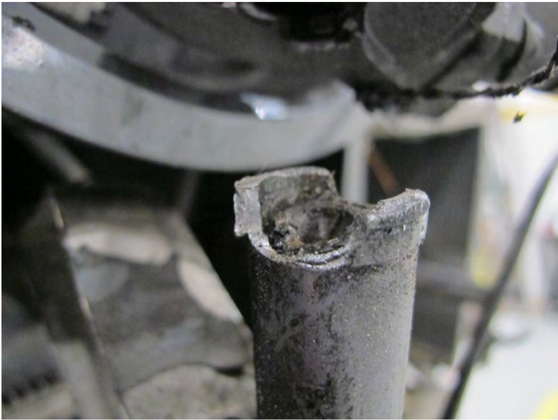
Surface of disconnect in belt tension actuator.
