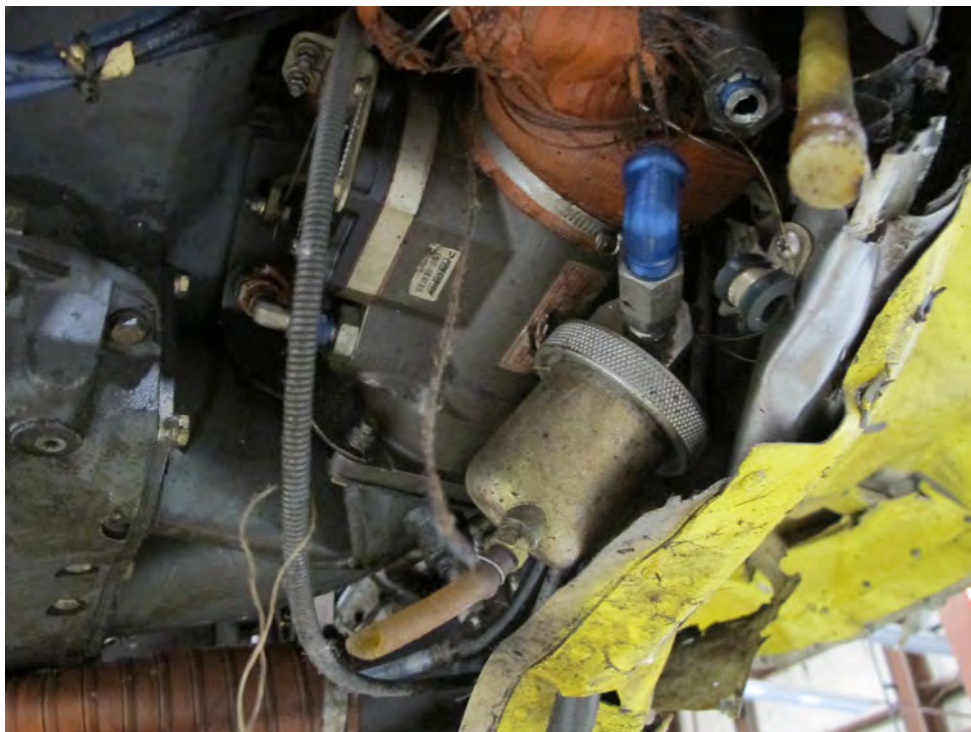
Gascolator and disconnect in fuel fitting.
