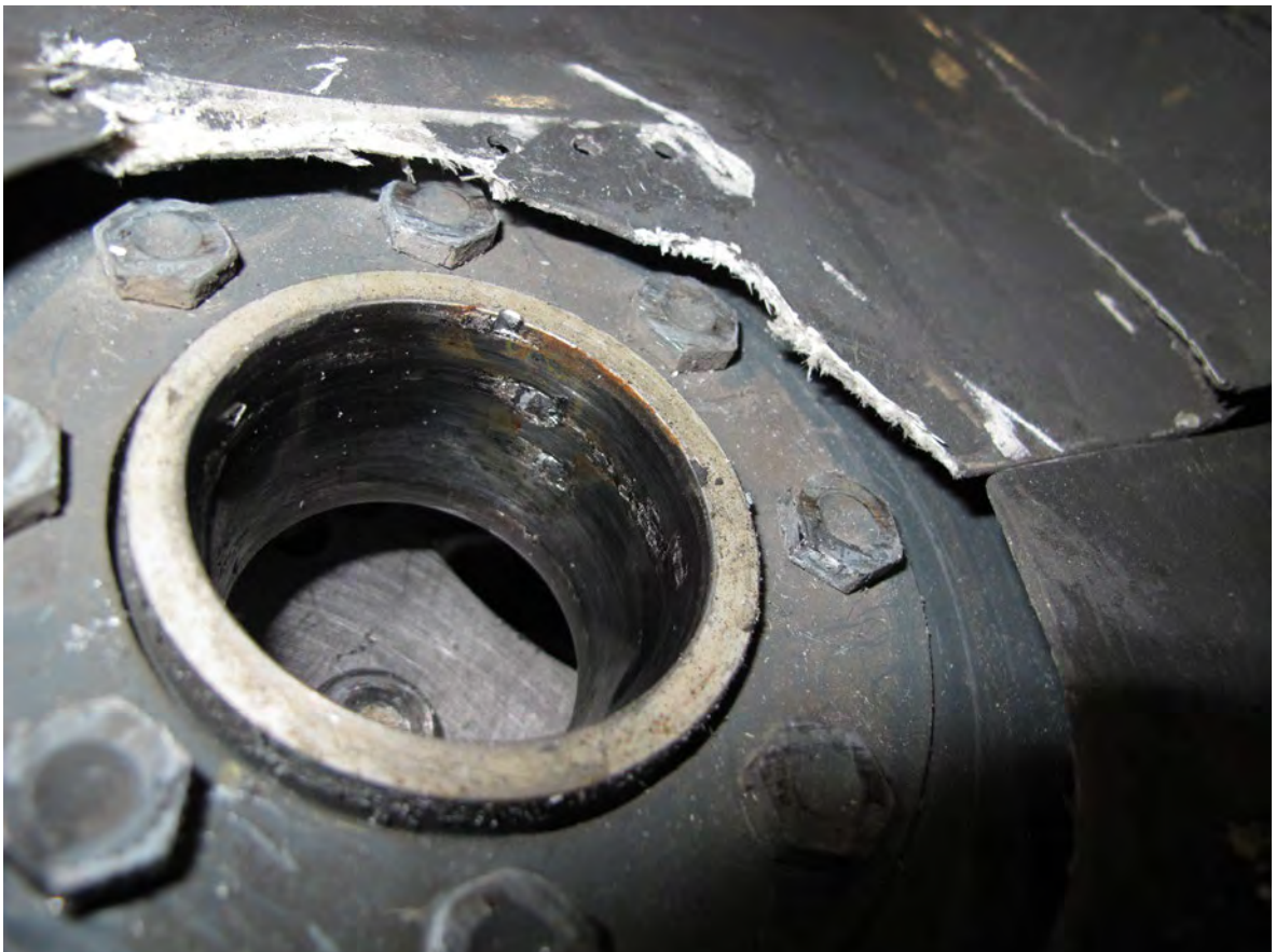
Above and below: Galling on fan shaft and in fan hub after removal of fan.
