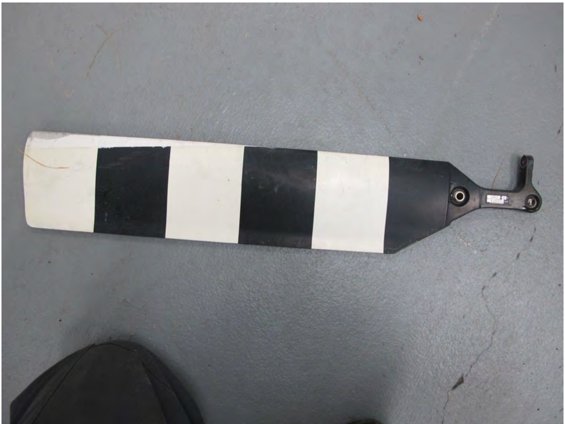
Above and below: Tail rotor blades.
