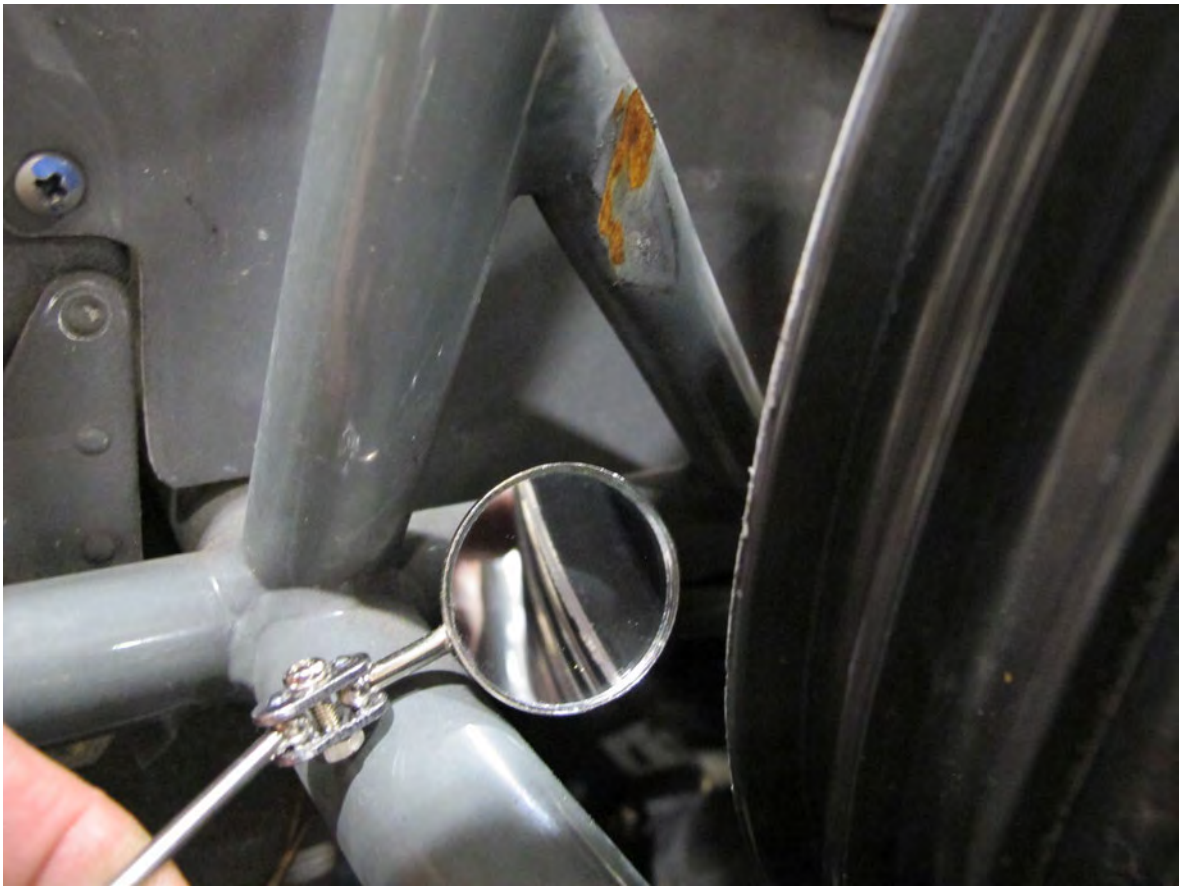
Above and below: Scoring on airframe adjacent to the forward face of the upper sheave.
