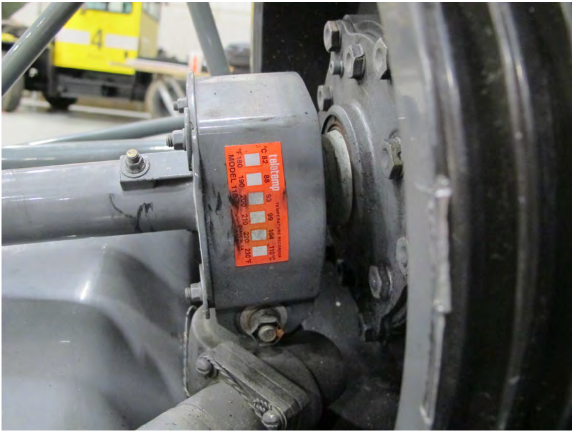
Upper belt tension actuator support bearing.
