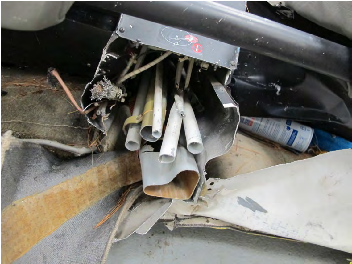
Above and below: Flight control tubes cut during recovery.
