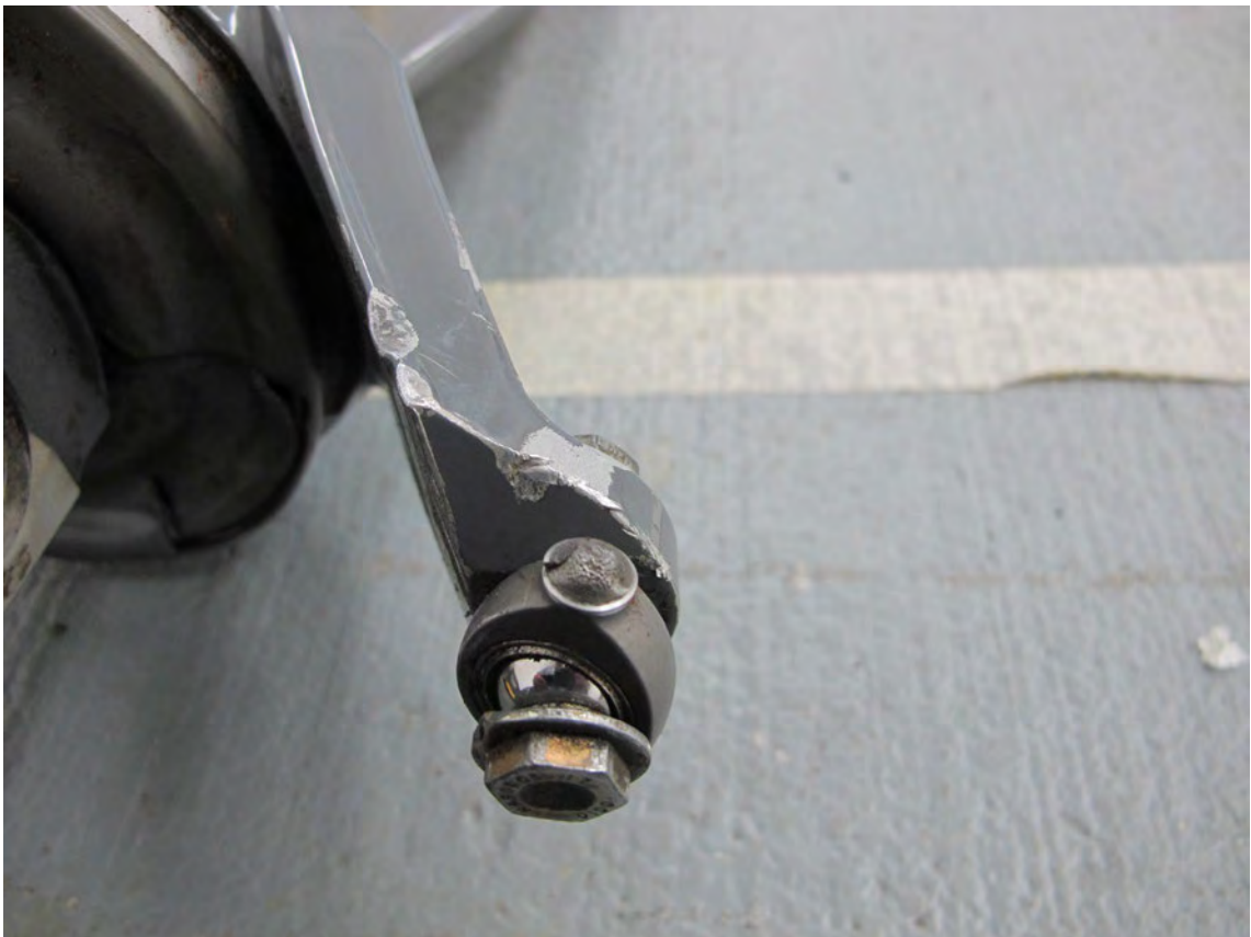
Above and below: Disconnect C in main rotor pitch link.
