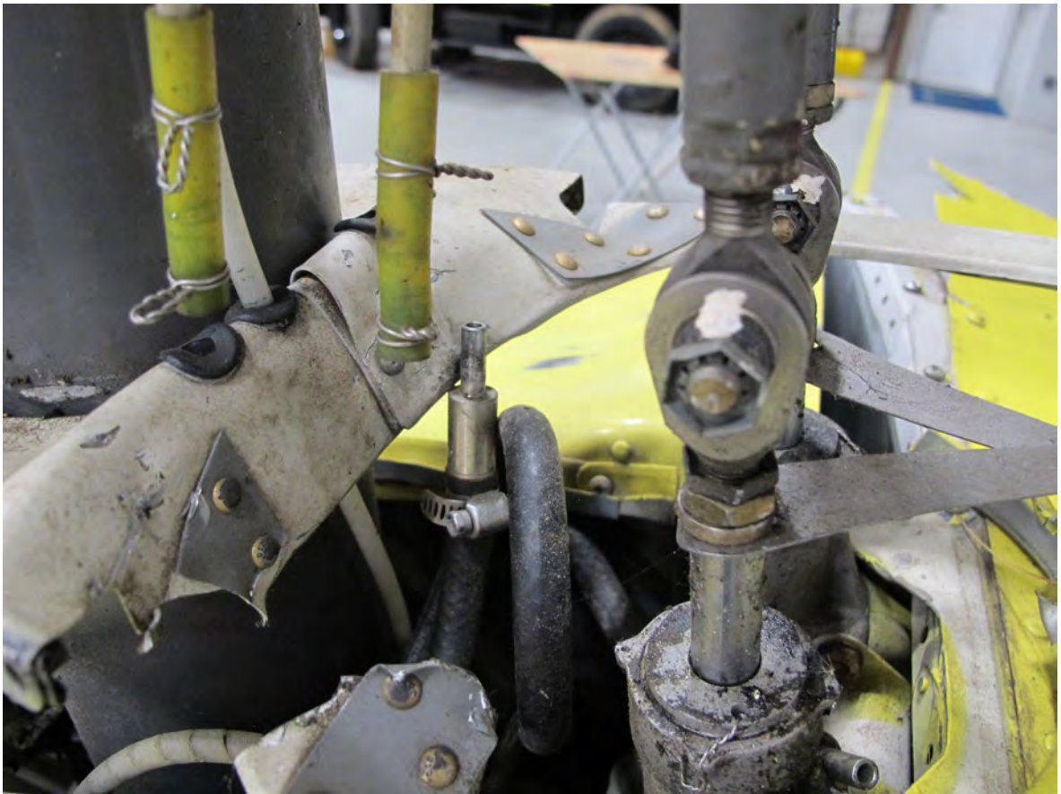
Fuel system vent hoses and tubes with auxiliary fuel tank rollover valve.
