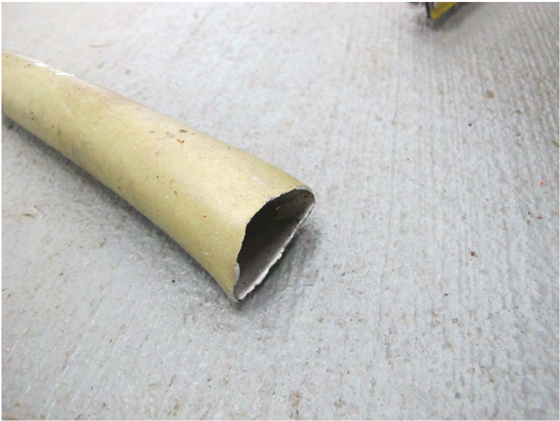
Disconnect A in C319-3 torque tube.
