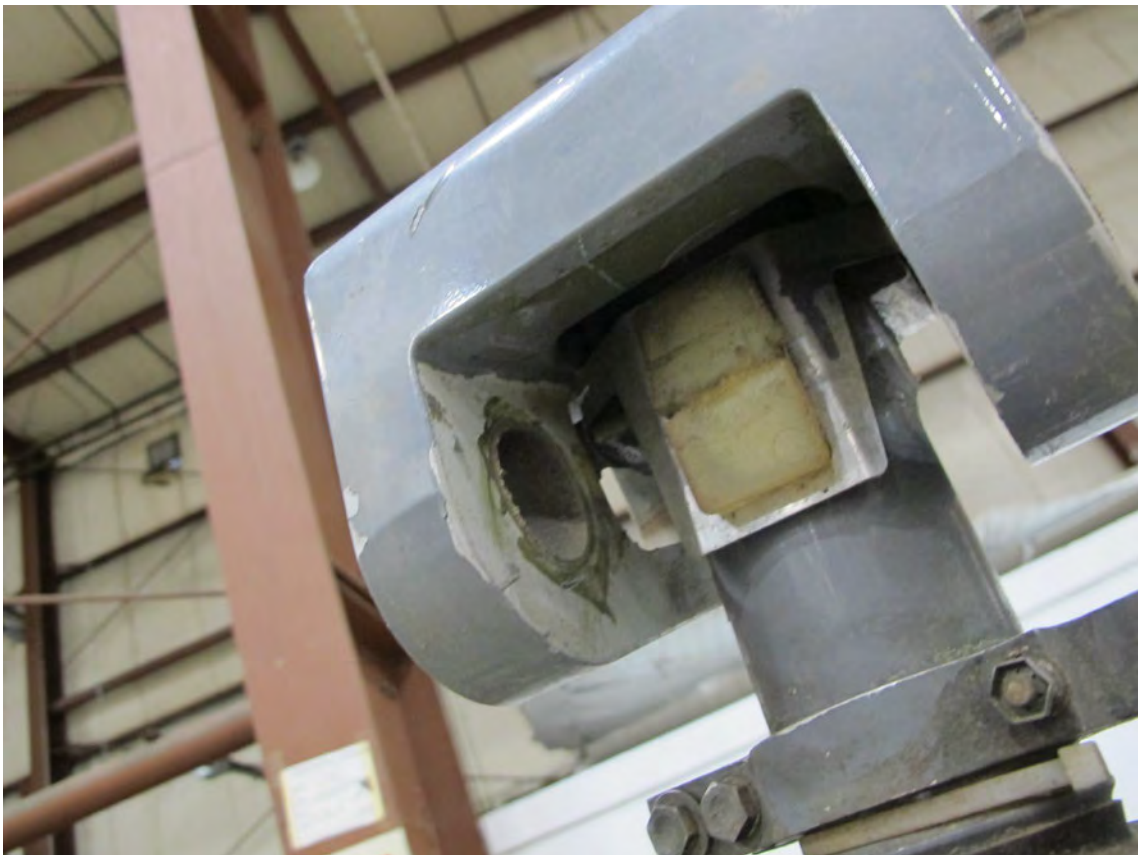
Teeter stop for main rotor blade SN 6318.
