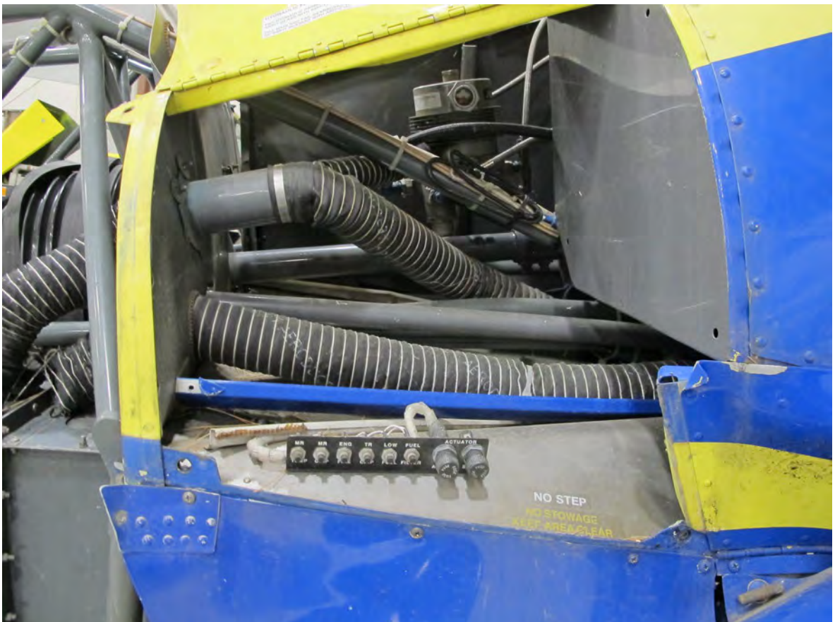
Aft horizontal firewall.
