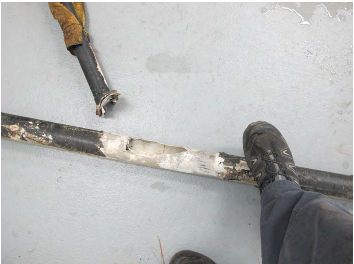
Disconnect at front left strut and left skid.
