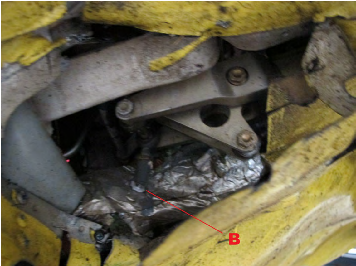
Disconnect B in left C121-28 push pull tube.
