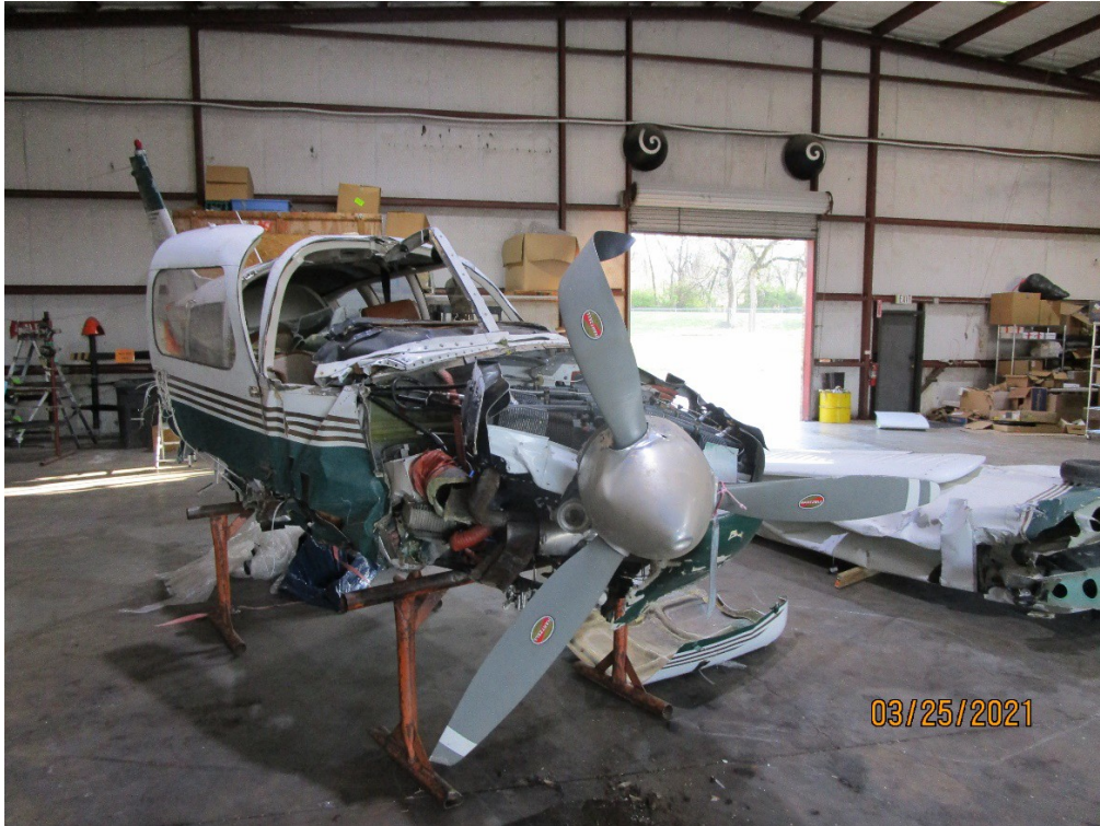
Damage to the three bladed propeller
