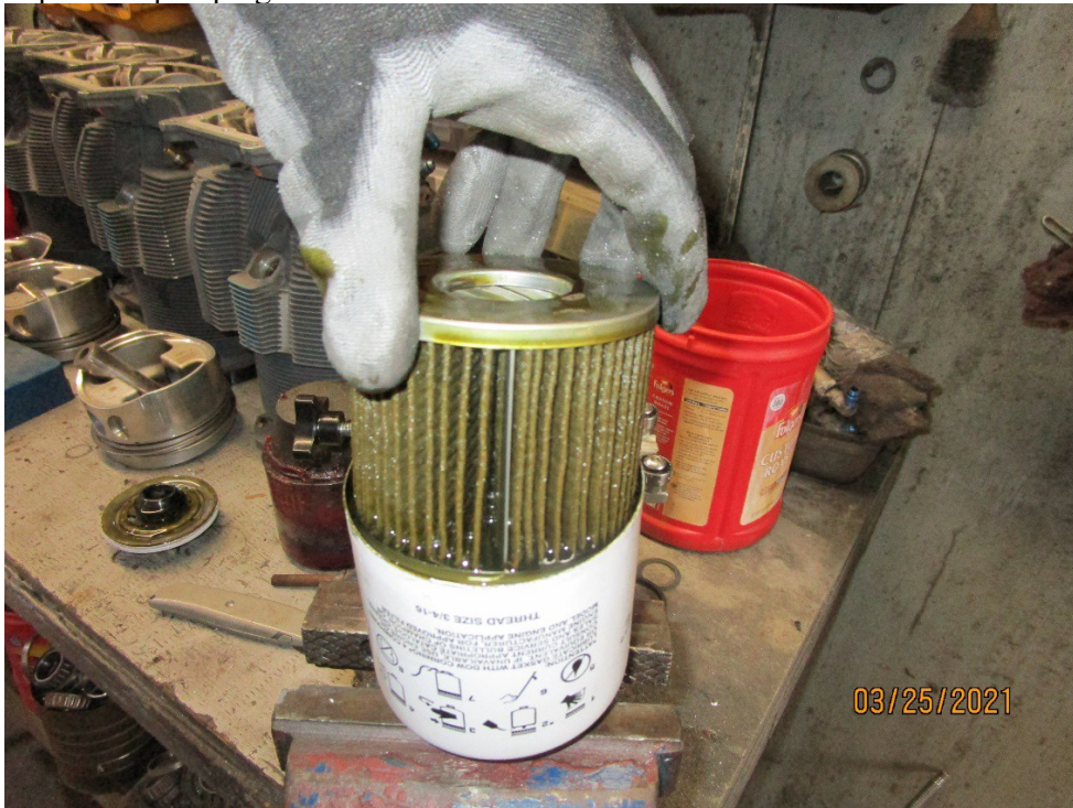
Oil filter, cut open and element inspected.
