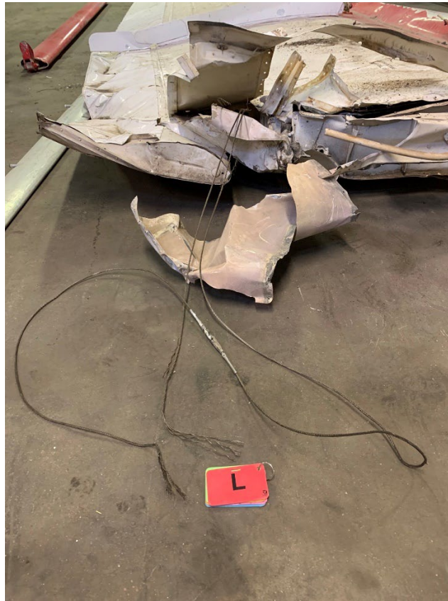
Figure 2. Left Wing Aileron Cables
