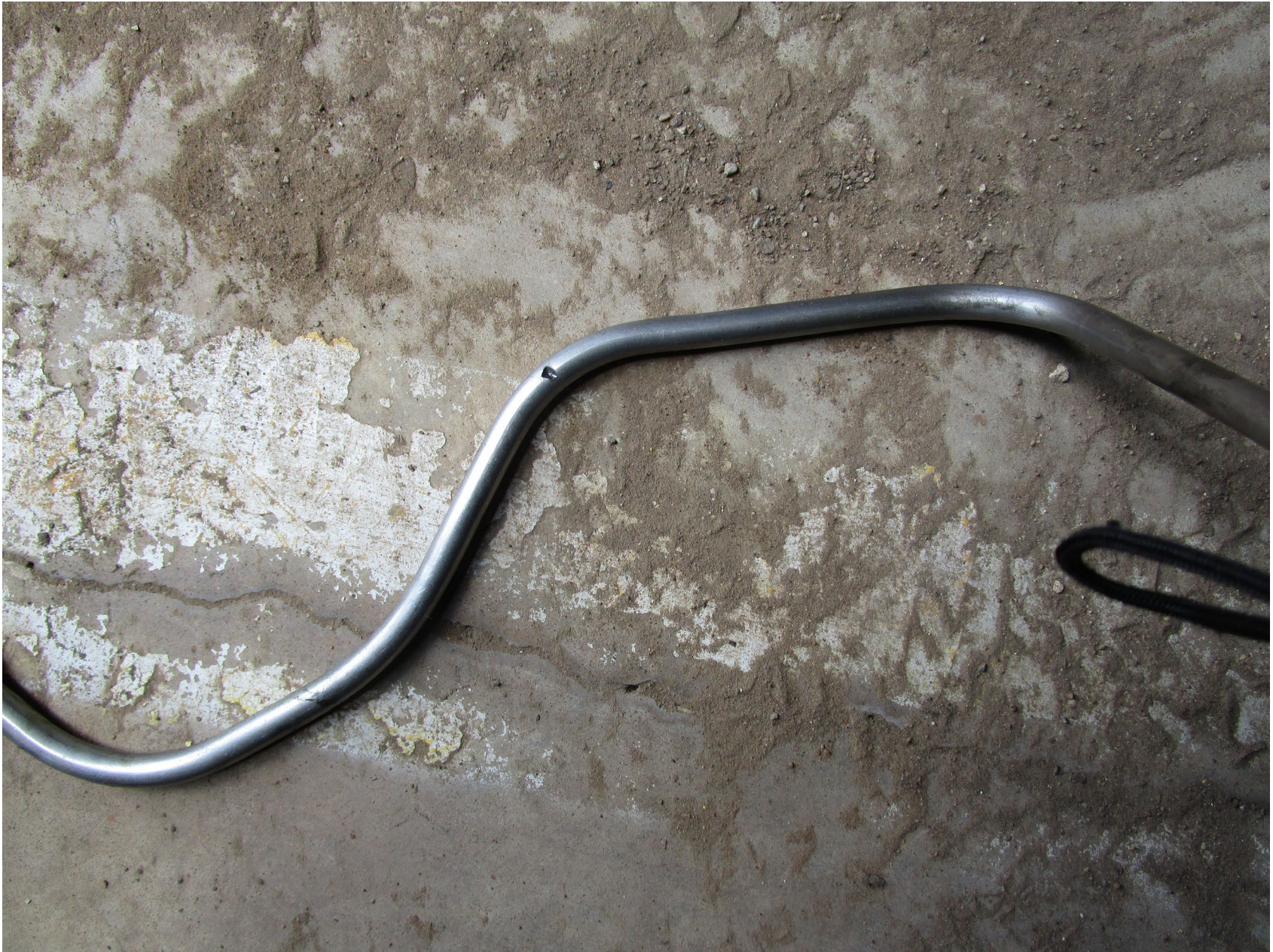
Photo 4 – Chaffed Oil Line
