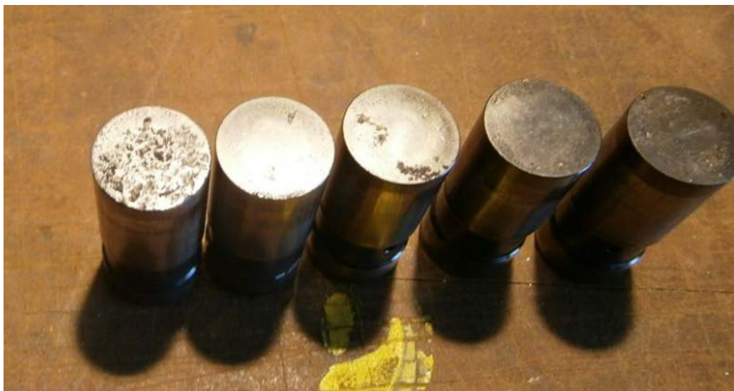
Figure 3 - Spalled TCM Continental hydraulic valve lifters P/N 653877, Note that P/N 653877 is not currently identified as a mandatory replacement in TCM MSB09-8A which states that lifter failures can present a safety of flight issue.
