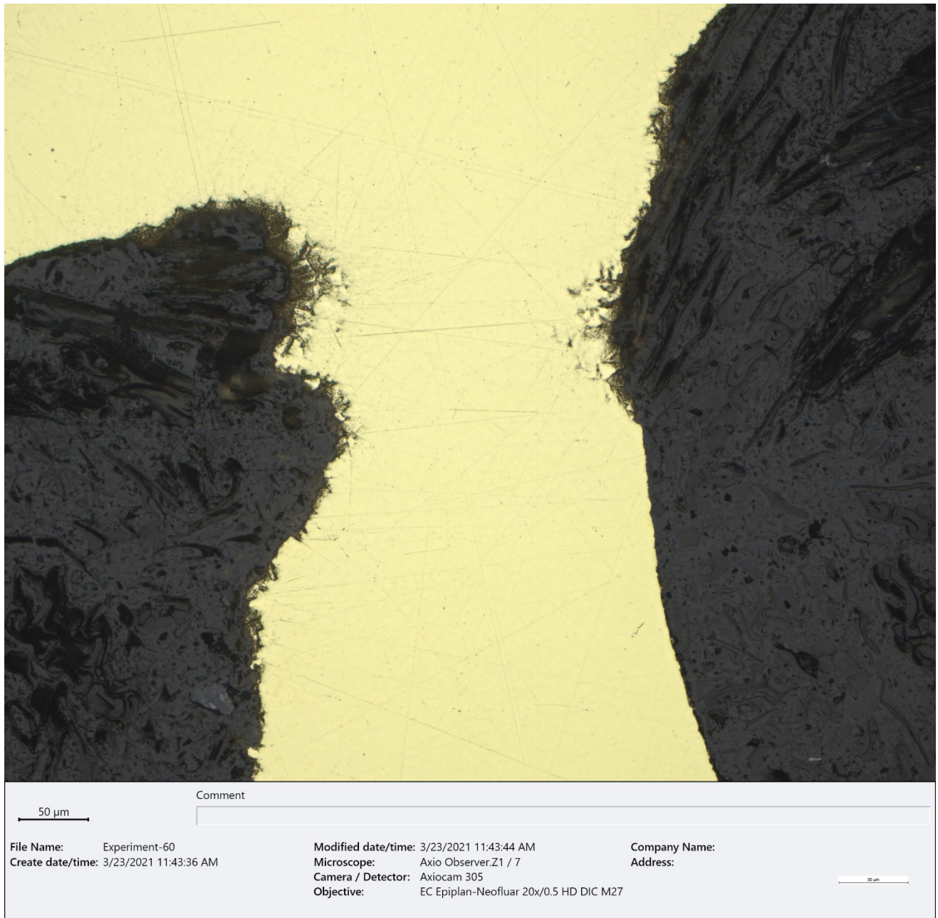
Figure 20 – Bright-field (BF) optical micrograph of an eroded area of a still intact web cross-section (~200X, as-polished).
