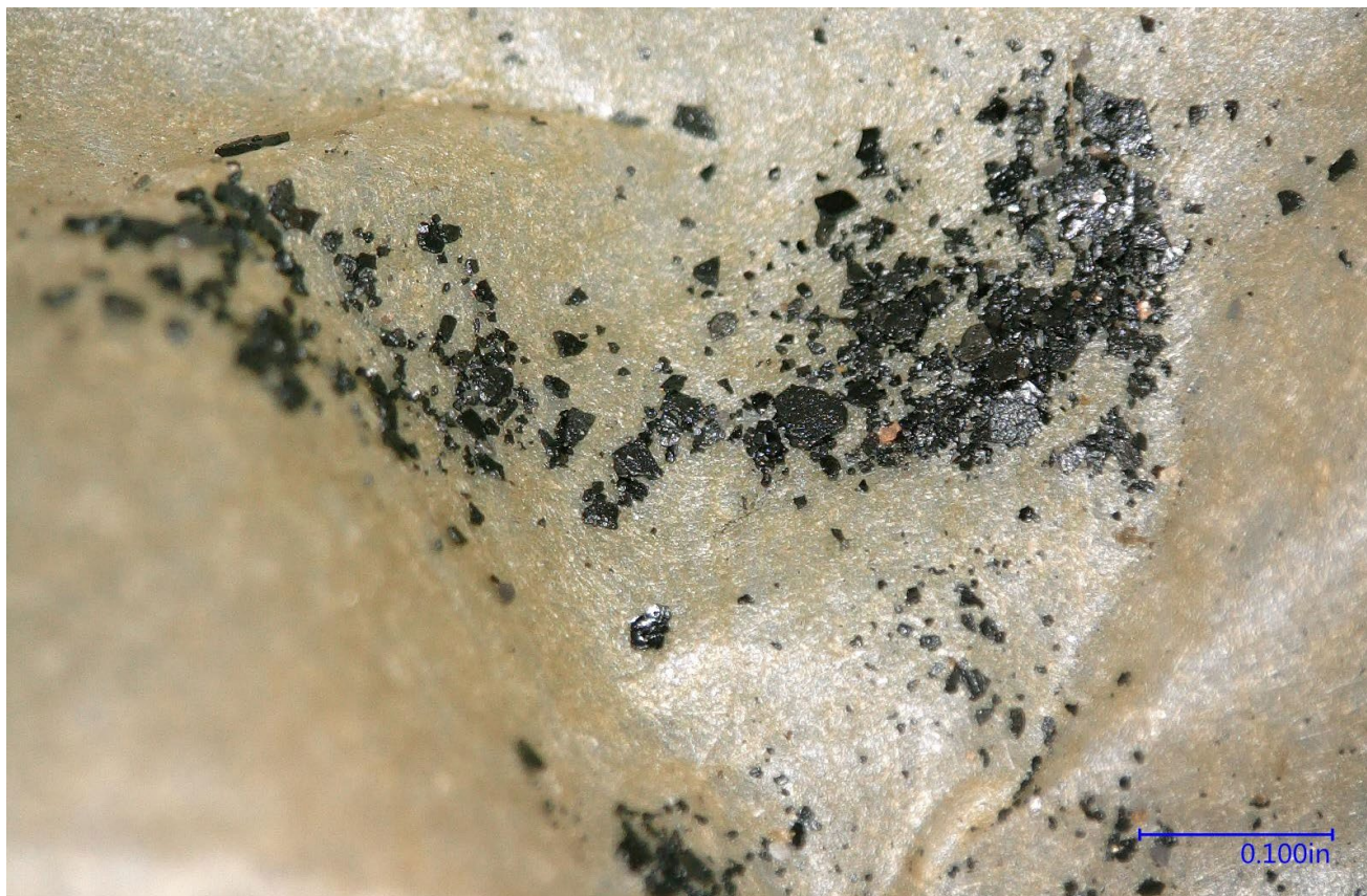
Figure 3 – View of the debris sent in a filter, showing most of the dark-colors particles.
