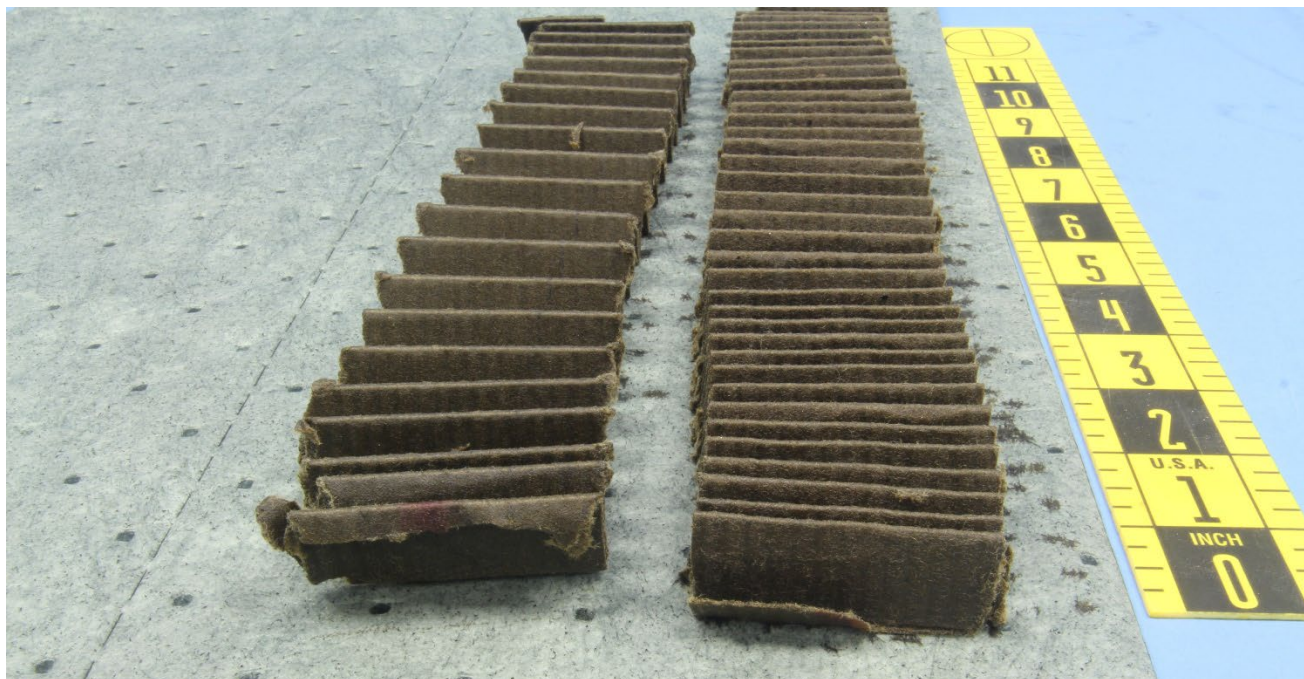
Figure 2 – View of two of the fractured ends of the filter.
