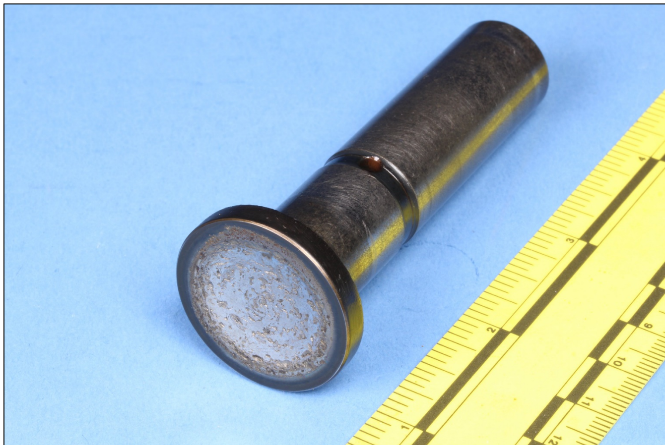
Figure 3. Head face on the number 1 exhaust tappet body.
