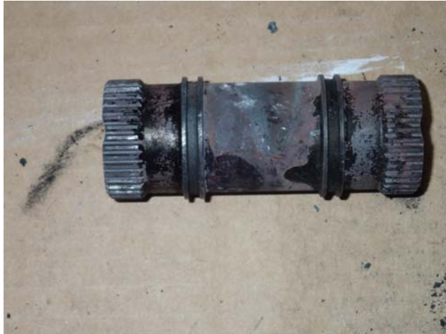
Power Turbine to Pinion Gear Coupling
