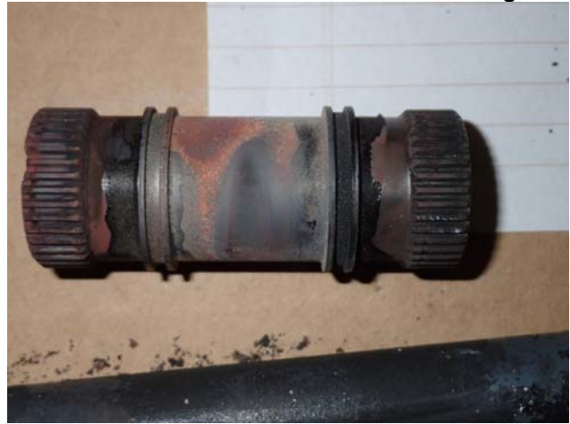
Power Turbine to Pinion Gear Coupling
