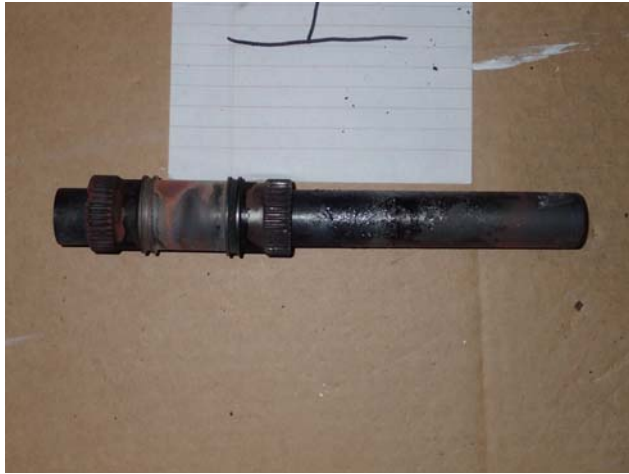
Power Turbine to Pinion Gear Coupling with Turbine to Compressor Coupling
