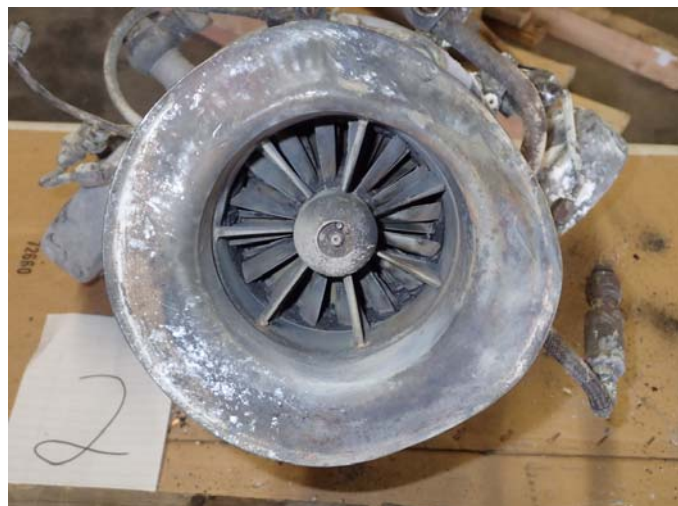
Compressor Inlet (Return)
