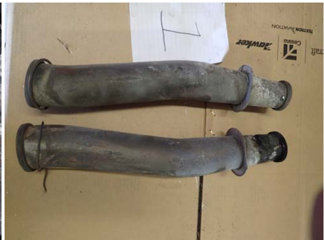
Compressor Air Discharge Tubes
