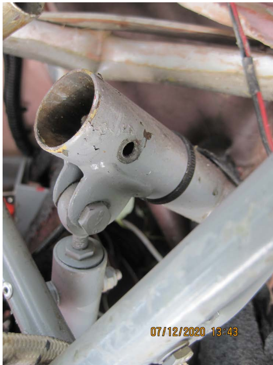
Photo 8 – Missing control stick socket (FAA photo)
