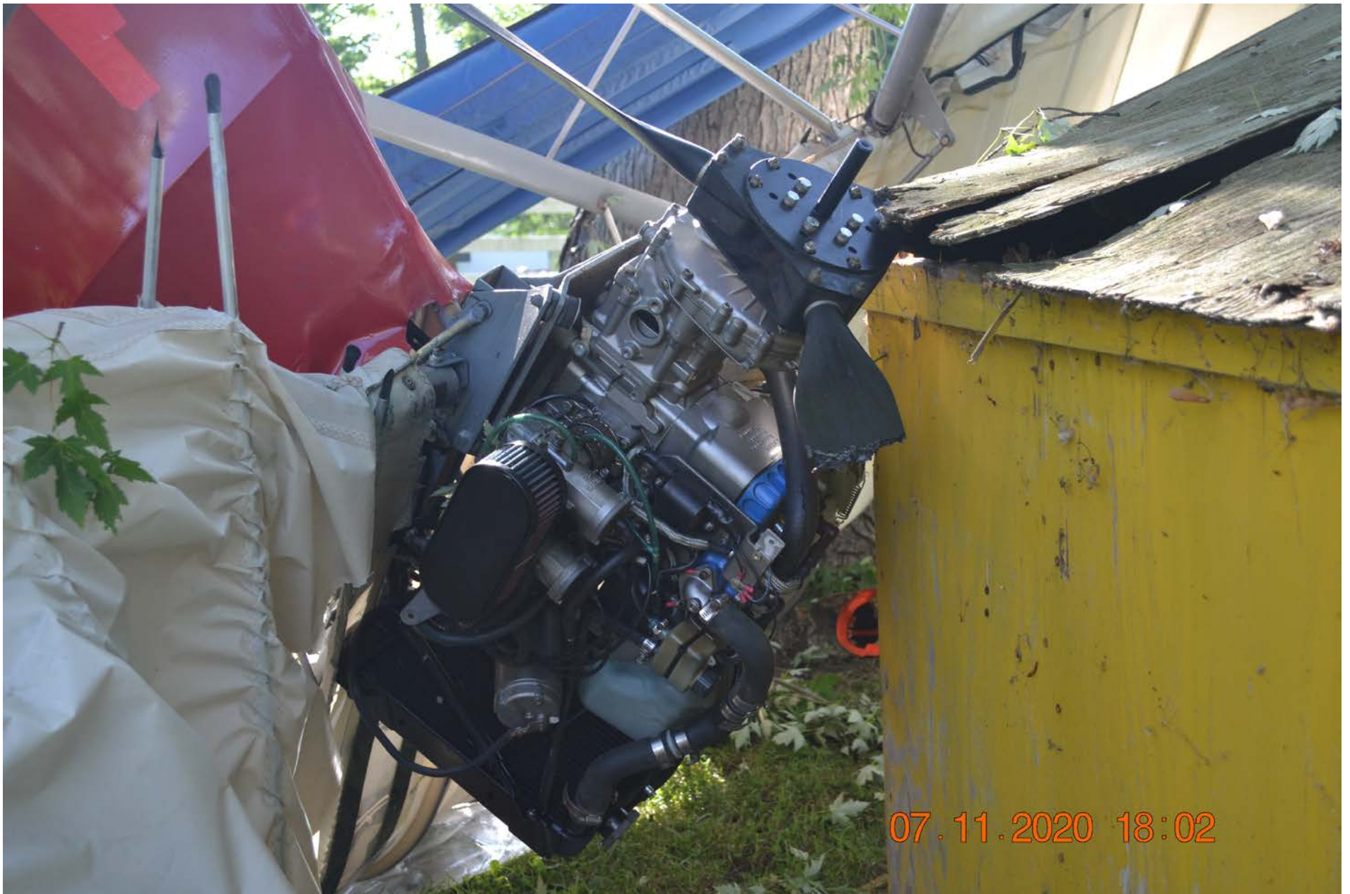
Photo 12 – The Rotax engine. Note severed propeller blade (FAA photo)
