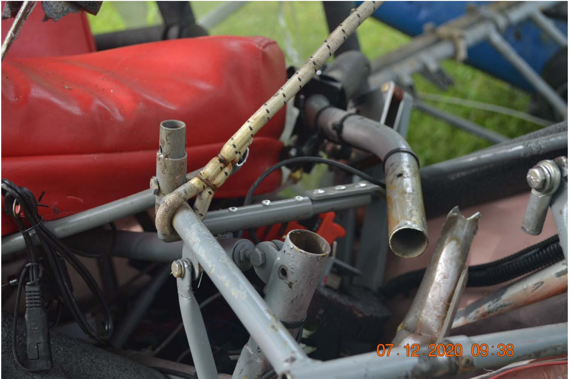
Photo 7 – Missing control stick (FAA photo)
