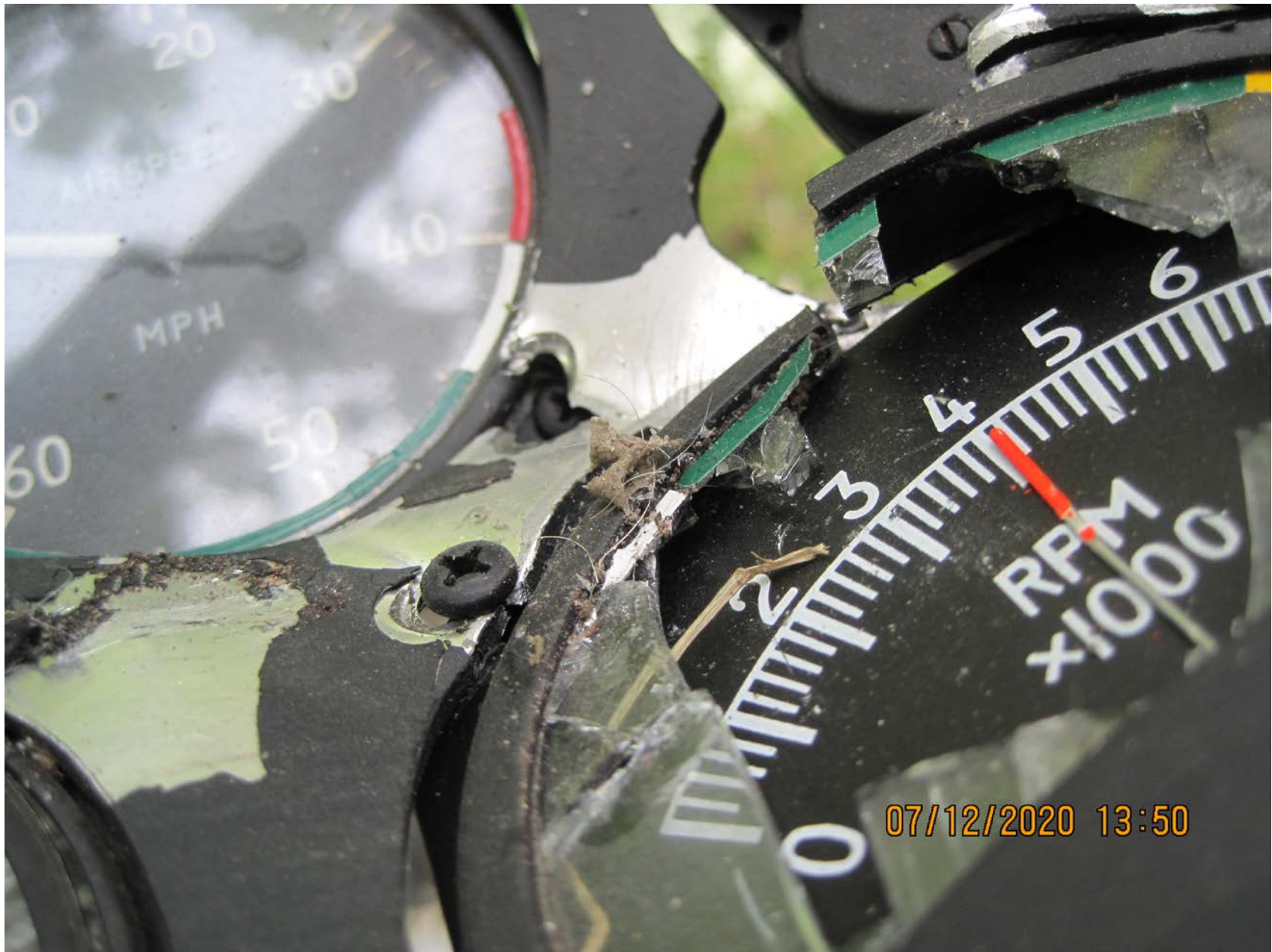
Photo 11 – The tachometer, indicating 4,000 rpm (FAA photo)
