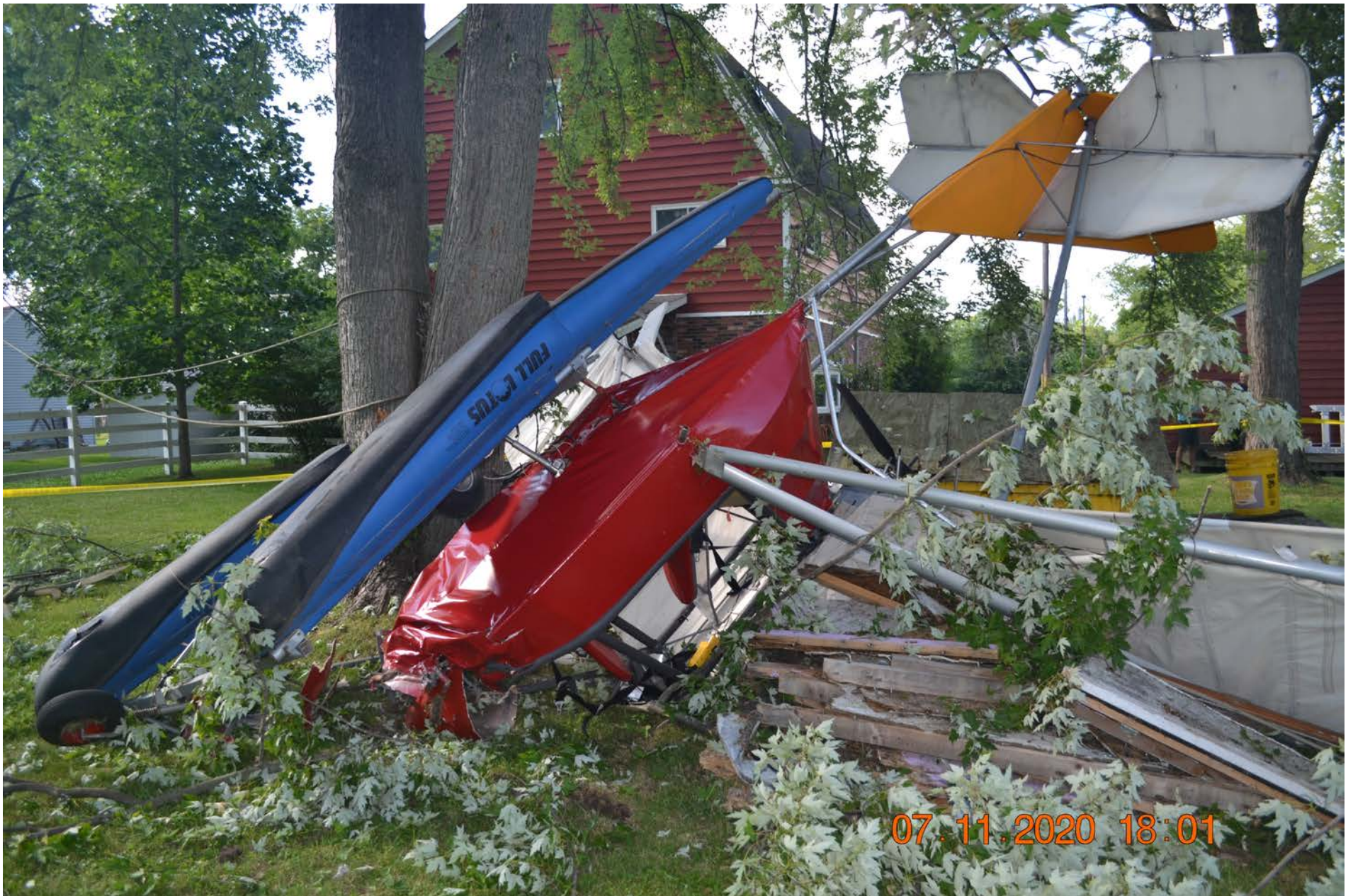
Photo 4 – Inverted N50JH. Note severed tree branches (FAA photo)
