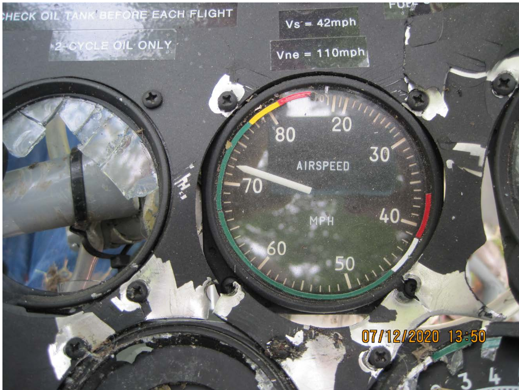
Photo 10 – The airspeed indicator, registering 72 mph (FAA photo)
