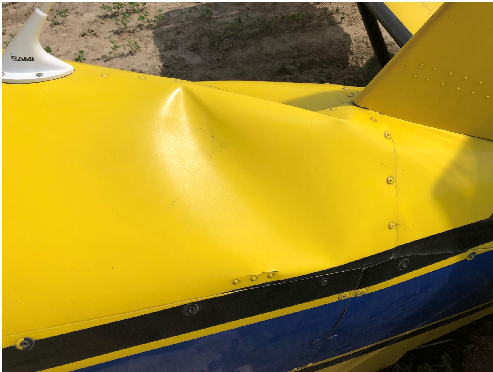
Photo 2 – Aft Fuselage Damage (FAA Photo)
