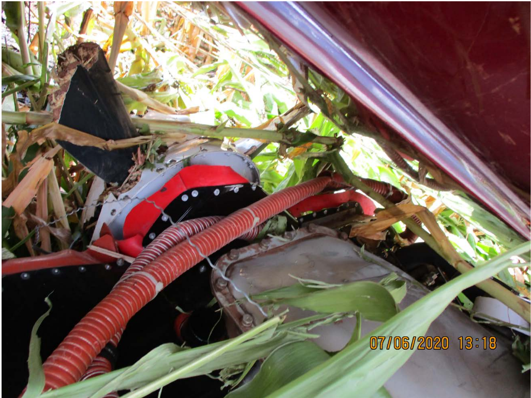
Photo 7 – Propeller hub and inverted engine (FAA photo)
