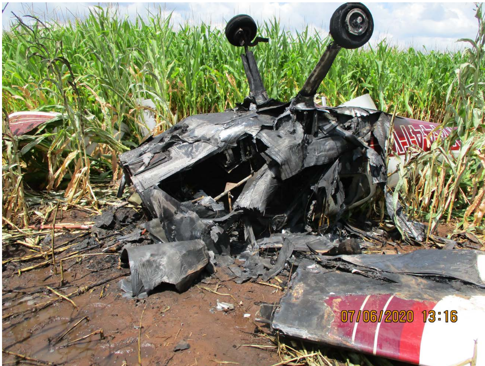
Photo 5 – Inverted cabin area totally consumed by fire (FAA photo)
