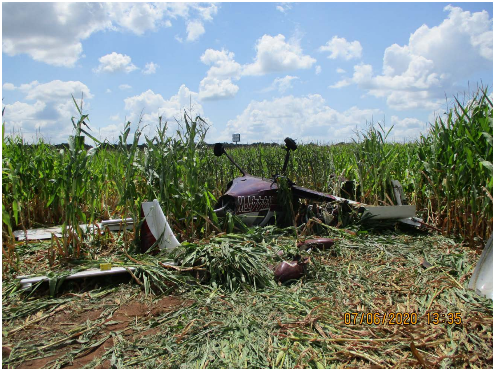
Photo 4 – The empennage (foreground) and cabin area (background) (FAA photo)
