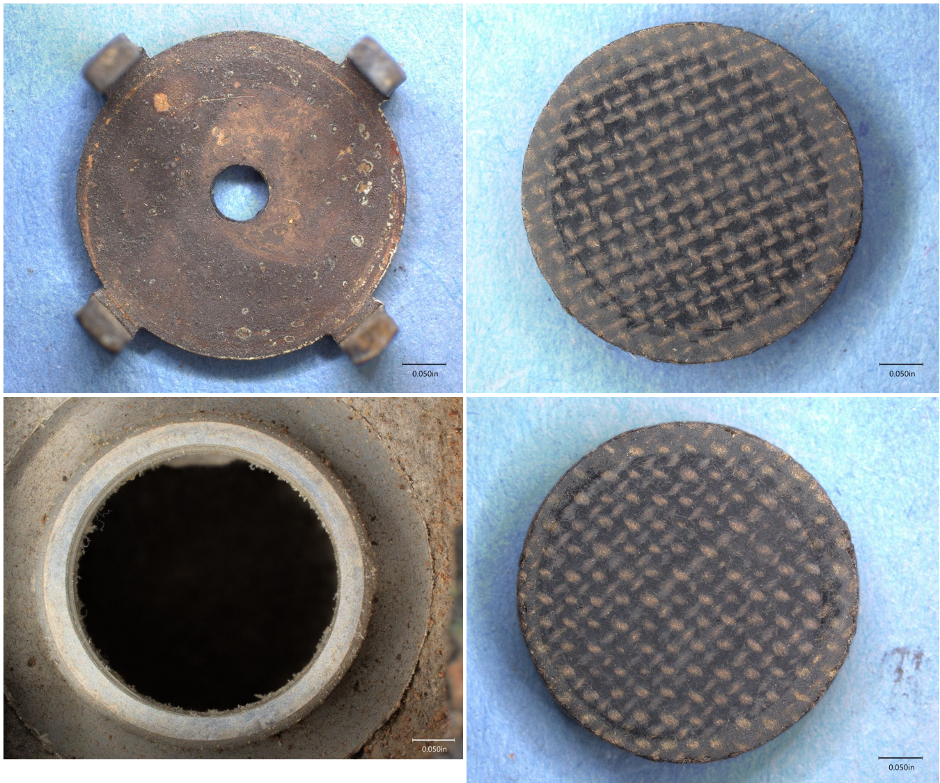
Figure 9: Digital microscope showing a view of the opposite side of the bypass valve guide as viewed in the previous figure after disassembly (upper left), the bypass valve port on the valve housing (lower left), and both sides of the bypass valve (upper and lower right). Circular off-center contact marks are evident around the outer edge of the bypass valve guide surface. Circular shaped rub marks were evident around the perimeter of the bypass valve on both sides as evidenced by a dull lighter appearance.
