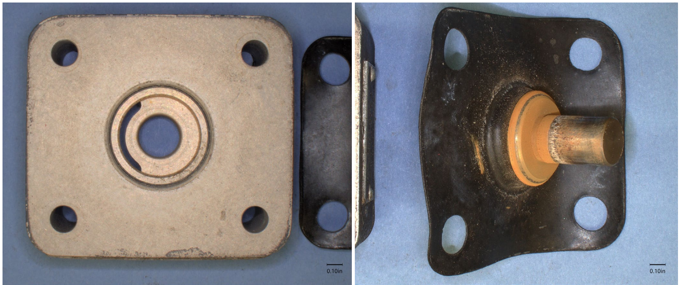
Figure 10: A digital microscope image showing a tilted view of the relief valve assembly (right) removed from the valve housing (left). A reddish orange powdery substance consistent with rust was observed covering the valve near the valve seat interface.
