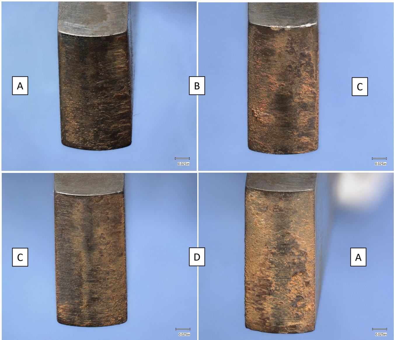
Figure 11: Digital microscope images of the fuel pump vane edges as removed from their relative rotor quadrant position (A-D). Material transfer and debris were observed consistent with adhesive and abrasive wear mechanisms.
