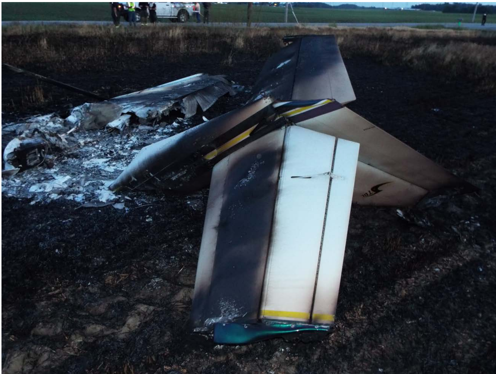
Photo 5 – Inverted empennage (FAA photo)
