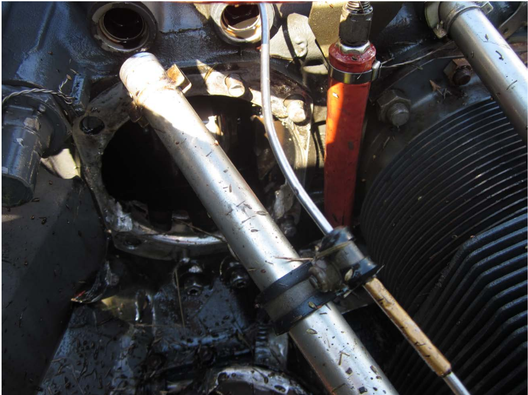
Photo 4 – Separated Engine Cylinder (FAA)
