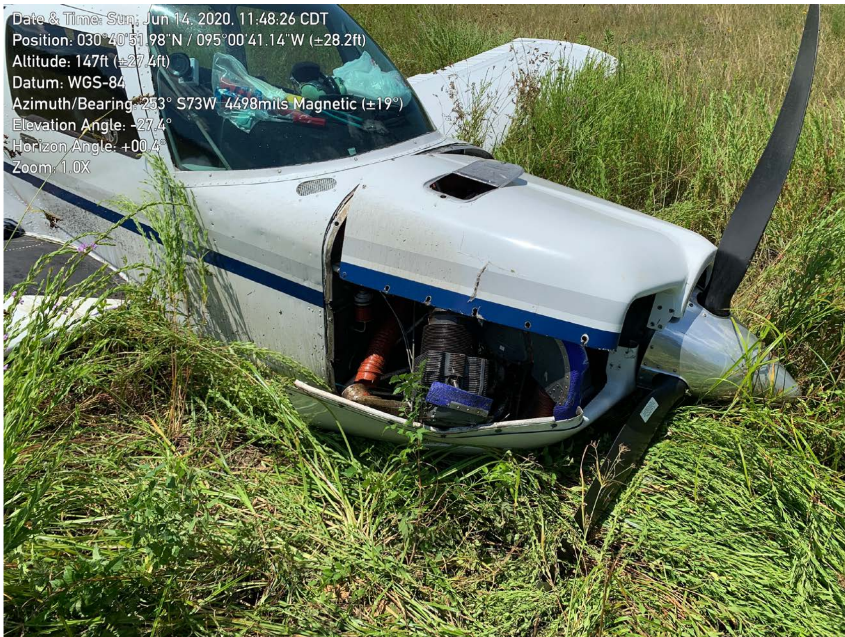
Photo 3 – Separated Engine Cylinder (FAA)
