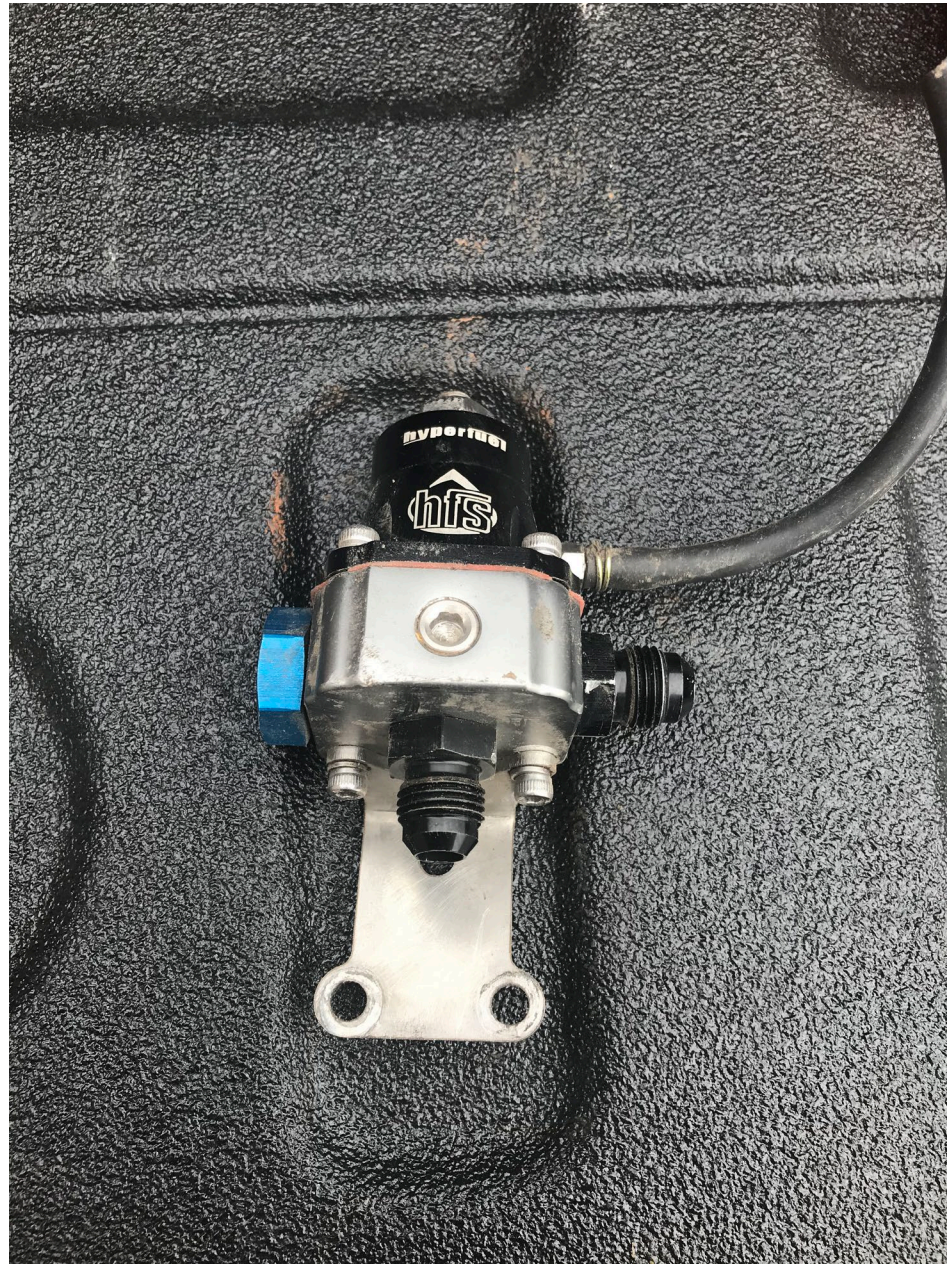
Photo 10 - Airplane fuel pressure regulator during postaccident examination (NTSB Photo)
