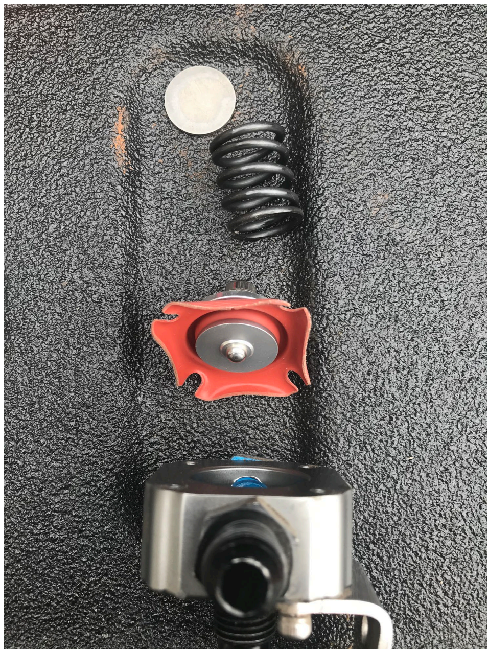
Photo 11 – Disassembled fuel pressure regulator (NTSB Photo)
