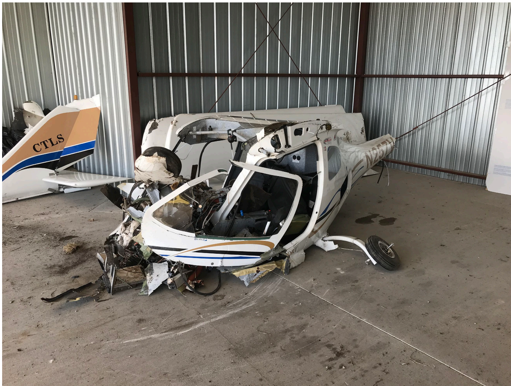
Photo 7 - Airplane fuselage during postaccident examination (NTSB Photo)
