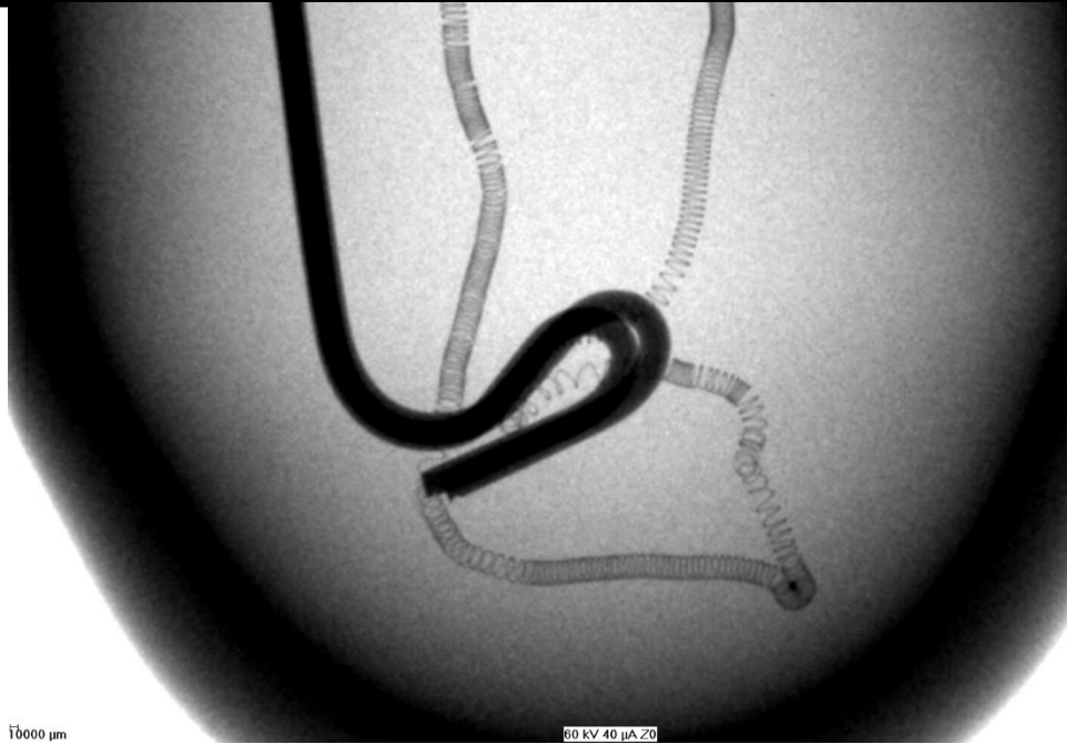
Figure 3. Radiograph of right bulb of Master Warning annunciator.
