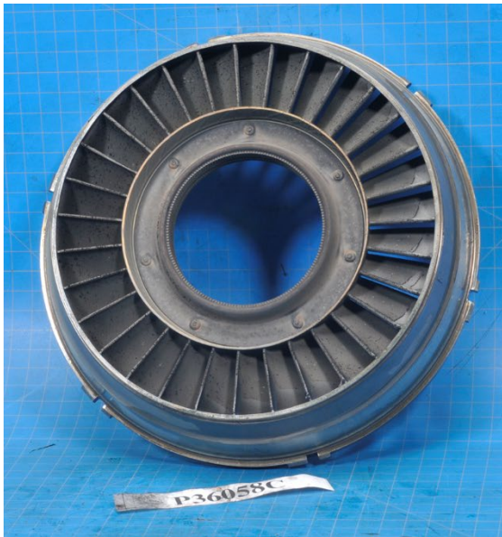
Photo 19- 3 rd Stage Turbine Stator, (L) Pressure Side, (R) Suction Side
