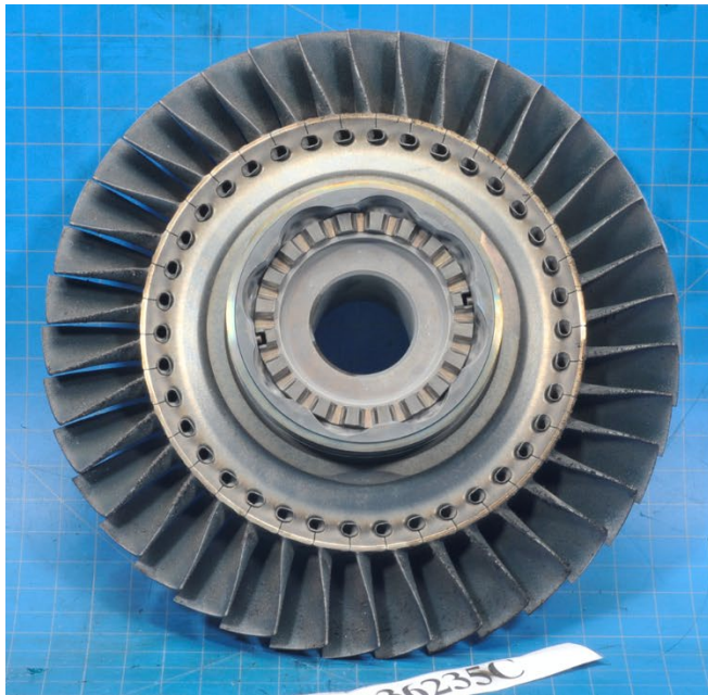
Photo 58-2 nd Stage Turbine Rotor, (L) Leading Edge, (R) Trailing Edge
