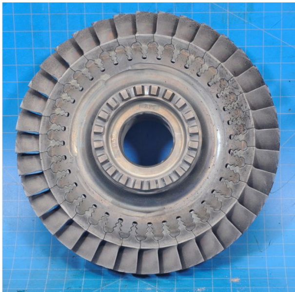
Photo 60- 1 st Stage Turbine Rotor, (L) Leading Edge, (R) Trailing Edge
