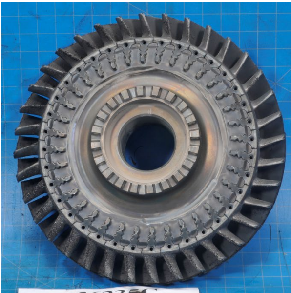
Photo 60- 1 st Stage Turbine Rotor, (L) Leading Edge, (R) Trailing Edge
