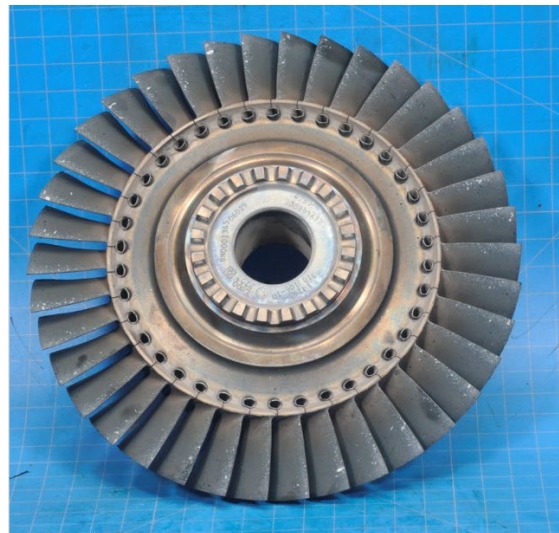
Photo 20- 2 nd Stage Turbine Rotor, (L) Leading Edge, (R) Trailing Edge
