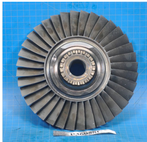
Photo 18- 3 rd Stage Turbine Rotor, (L) Leading Edge, (R) Trailing Edge
