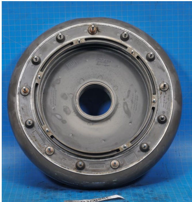
Photo 31- Compressor Crossover Duct Impact Damage/Hole
