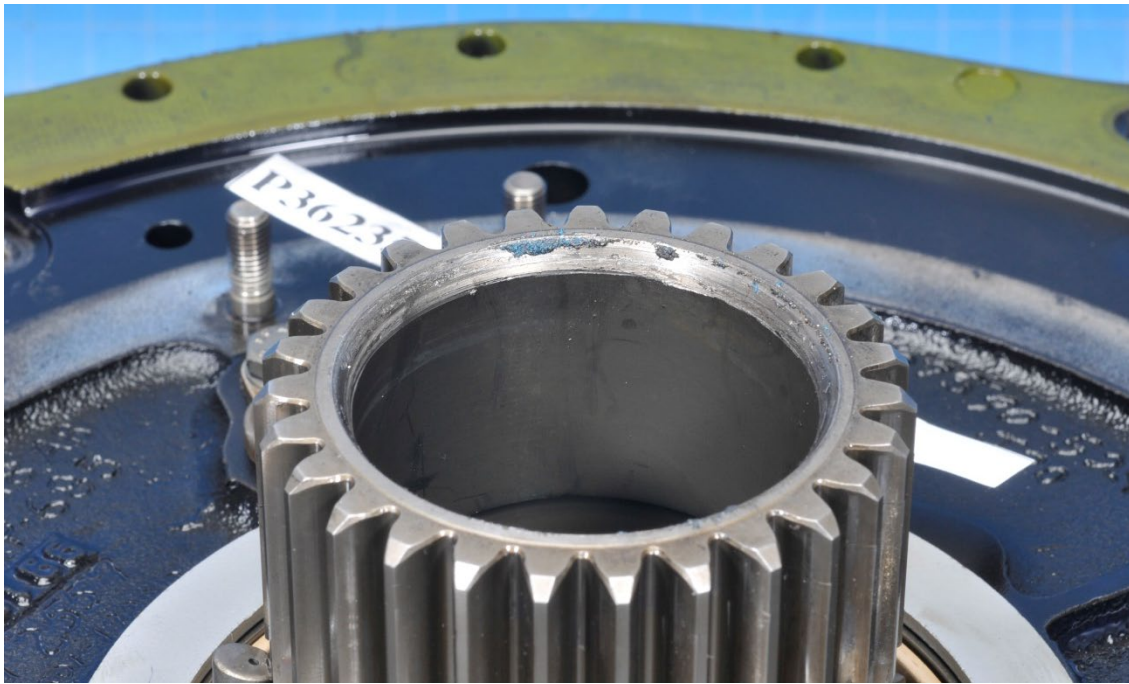
Photo 51- Sun Gear Forward Face Circumferential Scoring
