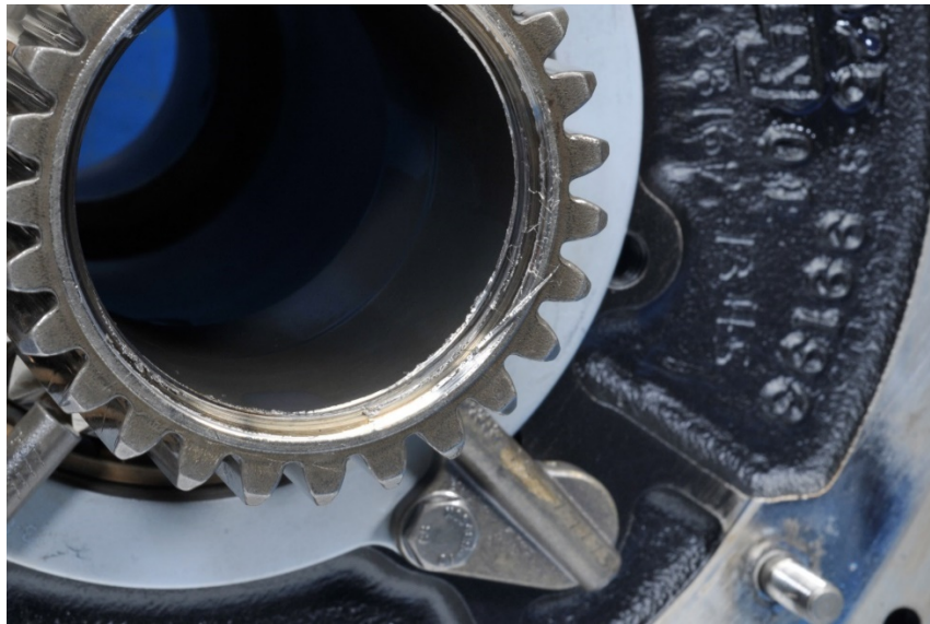
Photo 14- Sun Gear Inner Diameter Rub Damage
