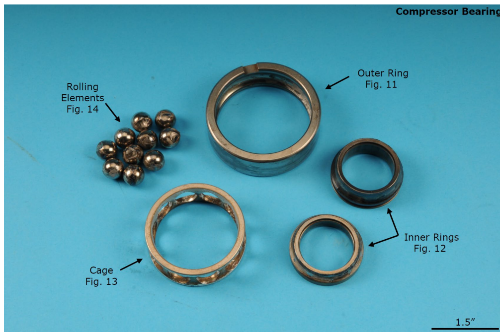
Photo 76- Disassembled No. 1 Bearing
