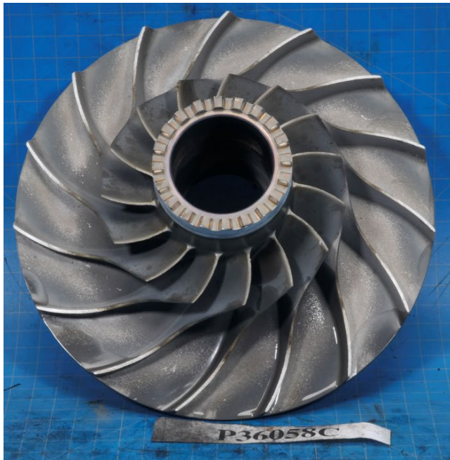
Photo 25- (L) 2 nd Stage Compressor Impeller Vane Scoring, (R) Impeller Curvic Coupling Outer Diameter Scoring
