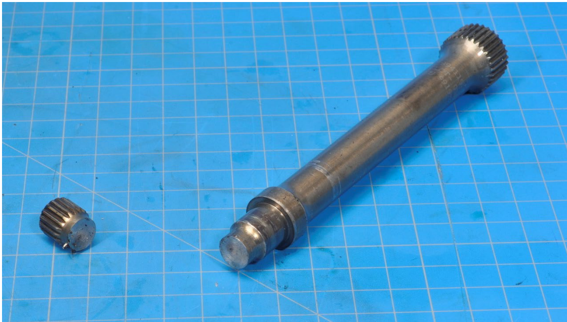
Photo 54- Separated Torque Coupling Shaft
