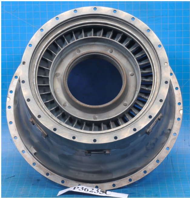
Photo 59- 2 nd Stage Turbine Stator, (L) Pressure Side, (R) Suction Side
