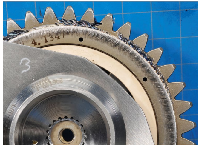
Photo 50- Planetary Gear Teeth, Aft Face Circumferential Scoring
