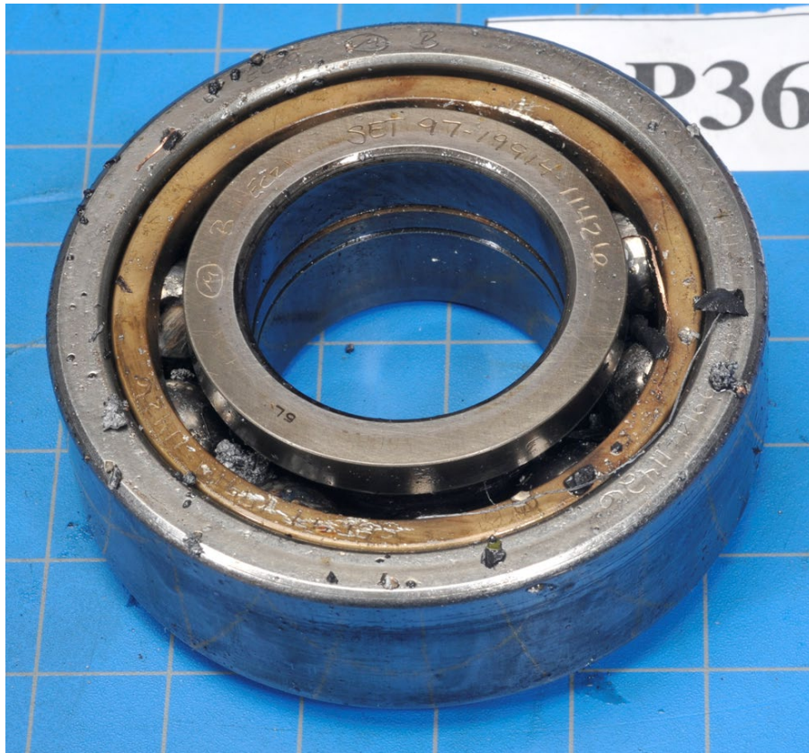
Photo 68- No. 1 (Compressor) Bearing
