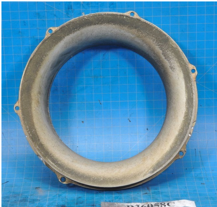
Photo 30- 1 st Stage Impeller Shroud Circumferential Scoring
