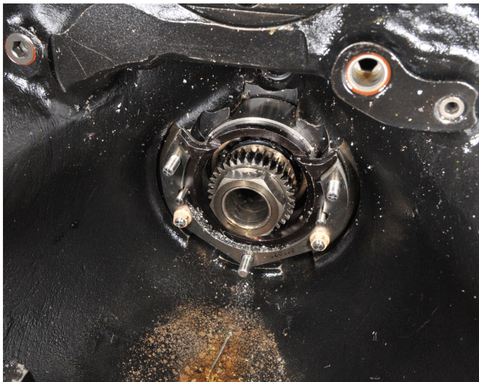
Photo 55- Main Shaft and AGB Debris Accumulation
