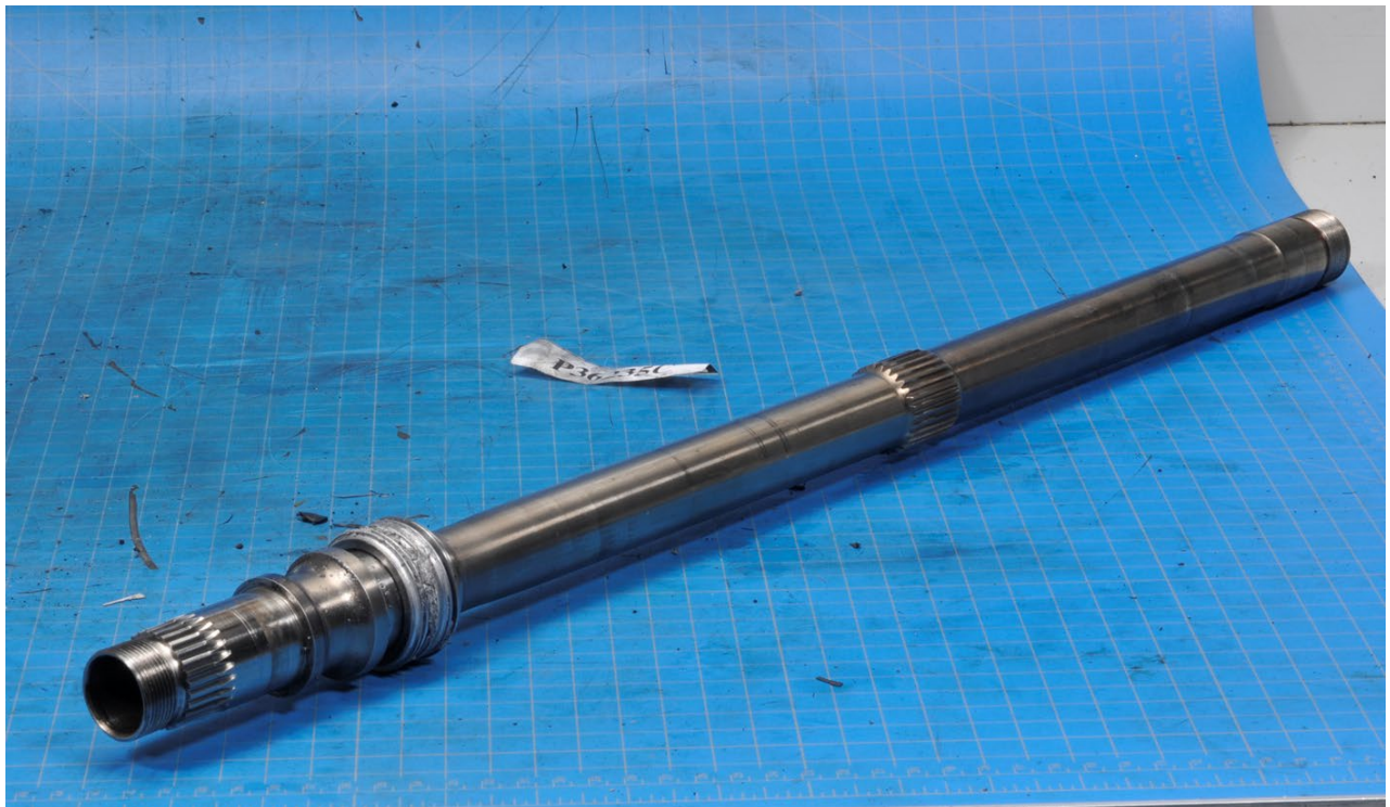
Photo 69- Main Shaft Knife Edge Seal Damage
