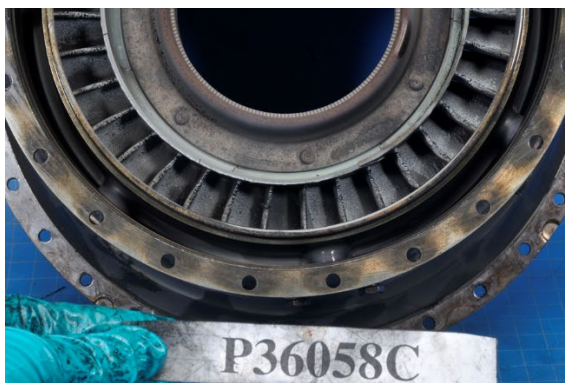
Photo 21- 2 nd Stage Turbine Stator, (L) Pressure Side, (R) Suction Side
