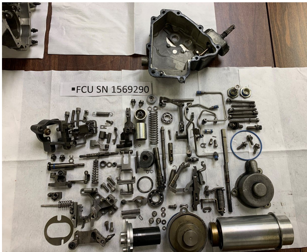
Photo 33- No. 1 Engine FCU Disassembled
