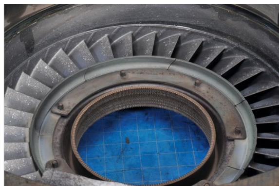
Photo 21- 2 nd Stage Turbine Stator, (L) Pressure Side, (R) Suction Side
