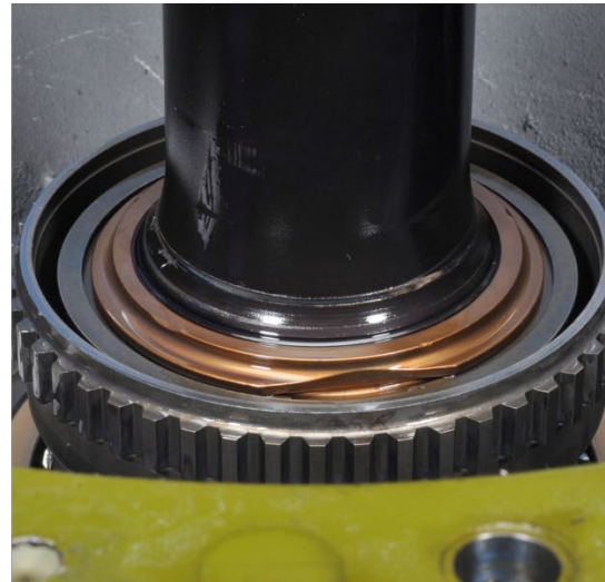
Photo 11- (L) Nose Cone Following Removal, (R) Propeller Shaft Circumferential Rub at Lower Radius
