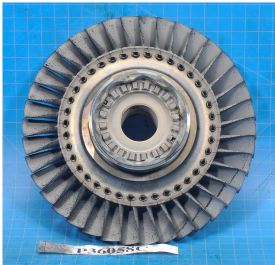
Photo 20- 2 nd Stage Turbine Rotor, (L) Leading Edge, (R) Trailing Edge
