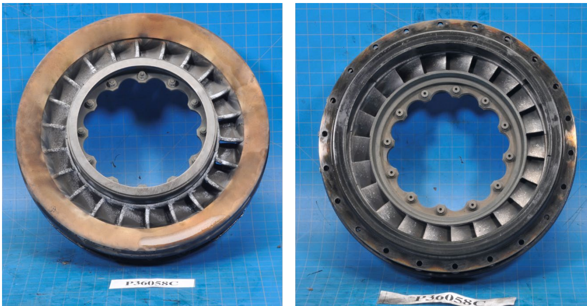
Photo 23- 1 st Stage Turbine Stator, (L) Pressure Side, (R) Suction Side
