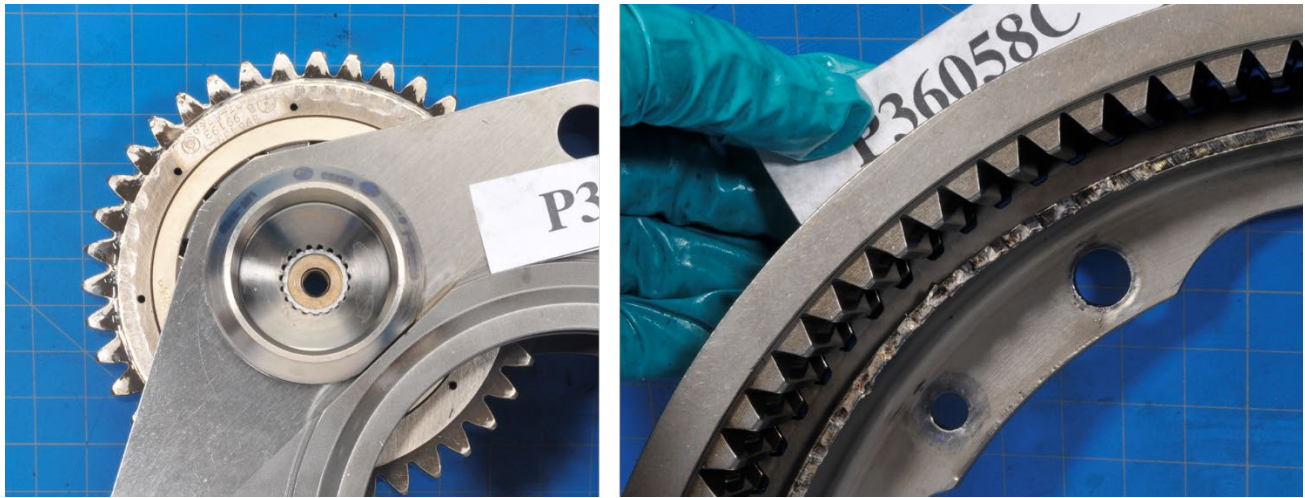
Photo 13- (L) Damage on Planetary Gear Teeth Aft Face, (R) Rub/Impact Damage on the Ring Gear Support
