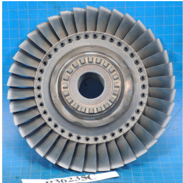
Photo 58-2 nd Stage Turbine Rotor, (L) Leading Edge, (R) Trailing Edge
