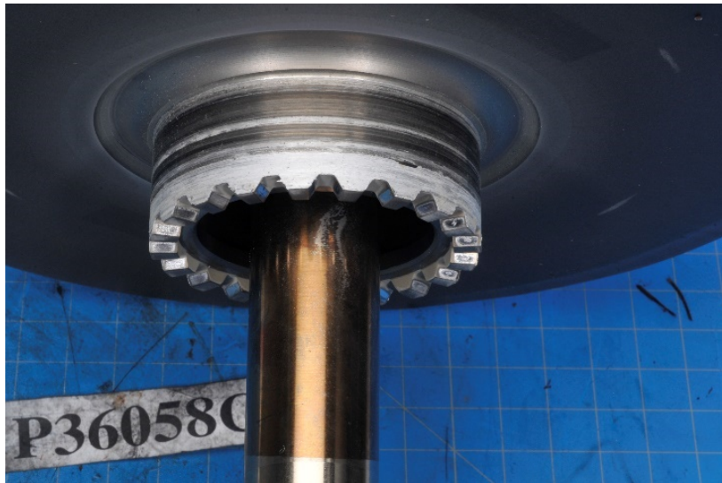
Photo 29- 1 st Stage Compressor Impeller Curvic Coupling Outer Diameter Scoring
