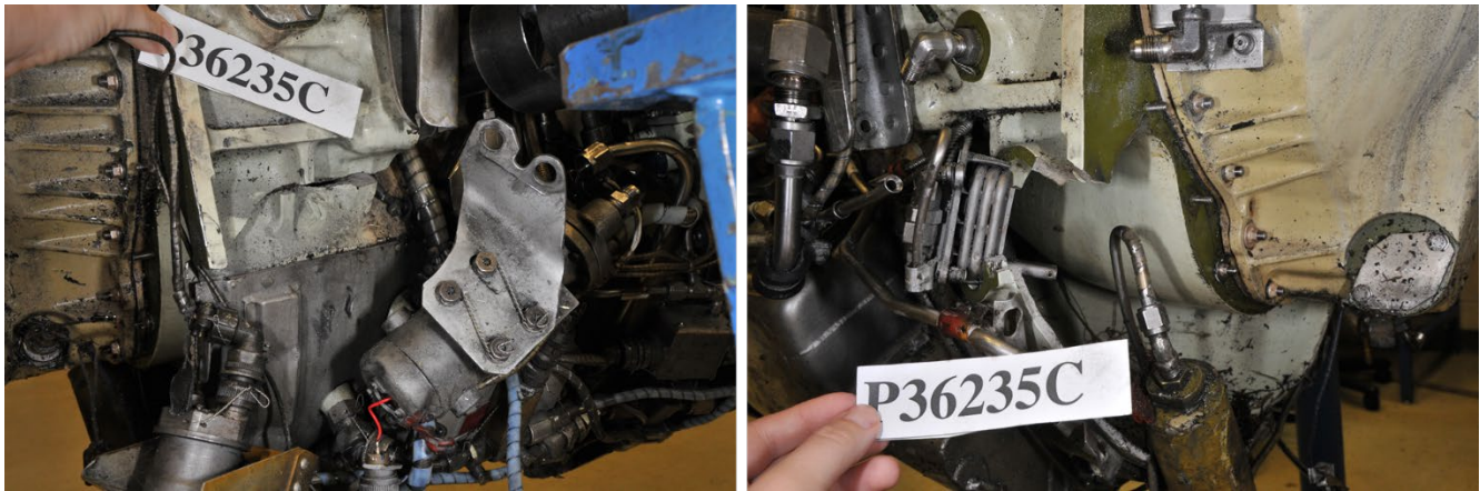
Photo 42- AGB Case Fracture, (L) Left Side, (R) Right Side
