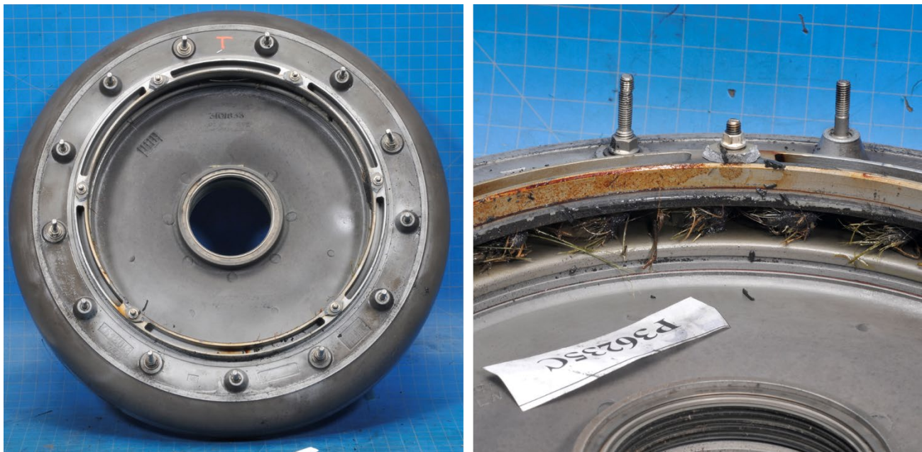
Photo 67- (L) Compressor Crossover Duct, (R) 1 st Stage Diffuser with Debris Accumulation
