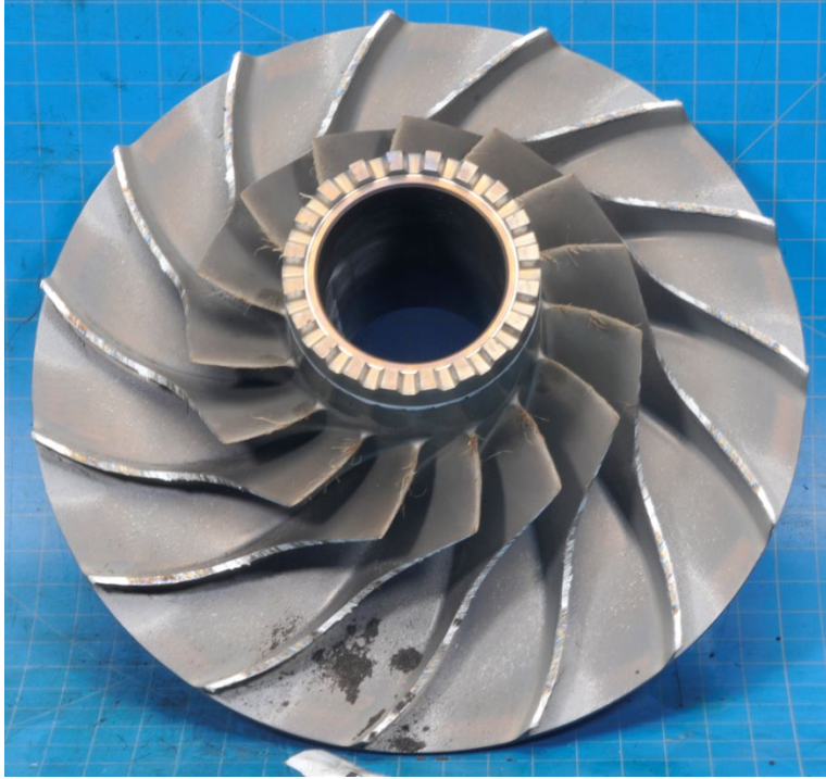
Photo 63- 2 nd Stage Compressor Impeller Tip Rub
