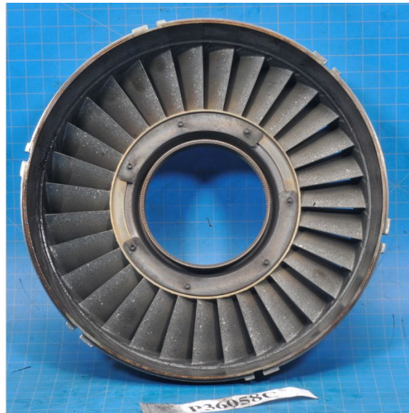
Photo 19- 3 rd Stage Turbine Stator, (L) Pressure Side, (R) Suction Side
