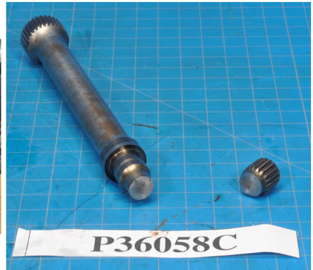
Photo 15- Separated Torque Coupling Shaft
