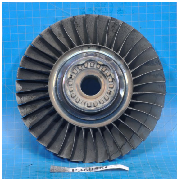
Photo 18- 3 rd Stage Turbine Rotor, (L) Leading Edge, (R) Trailing Edge
