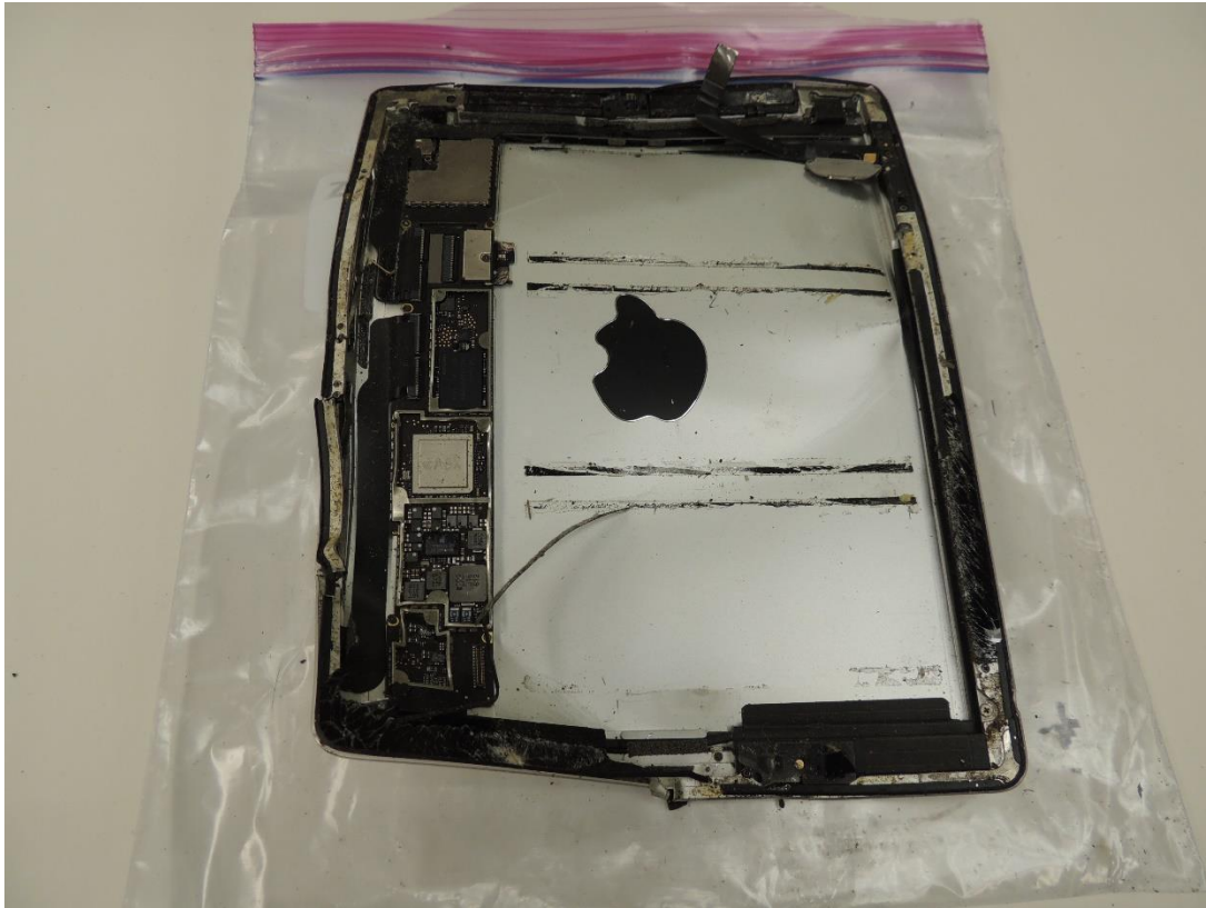
Figure 2. The iPad A1459 (4 th Generation), as received.
