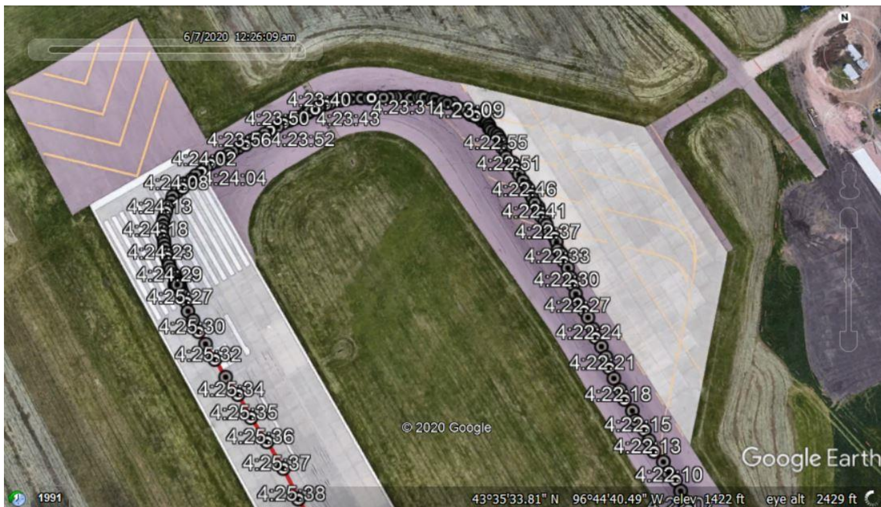
Figure 6. A Google Earth plot showing the accident aircraft's ground track in the vicinity of the run-up apron and subsequent departure.
