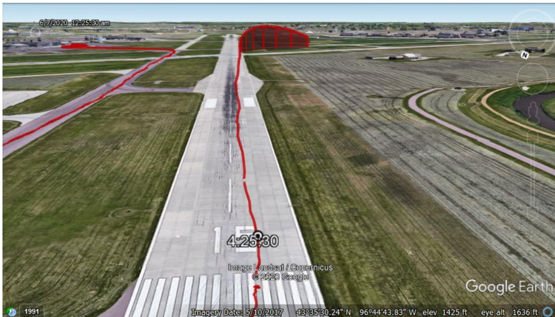
Figure 7. A Google Earth plot showing the accident aircraft's ground track and recorded altitude data in relation to the runway's centerline.
