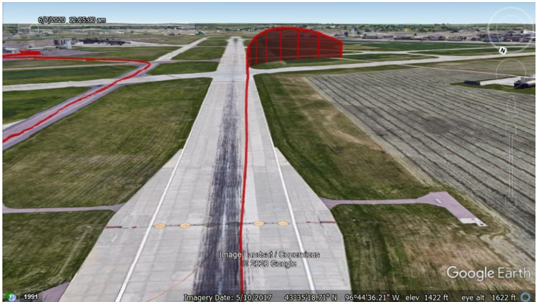
Figure 8. A Google Earth plot showing the accident aircraft's ground track and recorded altitude data in relation to the runway's centerline. There is a noticeably right ground track that begins about 1500 feet from the departure runway's threshold.
