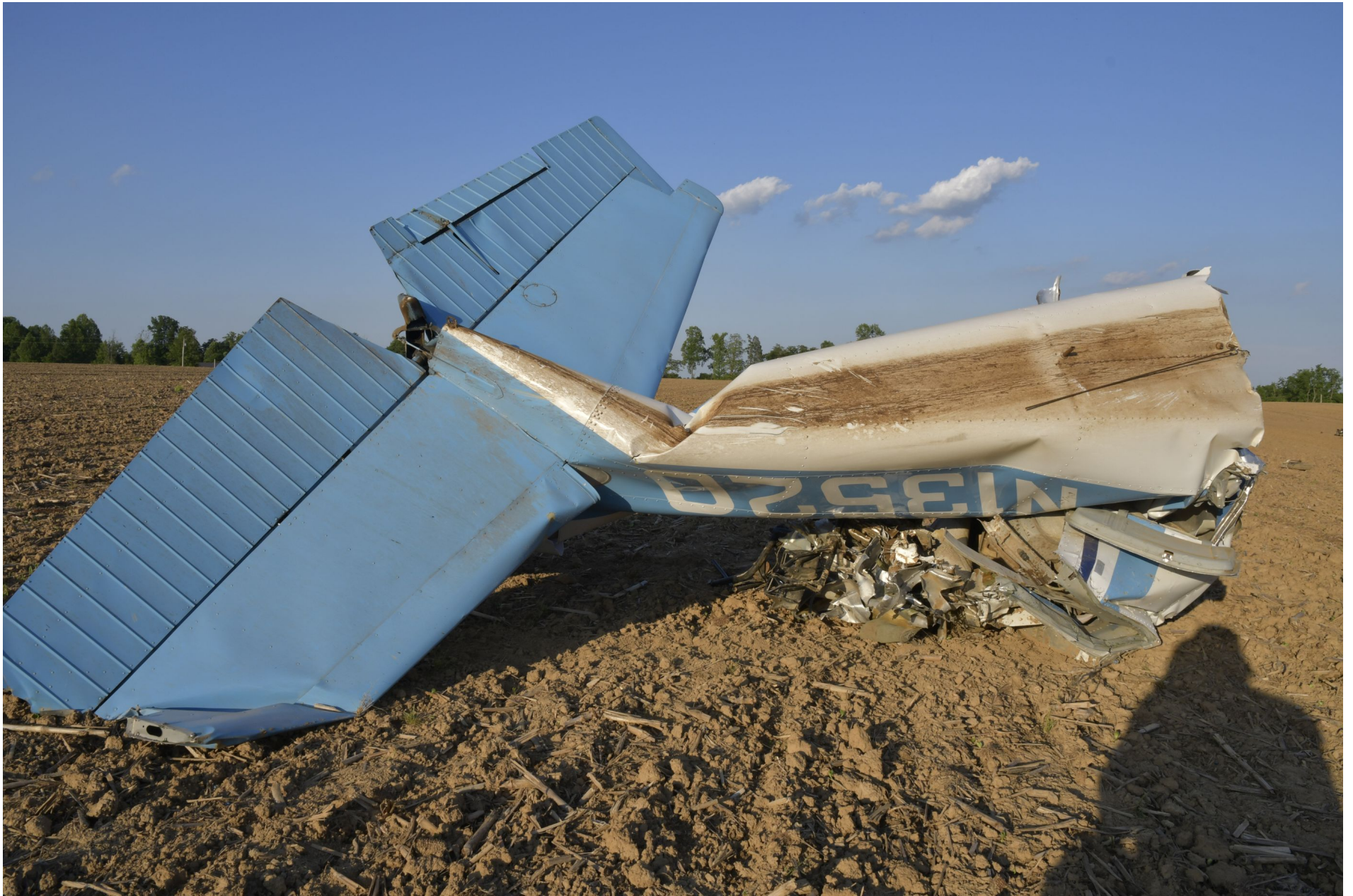
Photo 9 – Empennage (Courtesy of ISP)
