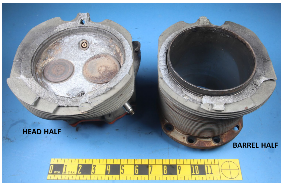
Figure 1: Macro photo of the two halves of the separated no. 1 cylinder.
