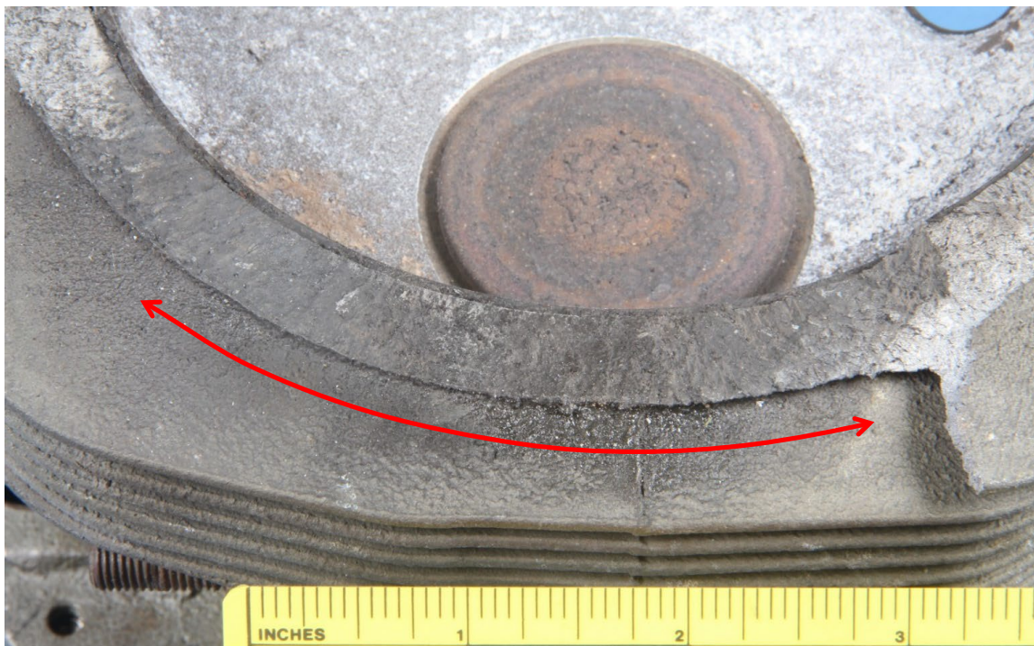
Figure 4: (Top) Macro photo of the fracture surface on the head half of the separated cylinder. (Bottom) Close-up photo of the fracture surface on the exhaust side in the location indicated by the yellow arrow in the top photo. The red double-sided arrow indicates a through-wall crack on the fracture surface.
