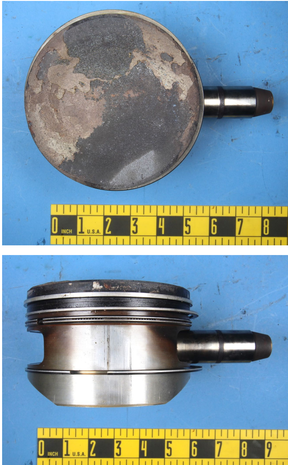
Figure 7: Macro photos of the no. 1 piston head and mating piston pin as viewed from the top and side (top and bottom images, respectively).
