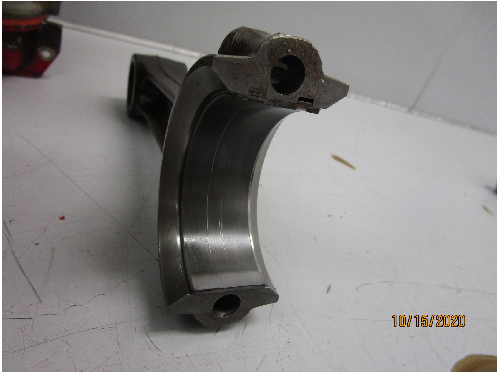
Photo 13 - Close-up view of the connecting rod bearing. The bearing surface exhibits witness marks consistent with hard particle passage.
