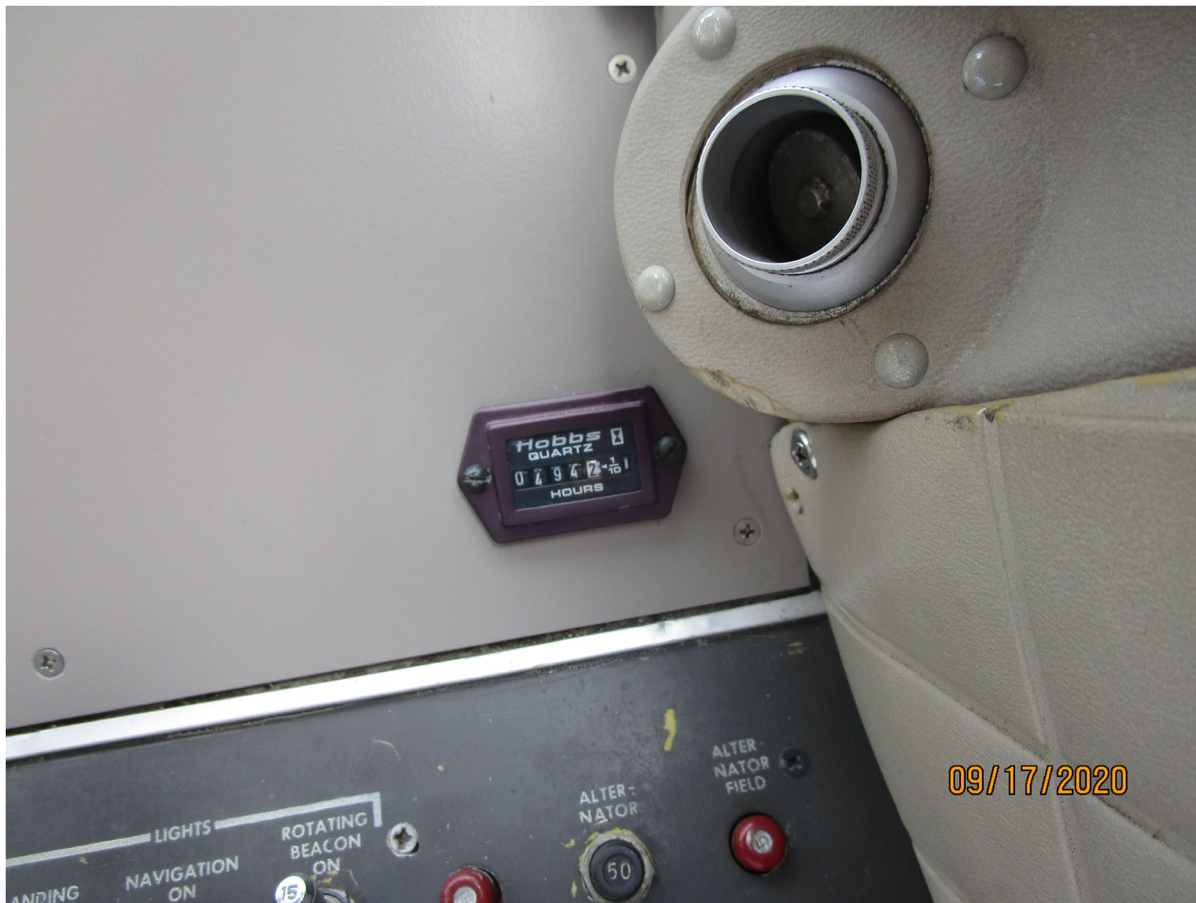
Photo 4 - View of the Hobbs meter. The meter indicates 494.2 hours.
