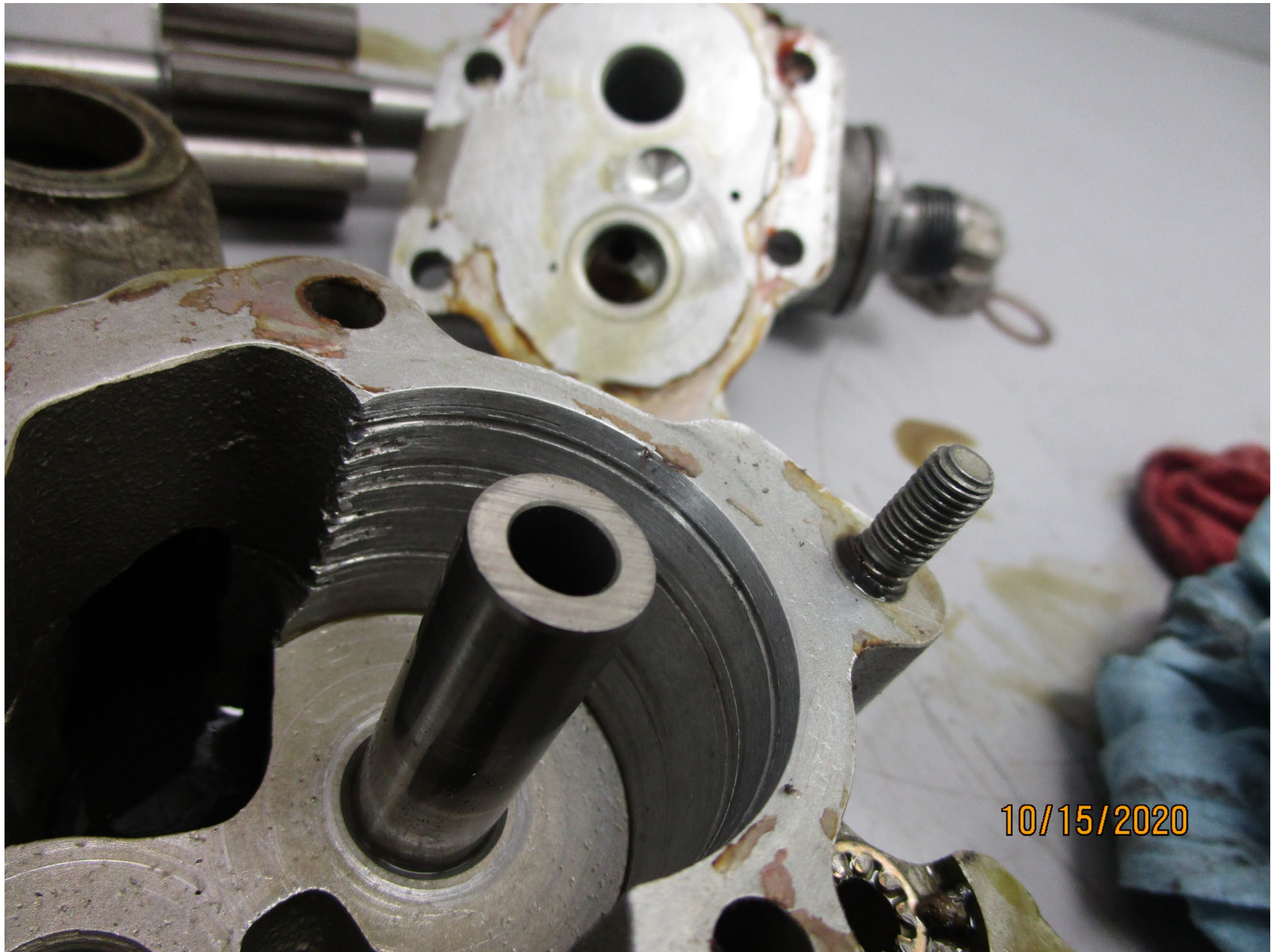
Photo 10 - Close-up view of inside surfaces of the oil pump. The surfaces exhibit witness marks consistent with hard particle passage.
