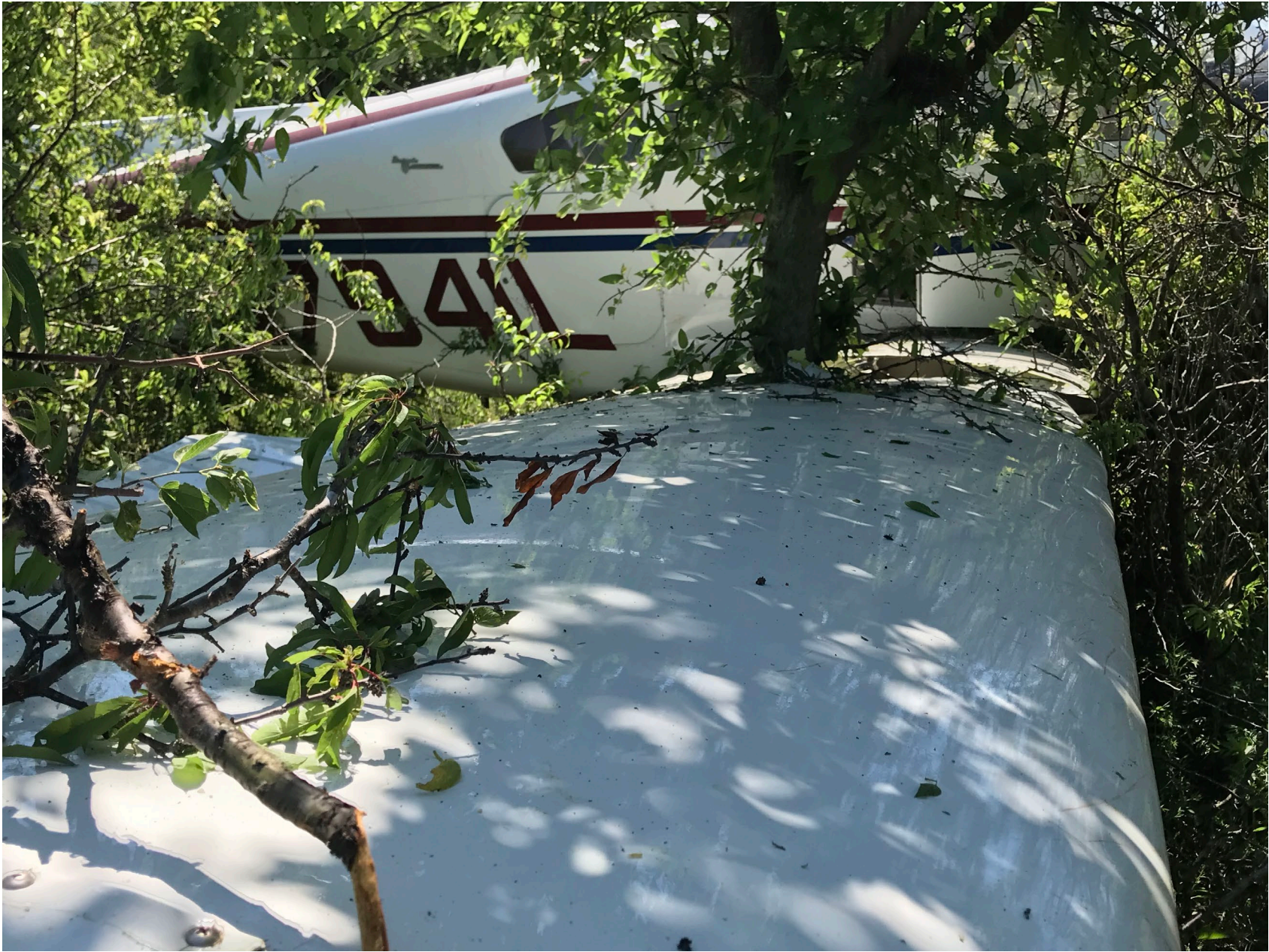
Photo 3 - FAA supplied view of the right wing. The leading edge of the wing about midspan is deformed around a tree trunk.
