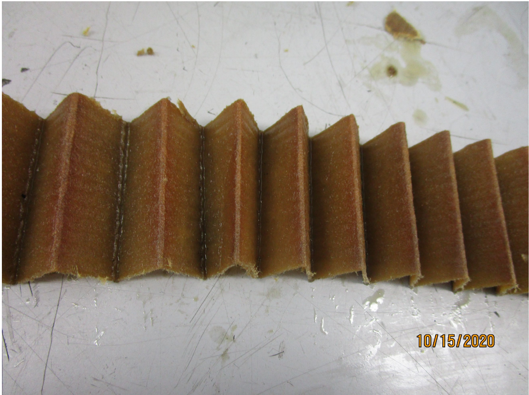
Photo 12 - Close-up view of the filter in the oil filter.
