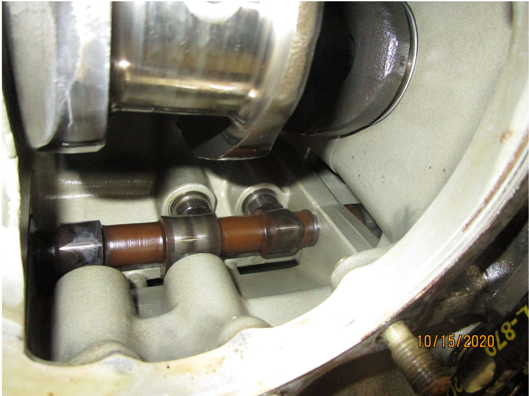
Photo 14 - Close-up view through the removed cylinder of the crankshaft and camshaft inside the crankcase.
