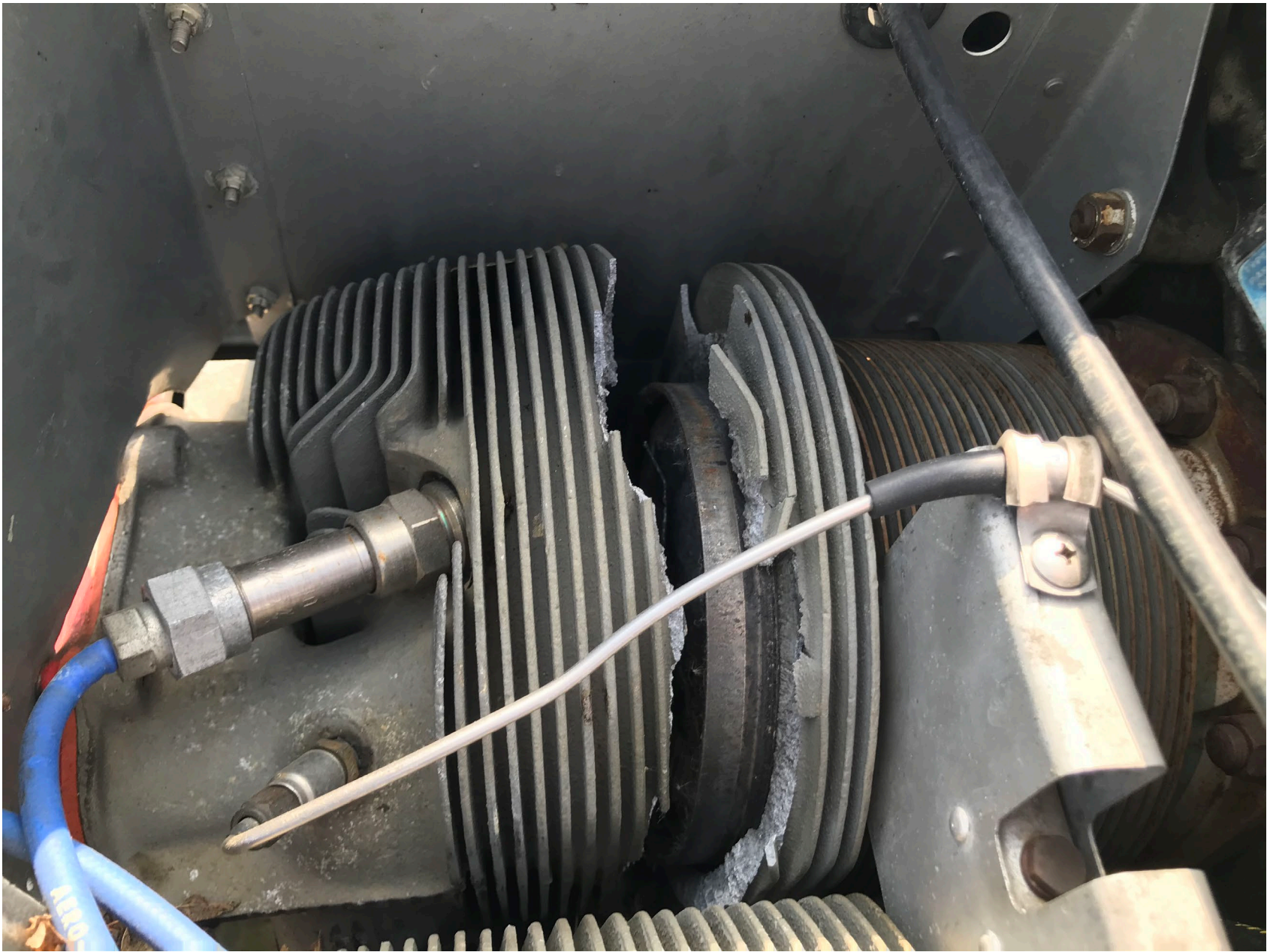
Photo 6 - Close-up view of the separated cylinder.
