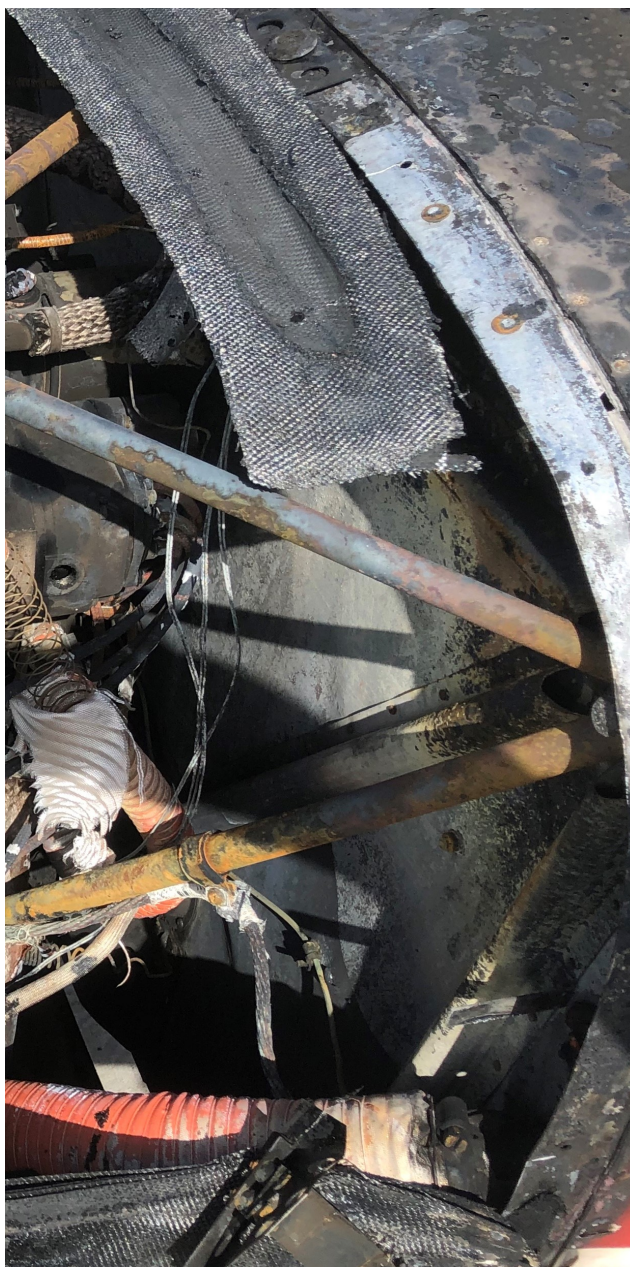
Photo 2 –Severe Heat Damage to Engine in Area of Left Side Firewall (Courtesy of FAA)
