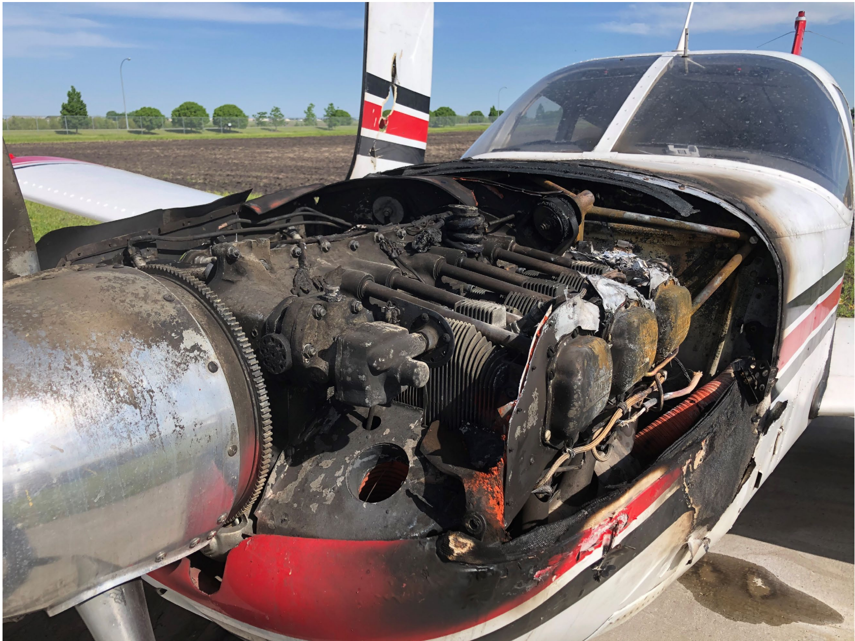
Photo 1 – Fire Damage to Left Side of Engine (Courtesy of FAA)
