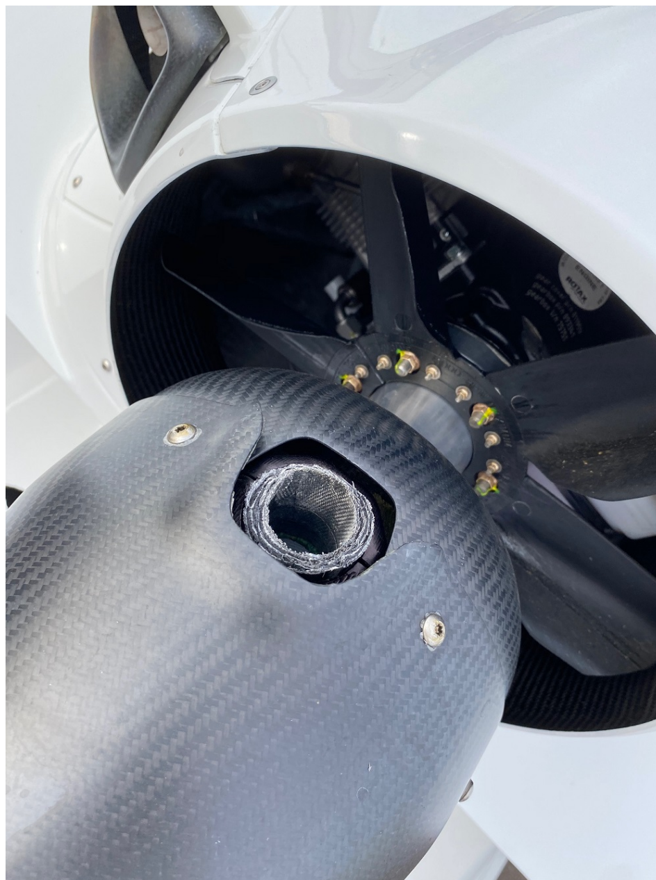
Photo 2 – Missing propeller blade
