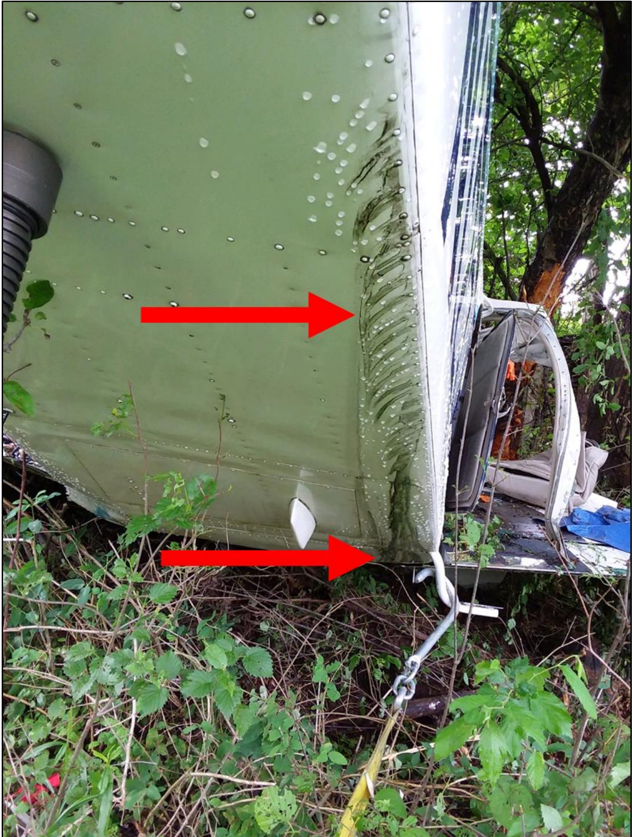
Figure 6 - Fuel Streaks on Lower Right Side of Fuselage (FAA Photo)
