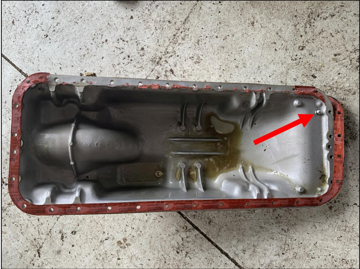
Figure 16 - Engine Oil Sump Pan Containing Portion of Quick-Drain Plug
