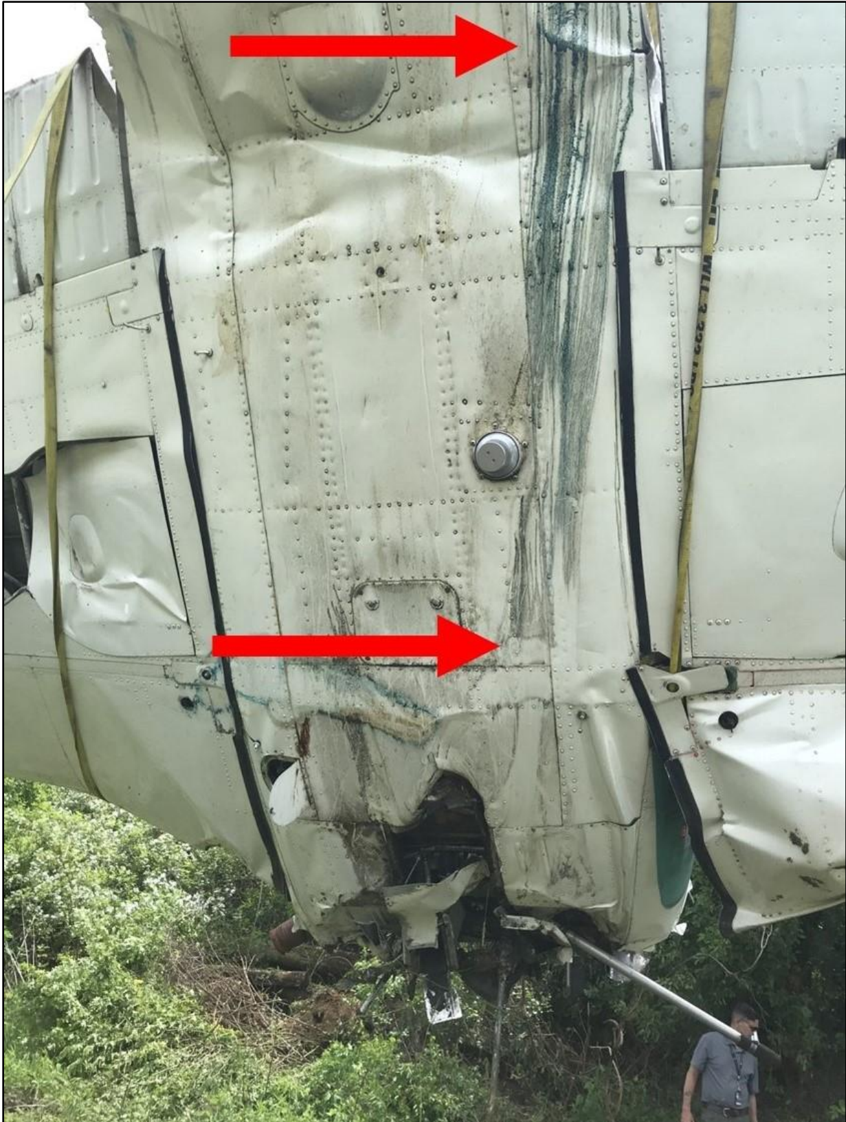
Figure 7 - Fuel Streaks on Lower Right Side of Fuselage (AMF Aviation Photo)
