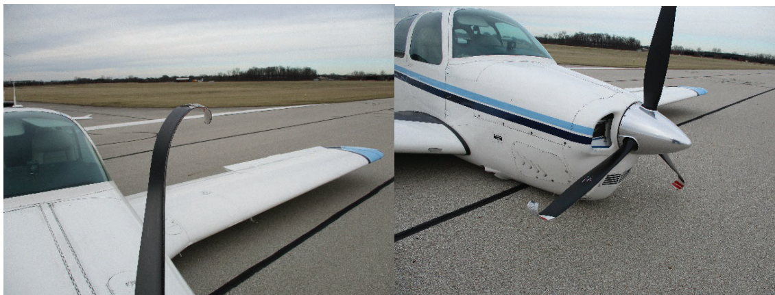
This is the condition of the props on N123JB after the 02/04/2020 incident.
