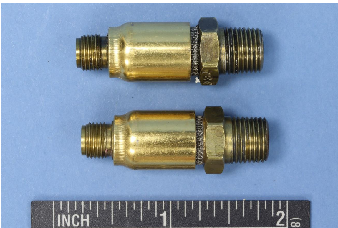
Figure 1 (cont.): e) number 3 cylinder injector fuel line; f) numbers 3 and 4 fuel injectors;
