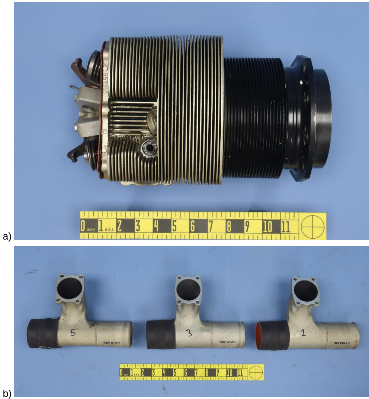
Figure 1: Images of accident parts as received: a) number 3 cylinder assembly; b) numbers 1, 3, and 5 intake elbow tubes;
