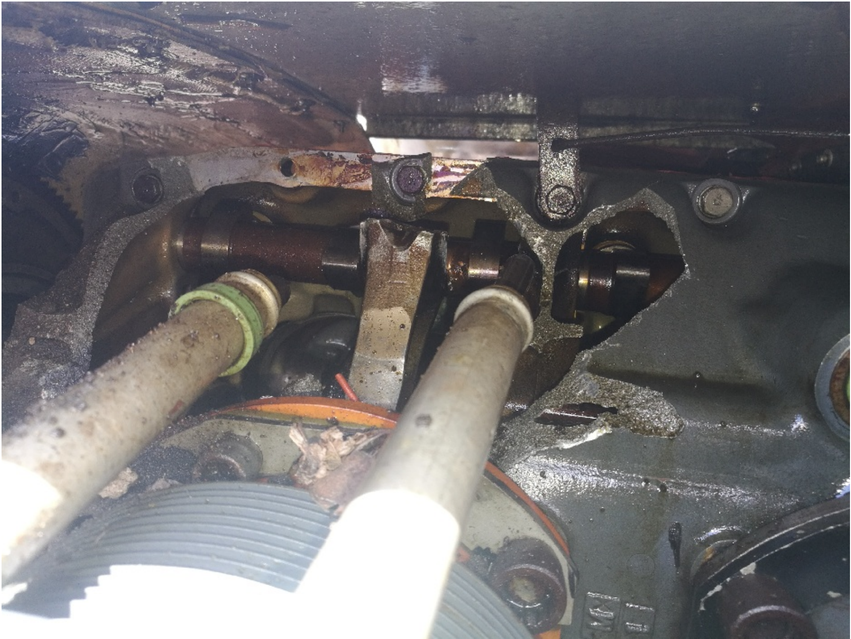
Photo 2 – Airplane engine showing hole in engine case
