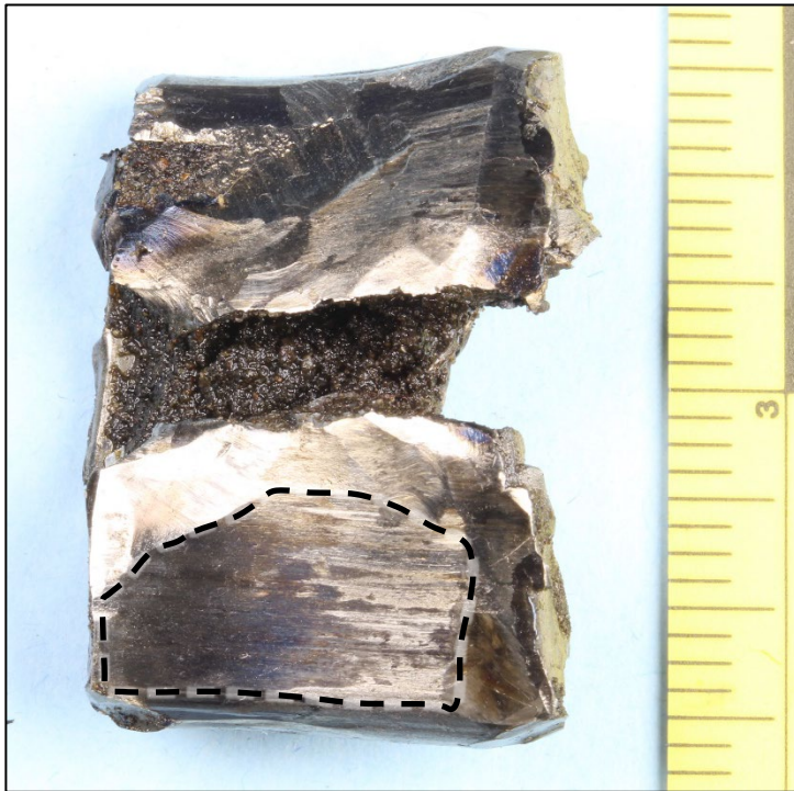
Figure 5. Bearing contact face on the connecting rod strap piece showing heat tinting and circumferential sliding contact marks in the area outlined with a dashed line.
