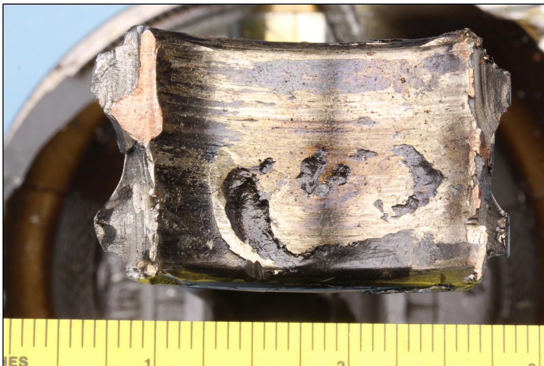
Figure 4. Bearing contact face on the connecting rod strap showing heat damage, circumferential sliding marks, and galled bearing material on the surface.
