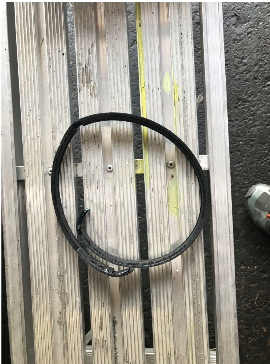
Photo 8 – Failed Alternator Belt
