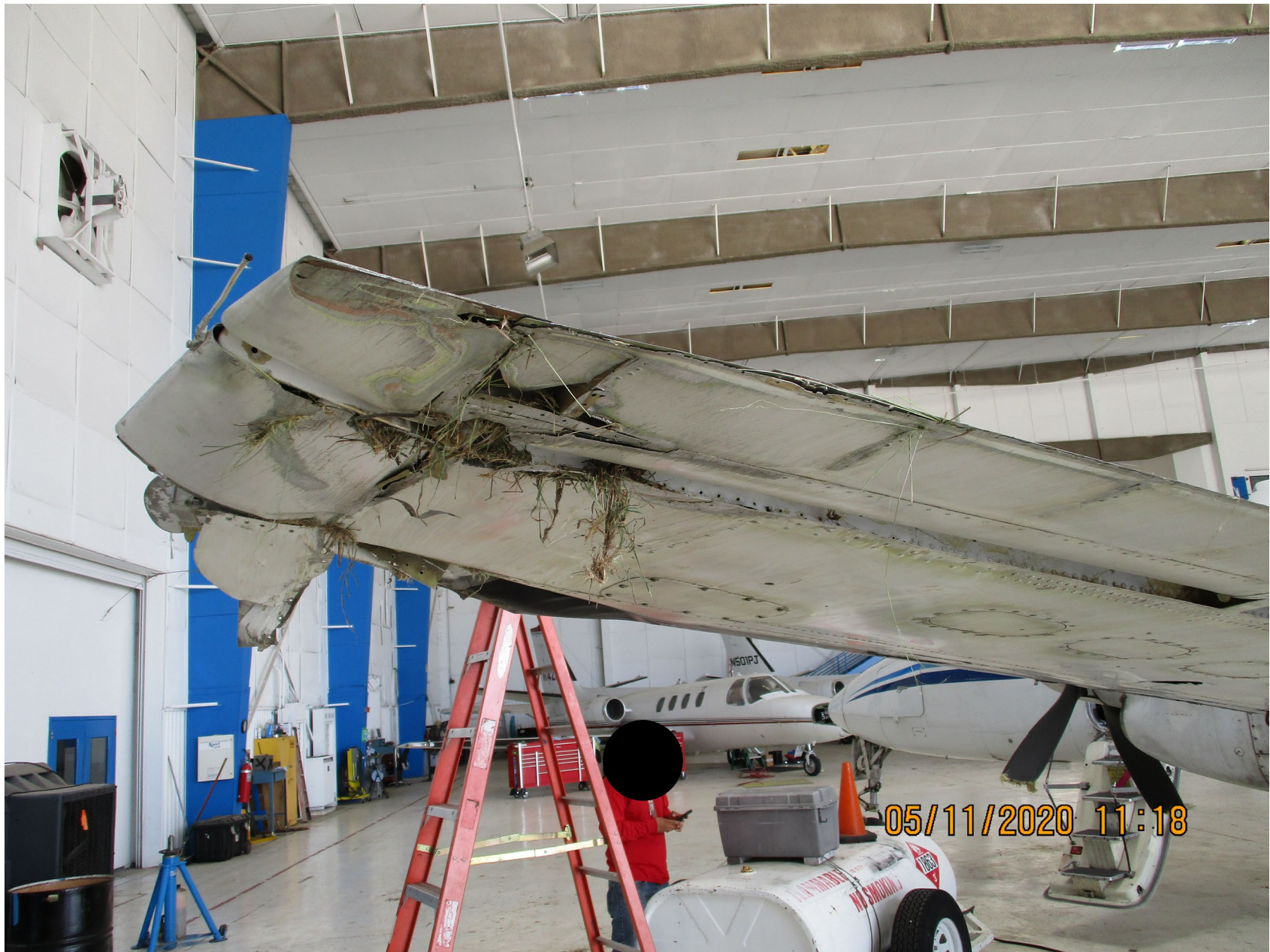
Photo 5 – View of the substantial damage sustained to the left wing (courtesy of the Federal Aviation Administration).
