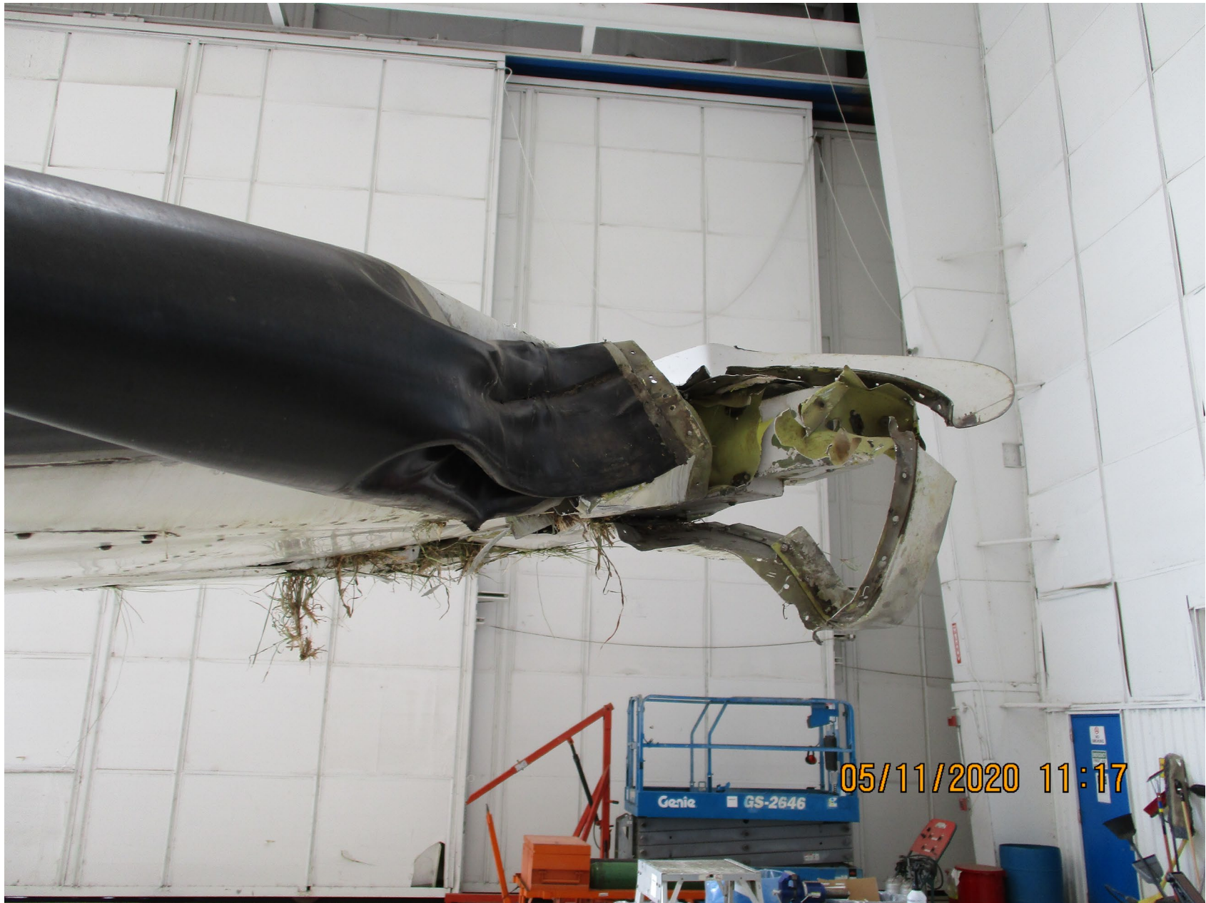
Photo 4 – View of the substantial damage sustained to the left wing (courtesy of the Federal Aviation Administration).
