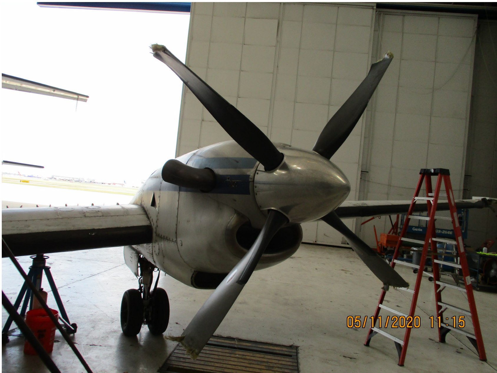
Photo 2 – View of the damage sustained to the left propeller (courtesy of the Federal Aviation Administration).
