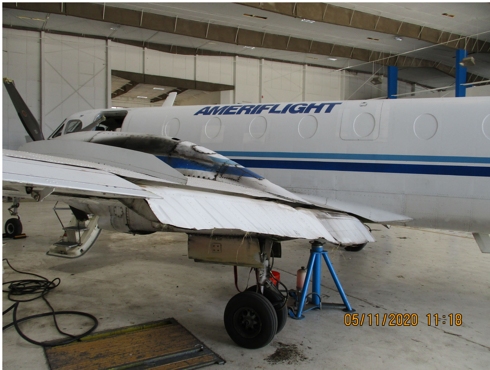
Photo 3 – View of the damage sustained to the left flap (courtesy of the Federal Aviation Administration).
