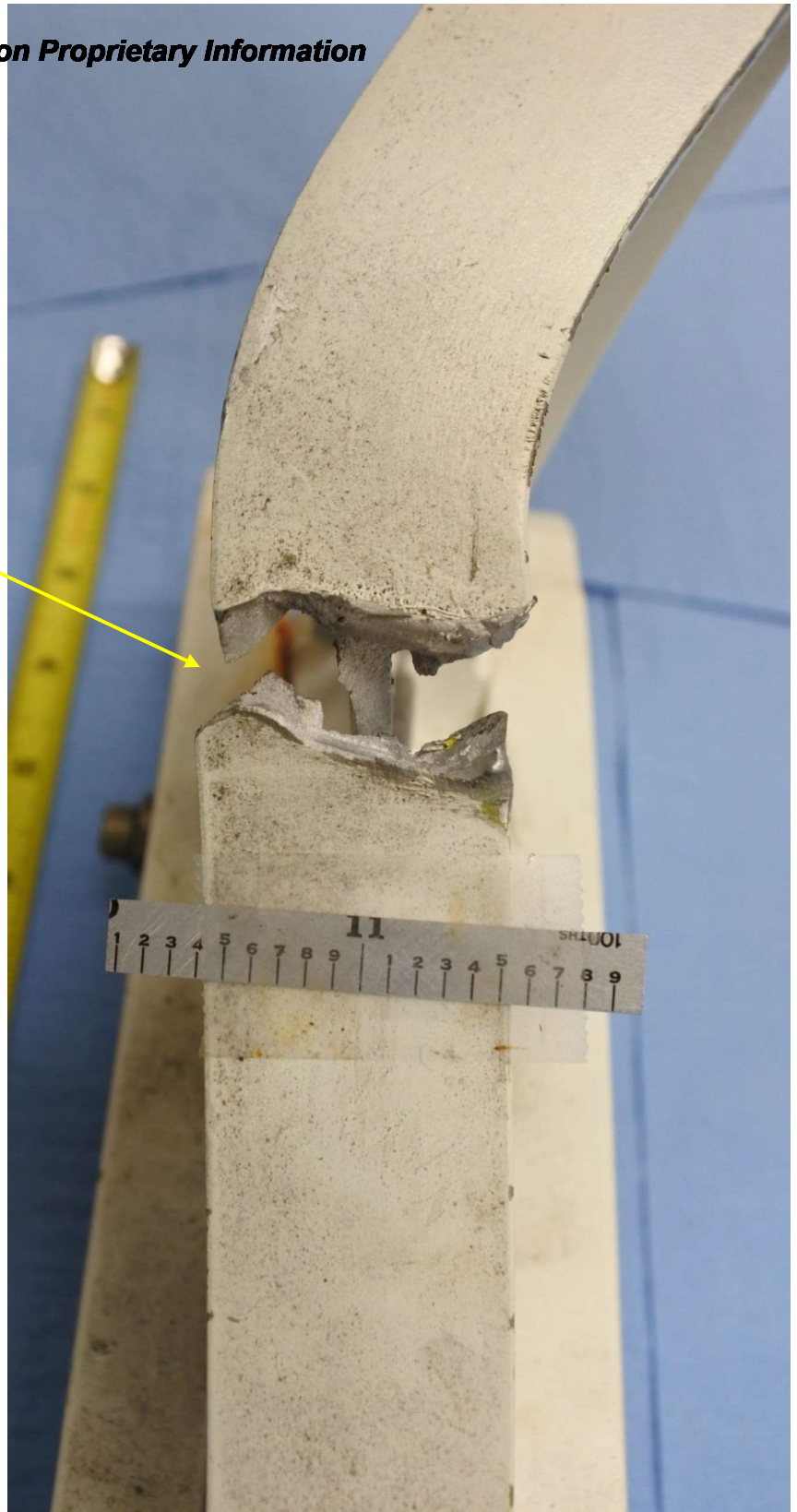
Figure 4 View showing inbd and outbd bending of the fractured upper drag leg arm. The flange width measured approximately 1.123" to 1.125" vs 1.120 +/- 0.010" required by the engineering drawing. Magnification: x0.2 and x1.7.
