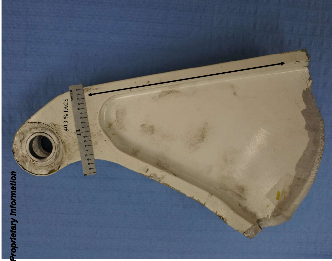
Figure 6 The paint and primer were cracked and peeled off from the part surfaces near the fracture area. Electrical conductivity measured higher near the fracture area, 42.1 % IACS. The typical electrical conductivity for 7075-T6 plate is 30.5 – 36.0 % IACS. Black arrow depicts tensile specimen location on the flange. Magnification: x1.1.
