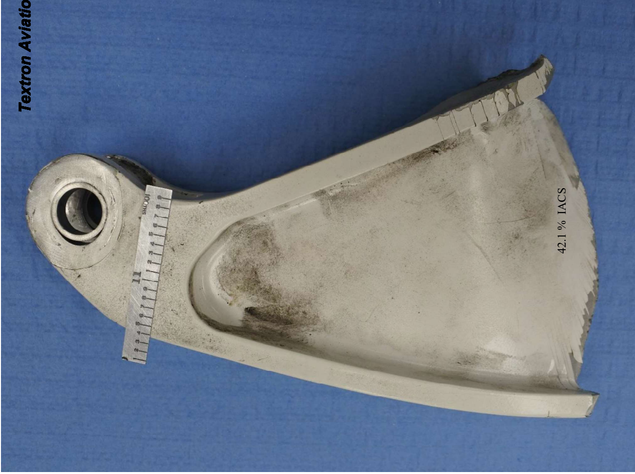
Figure 6 The paint and primer were cracked and peeled off from the part surfaces near the fracture area. Electrical conductivity measured higher near the fracture area, 42.1 % IACS. The typical electrical conductivity for 7075-T6 plate is 30.5 – 36.0 % IACS. Black arrow depicts tensile specimen location on the flange. Magnification: x1.1.
