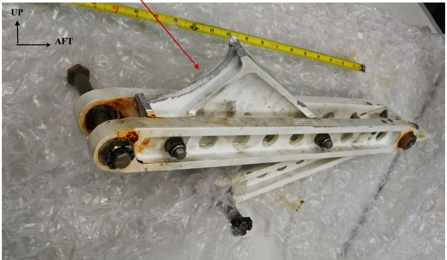
Figure 3 View showing contents of the box in Figure 2. The upper drag leg arm p/n 114-810026-1 was broken into two pieces fwd of a stiffening web as shown by red arrows. Magnification: x0.3.
