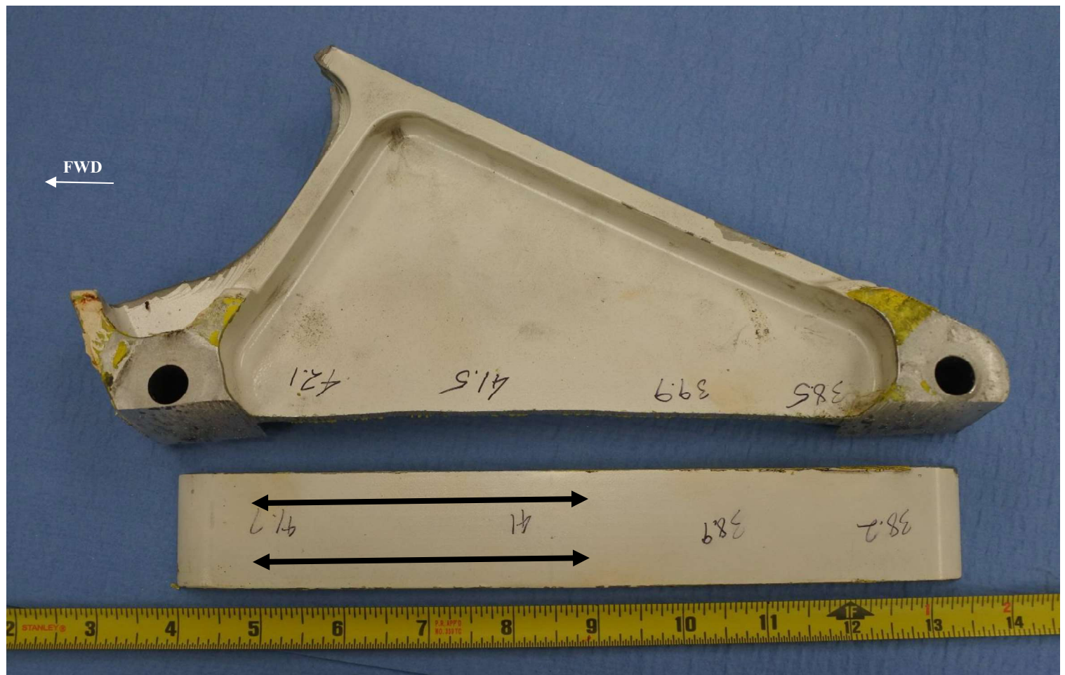
Figure 11 View of the opposing fractured piece showing location of the two new compact tensile specimens on the bottom flange. Consistent with previous conductivity measurements in Figure 6 the conductivity was higher near the fracture area and lower away from it; measurements indicated (38.2 to 42.1) % IACS in the area between the two holes. Black arrows depict location of the two new tensile specimens.
