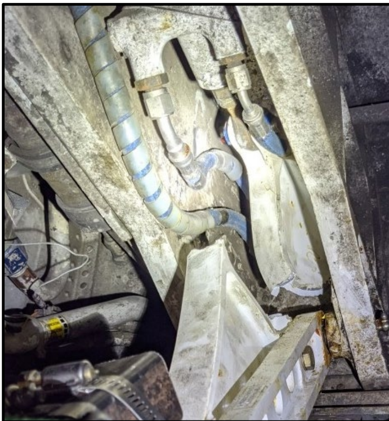
Figure 3-Fractured left Upper Drag Leg Arm on accident airplane.
