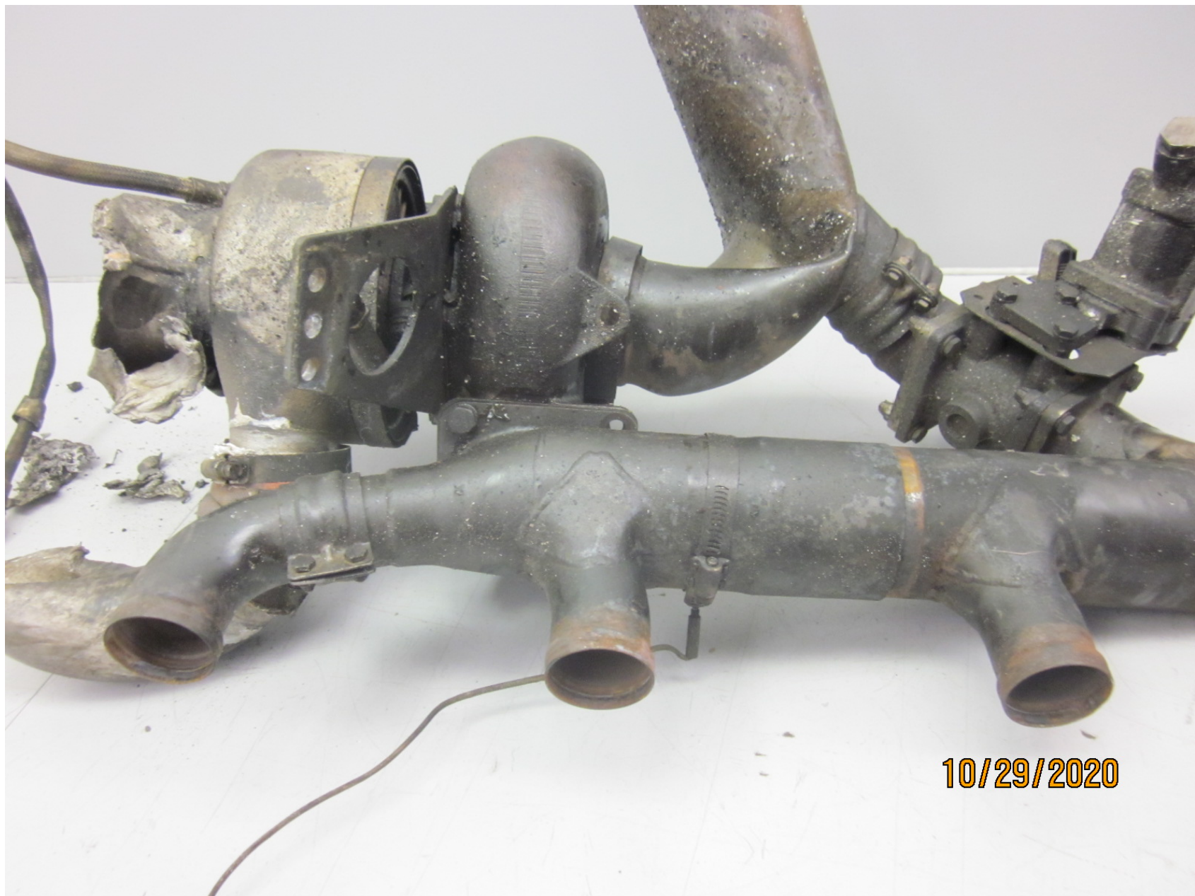
Photo 7 – Turbocharger, wastegate, and exhaust manifold (FAA photo)
