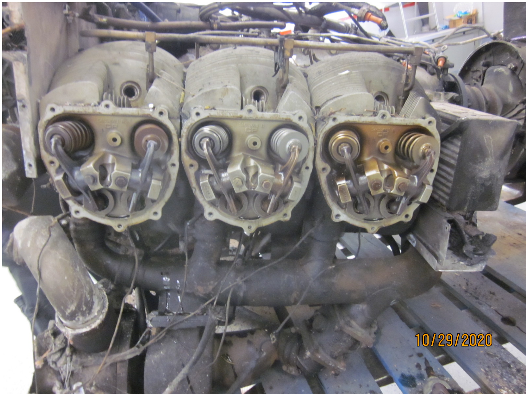
Photo 2 – Engine cylinder head after spark plug removal (FAA photo)
