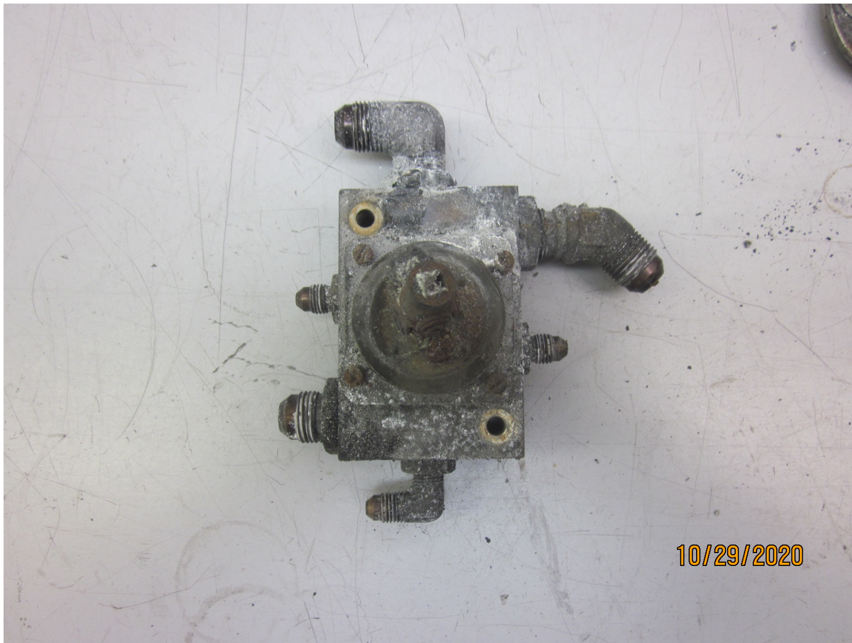
Photo 4 – Fuel selector valve (FAA photo)
