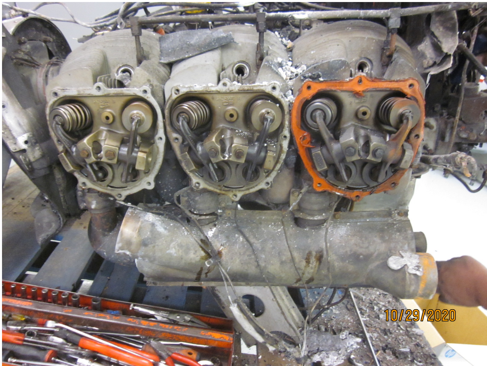
Photo 3 - Engine cylinder head after spark plug removal (FAA photo)
