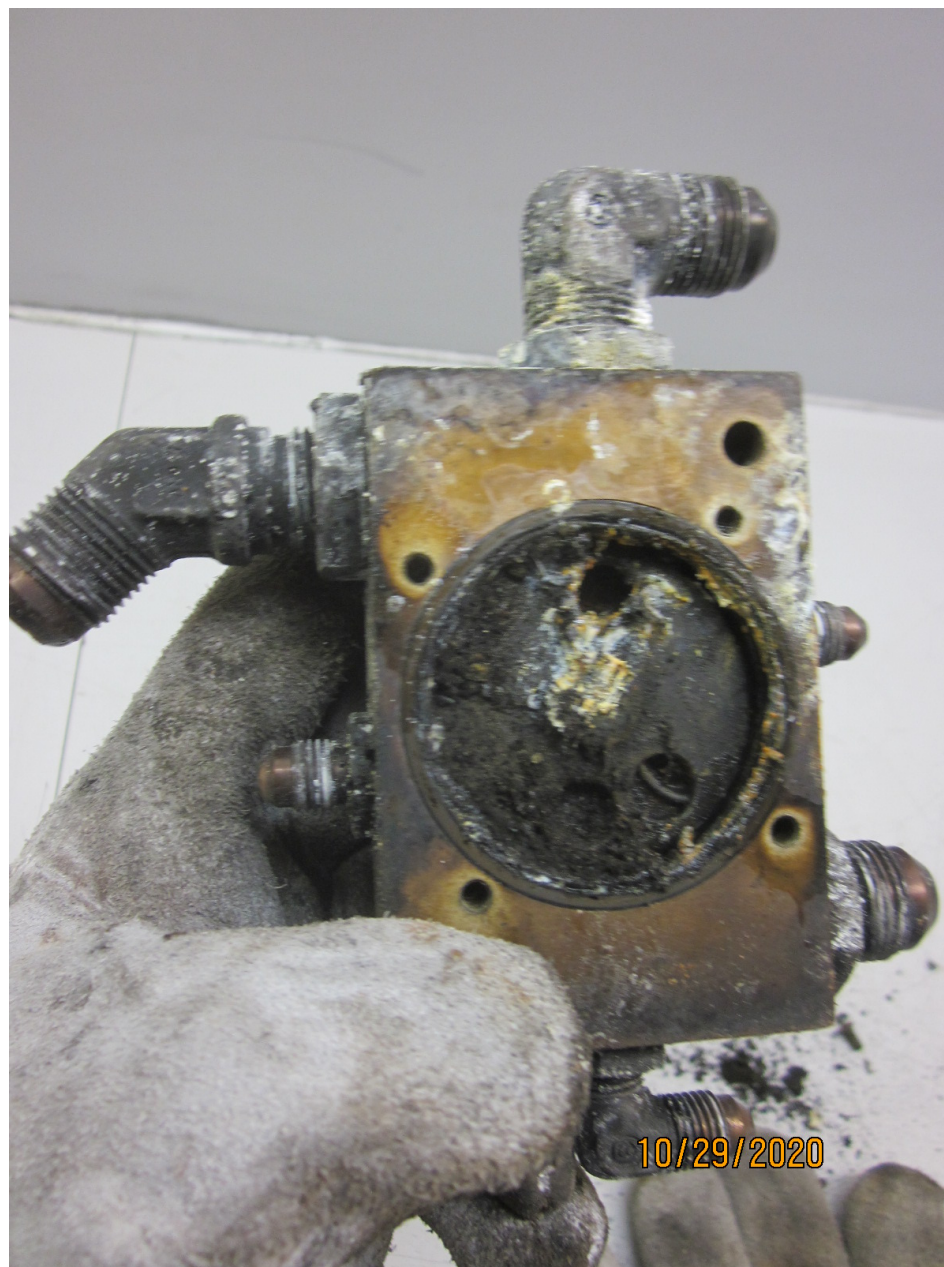
Photo 5 – Fuel selector valve (FAA photo)
