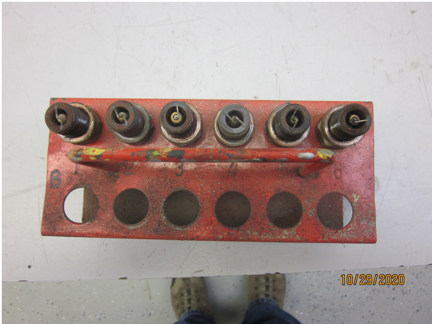
Photo 1 – Top spark plugs after removal from cylinder heads (FAA photo)
