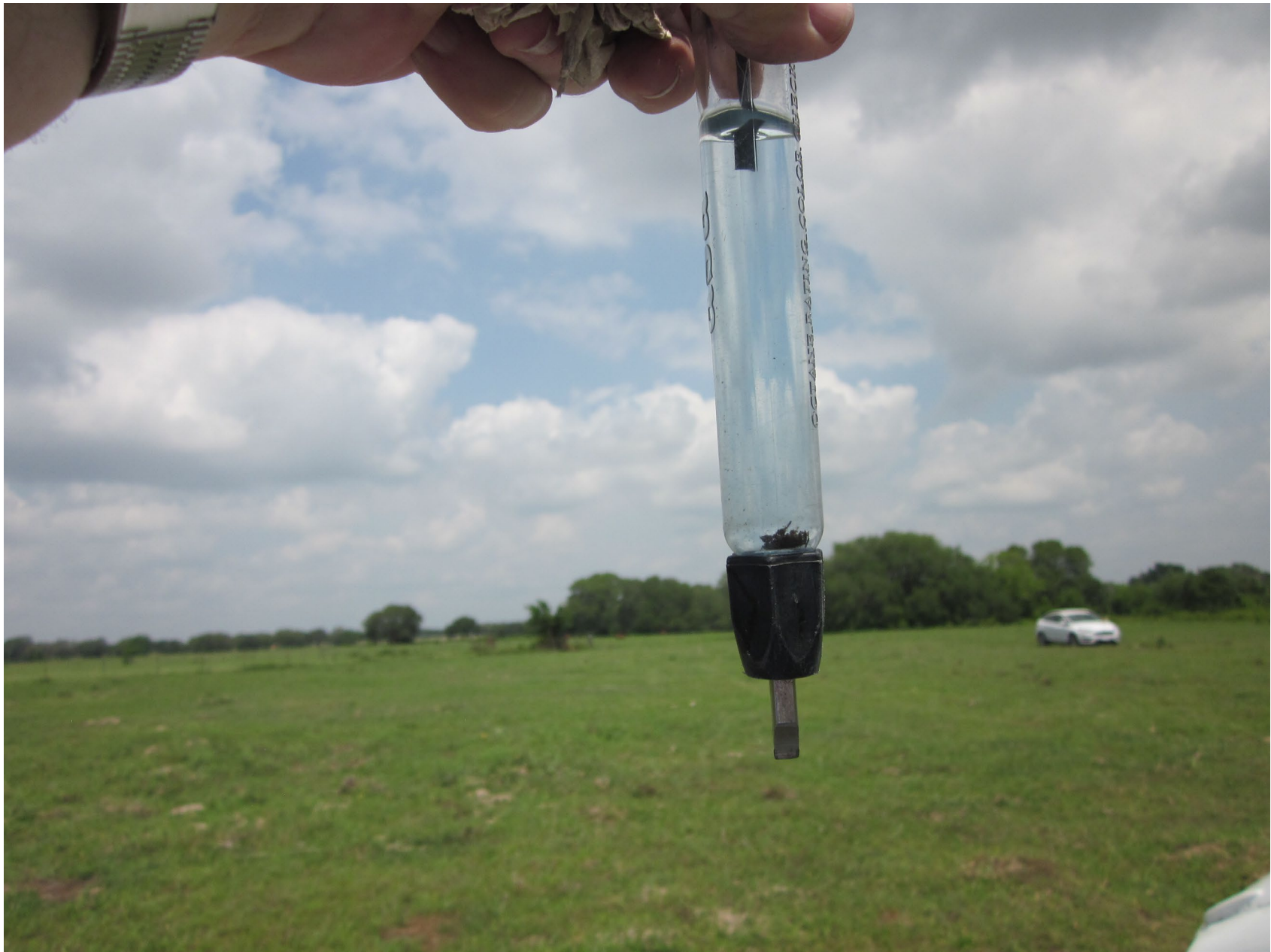
Photo 3 - Fuel Contamination Found in Left Wing Tank Fuel Sample (Source: FAA)
