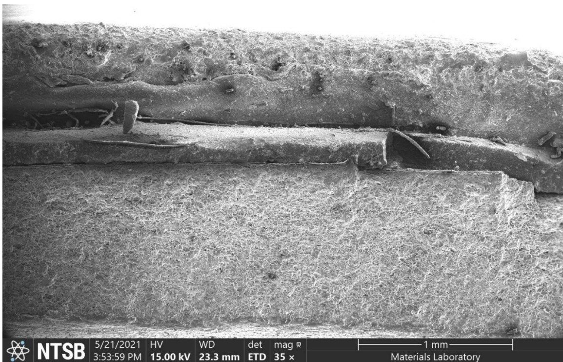
Figure 17 – SE micrograph of the fractured adhesive between the cylindrical outer sheath and the fractured shaft on the compressive side.
