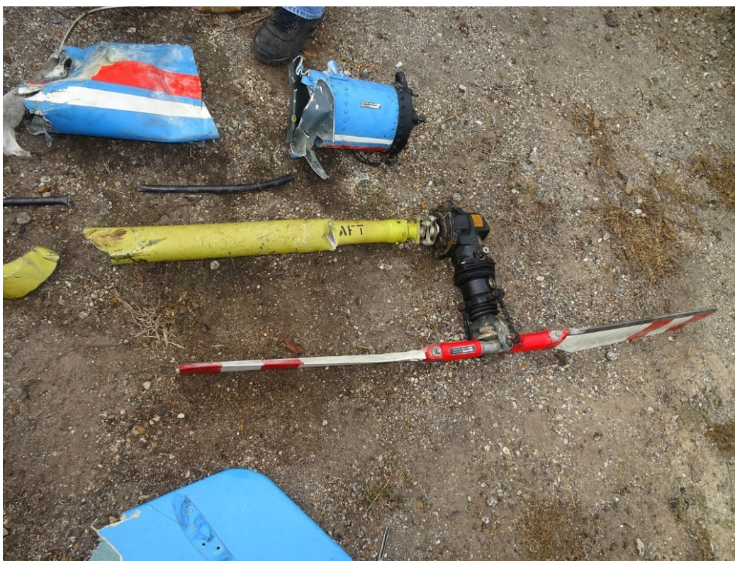
Figure 11. The aft TRDS segment leading to the tail rotor gearbox.
