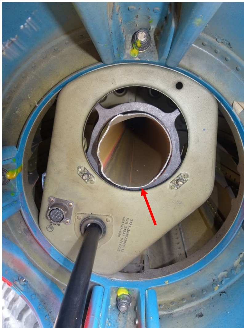
Figure 7. The TRDS fracture (red arrow) near the dampener within the tail boom.
