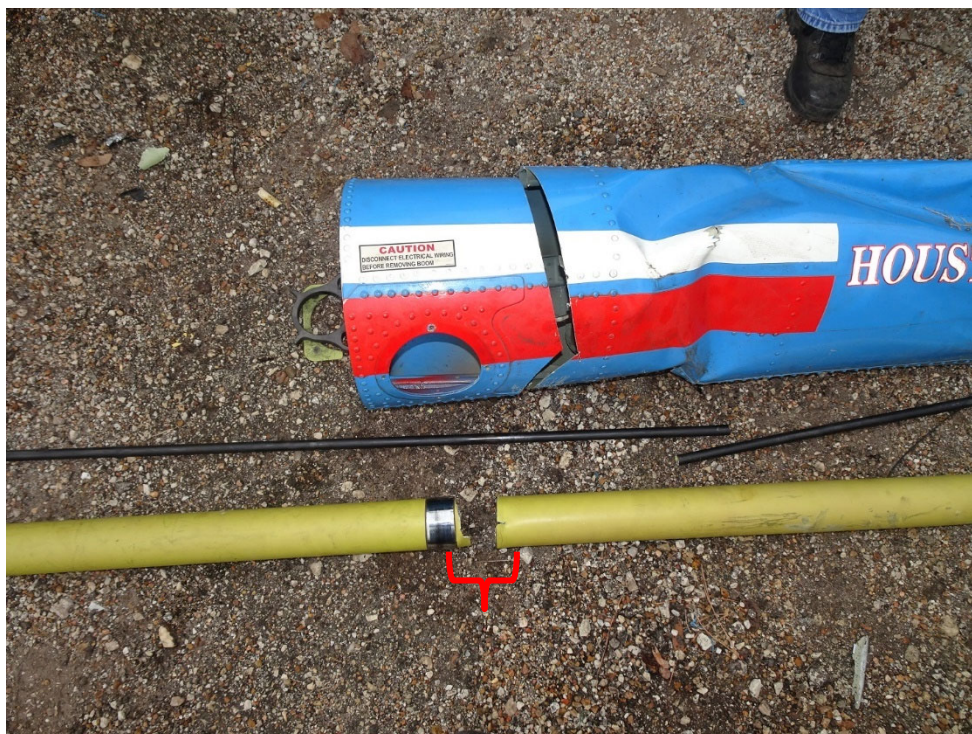
Figure 8. The TRDS fracture near the dampener (red bracket) after removal of the TRDS from the tail boom. The tail rotor control tube is seen above the TRDS.
