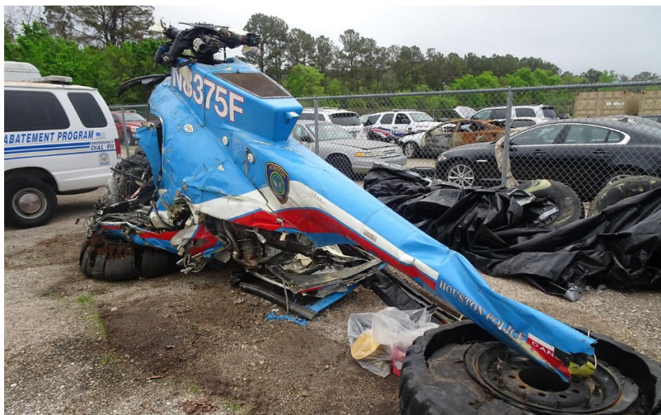
Figure 3. An aft view of the main wreckage showing deformation to the tail boom.
