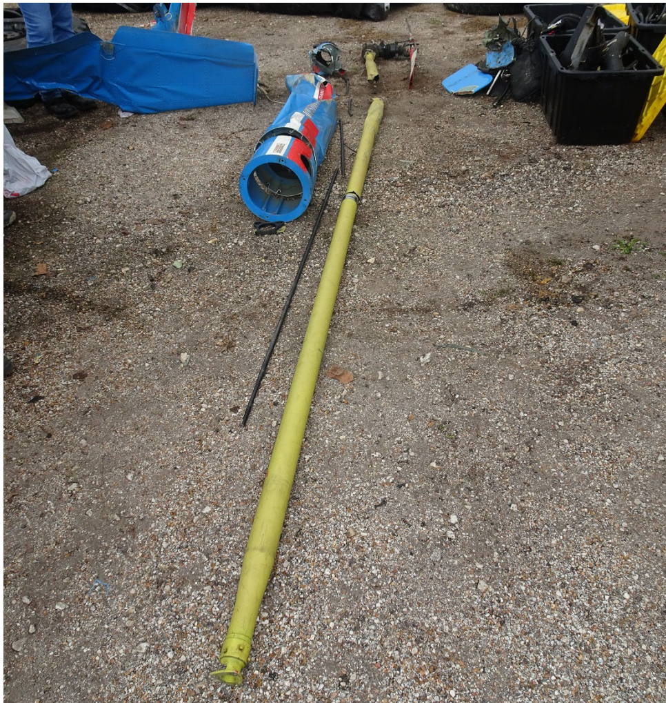
Figure 12. A view of the reconstructed TRDS after removal from the tail boom.
