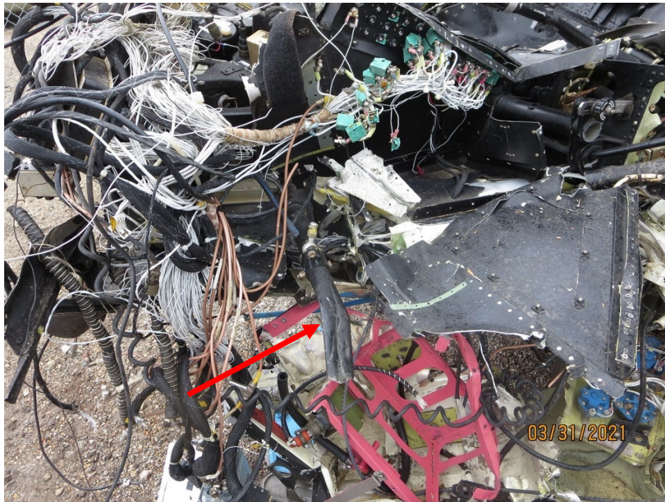
Figure 14. The red arrow points to the pedal torque tube as seen in the main wreckage. (Image courtesy of MD Helicopters Inc.)
