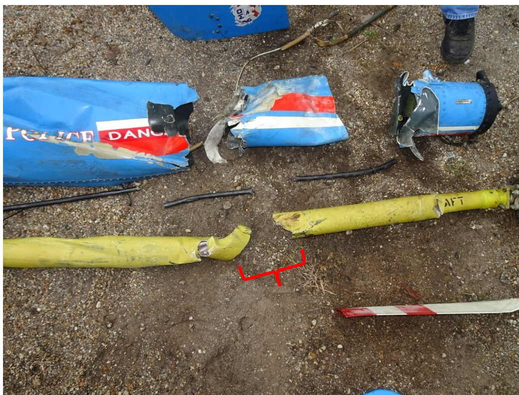
Figure 10. The TRDS fracture (red bracket) co-located with the aft tail boom separation.
