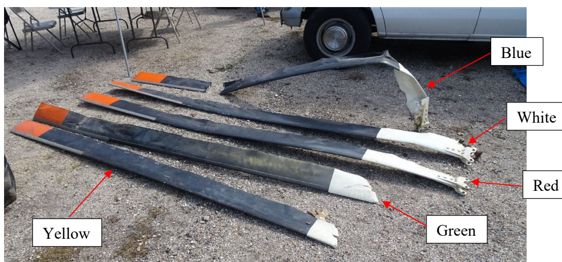
Figure 6. The five main rotor blades.
