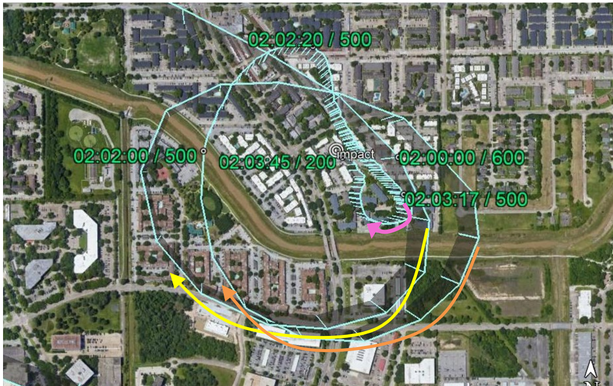
Figure 3. End of flight path. First right-hand turn at 600 ft msl indicated by yellow arrow, second right-hand turn at 500 ft msl indicated by orange arrow. The final right-hand turn is shown in pink.
