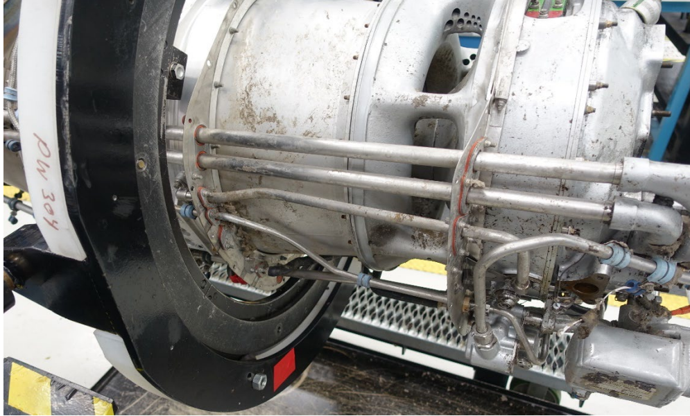
Photo 18- Engine Line Deformation, 6 o'clock Position
