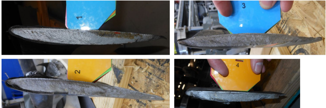
Photo 8- Propeller Blade Fracture Surfaces
