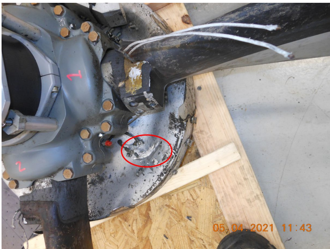
Photo 5- Spinner Bulkhead Impact Damage
