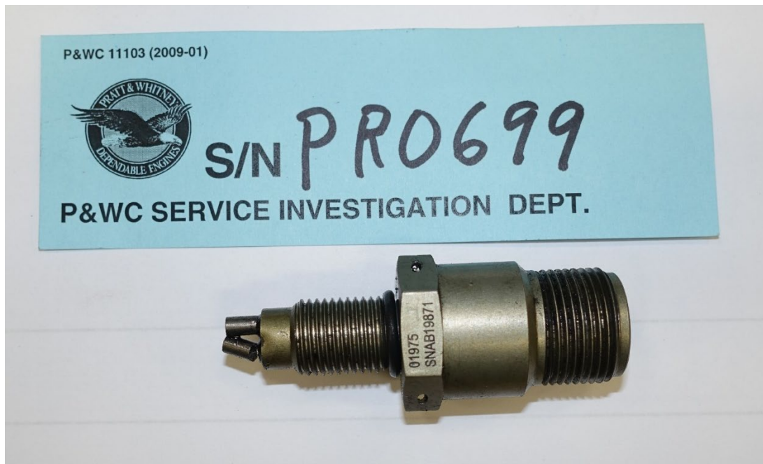
Photo 19- Magnetic Chip Detector (*Damaged During Removal)
