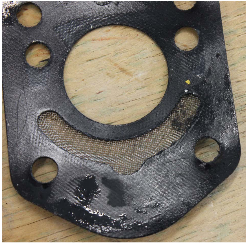
Photo 3: Propeller governor screen
