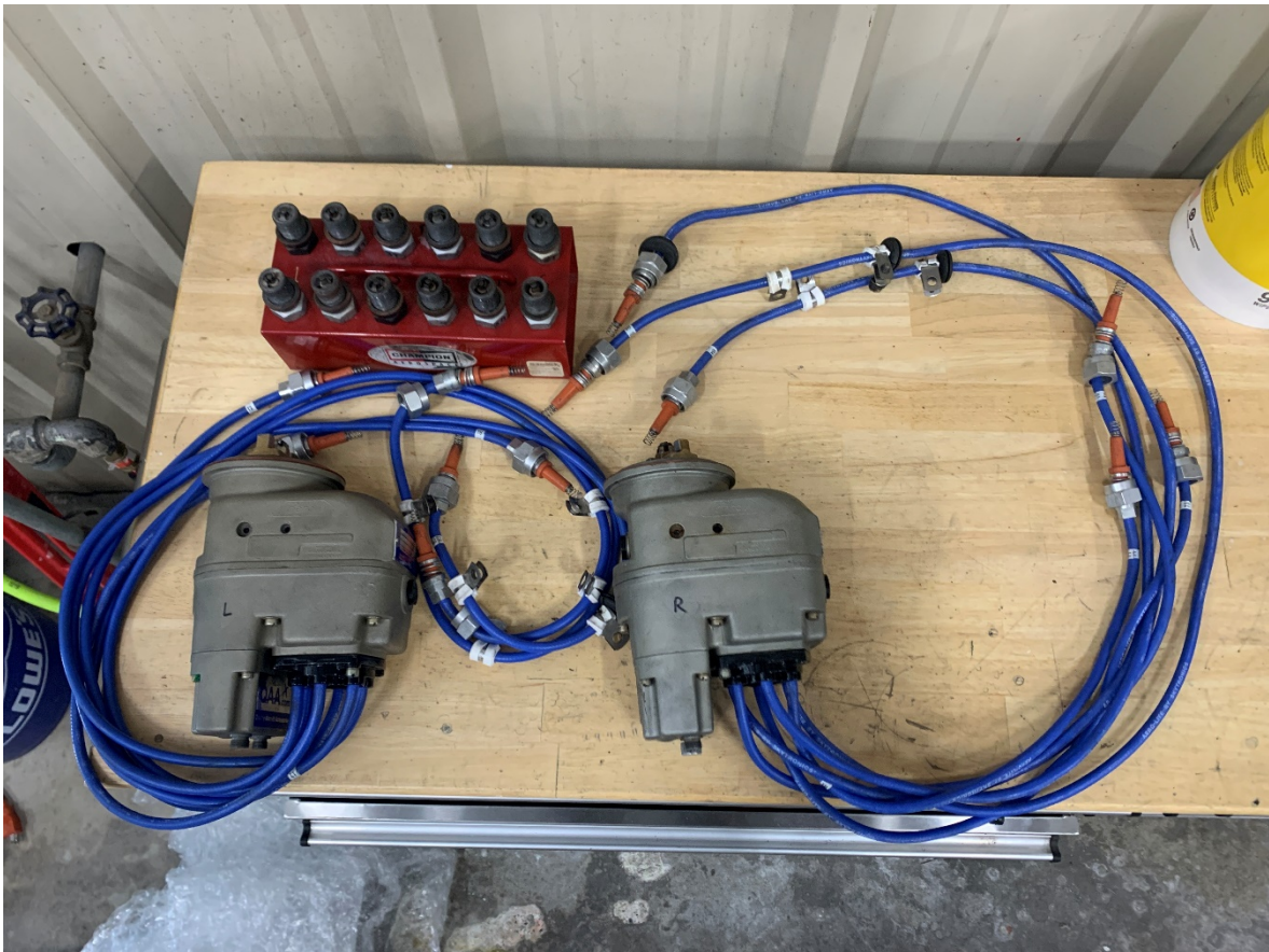
Figure 1: Left and right magnetos, and spark plugs, as received.
