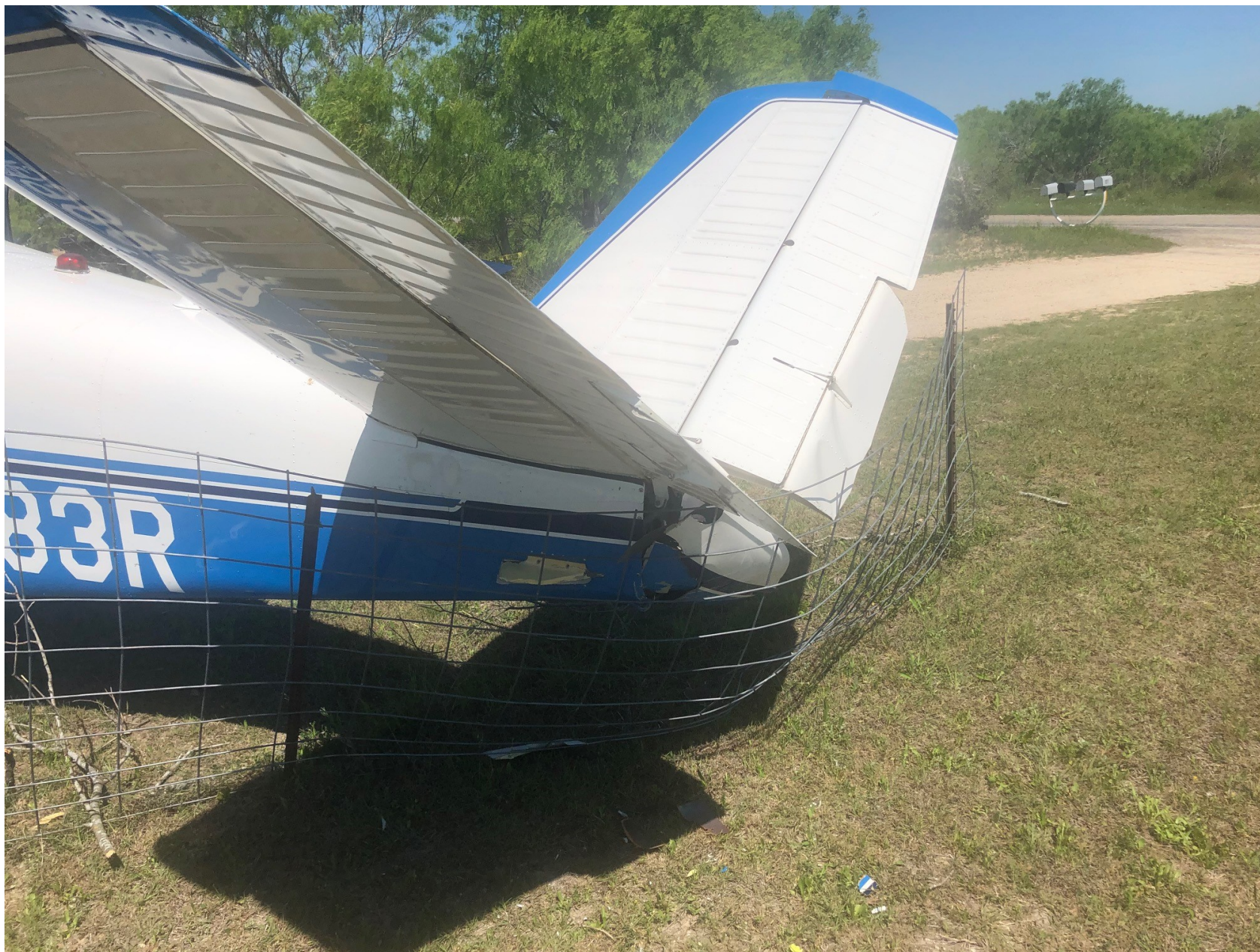
Photo 5 – View of the empennage at the accident site (courtesy of the Federal Aviation Administration).
