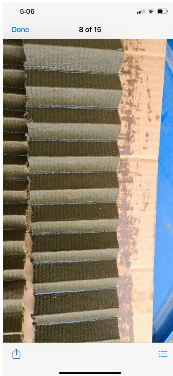
Photo 7 – View of the cut open engine oil filter (courtesy of Wentworth Aircraft, Inc.).
