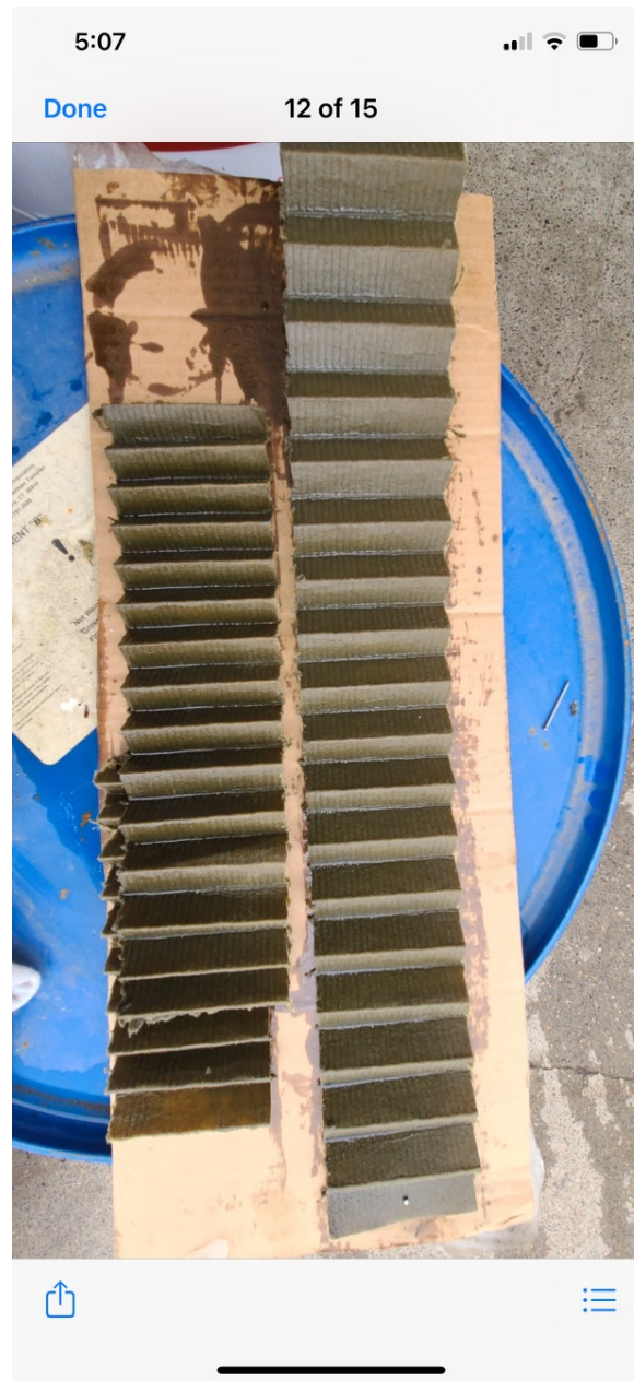
Photo 8 – View of the cut open engine oil filter (courtesy of Wentworth Aircraft, Inc.).
