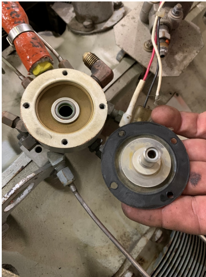
Figure 8: Internal Components of Fuel Manifold Valve
