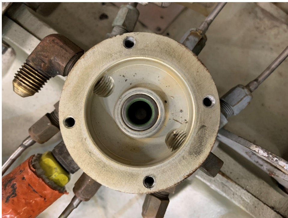
Figure 9: Debris inside of Fuel Manifold Valve
