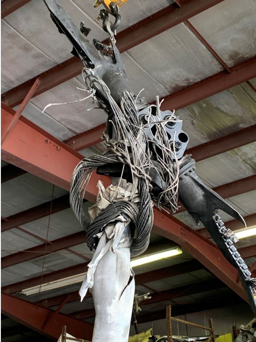
Figure 2: View of powerline wires wrapped around rotor head
