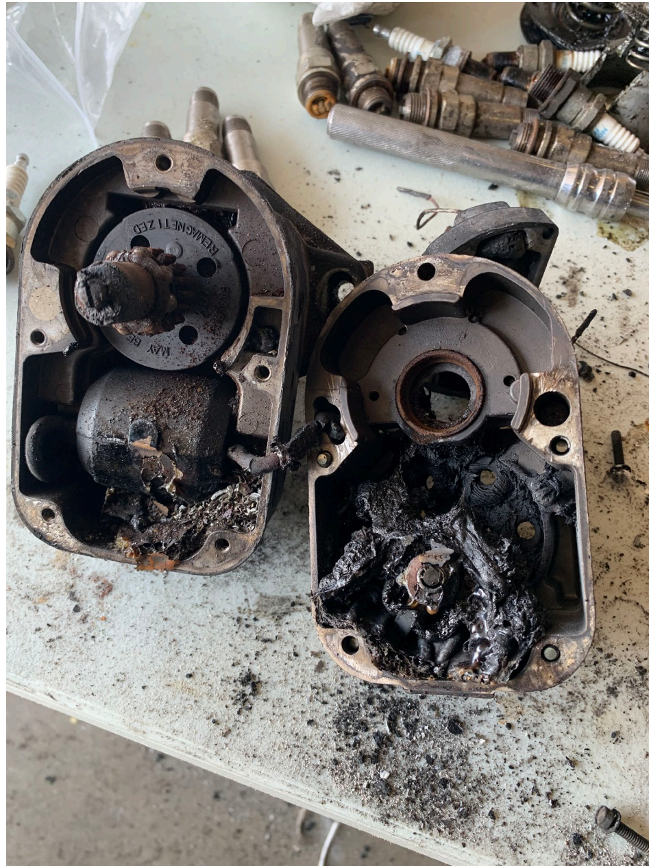
Photo 8 - First magneto during postaccident examination (NTSB Photo)
