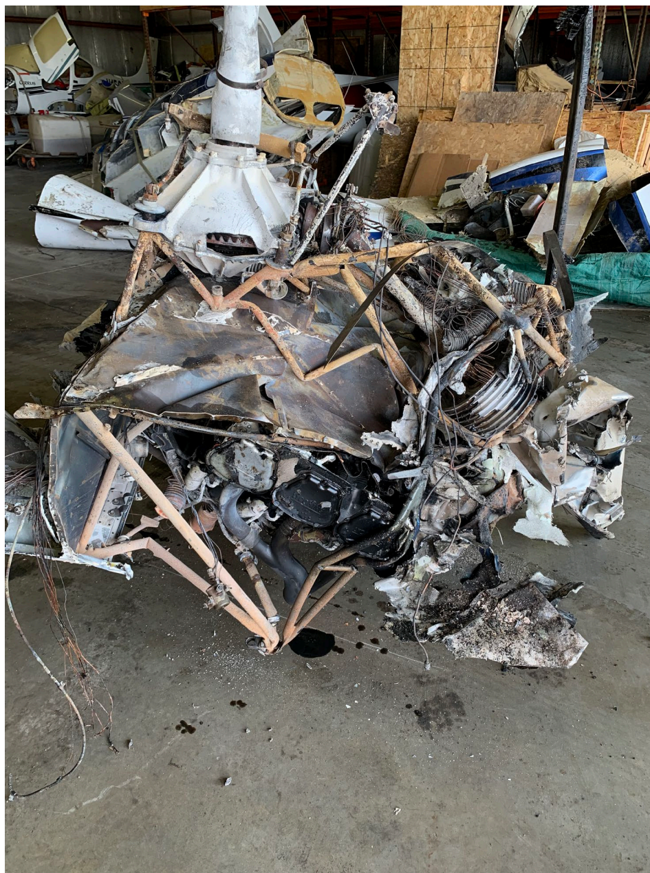
Photo 6 – Engine, fuselage cage, and gearbox during postaccident examination (NTSB Photo)
