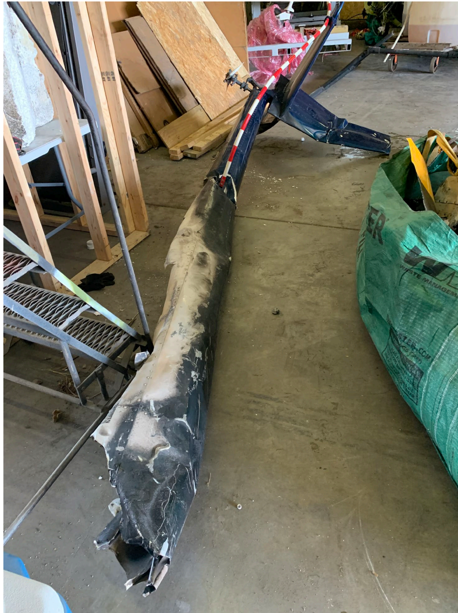
Photo 5 – Tail boom and tail rotor during postaccident examination (NTSB Photo)
