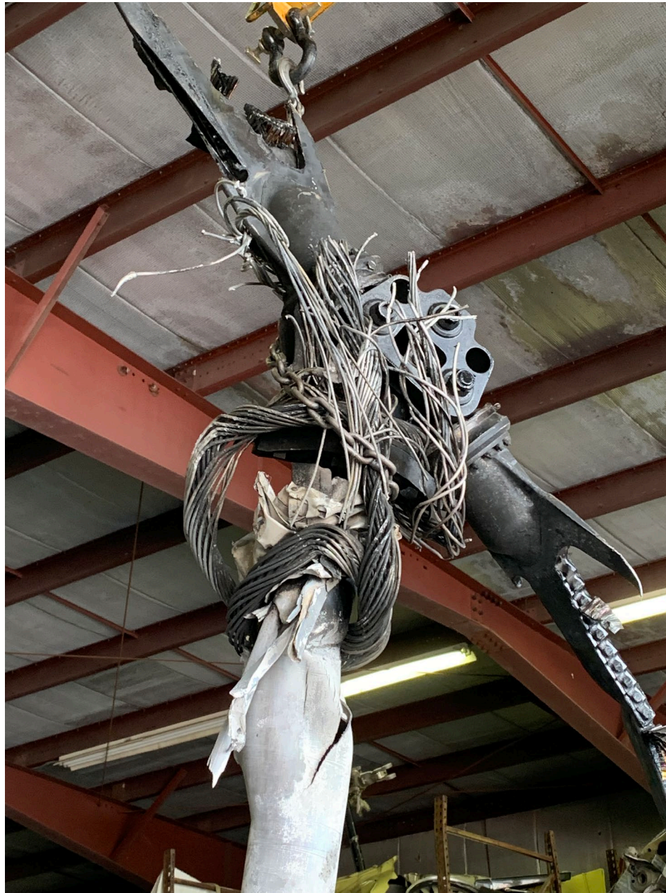
Photo 7 – Rotor mast and rotor head during postaccident examination (NTSB Photo)
