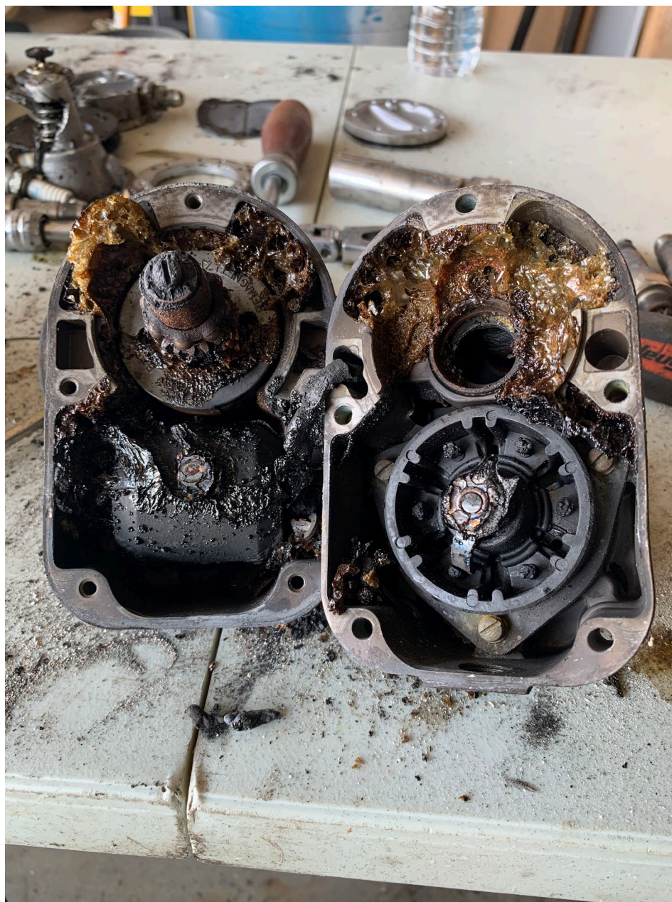
Photo 9 – Second magneto during postaccident examination (NTSB Photo)
