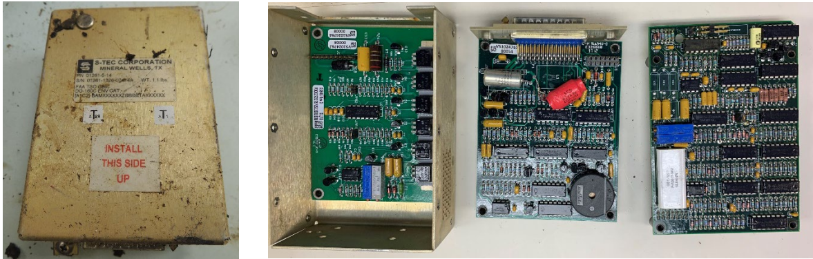
Figure 4. S-Tec Pitch Computer as received (left). Internal components (right).
