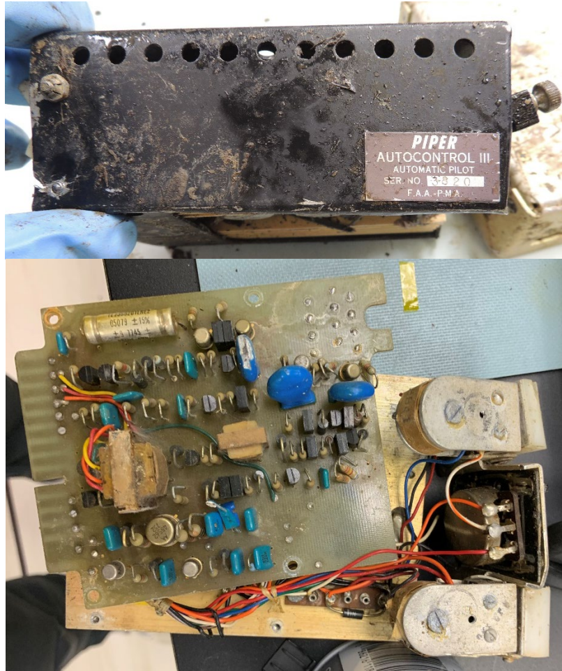
Figure 6. Piper Autocontrol III as received (top). Internal components (bottom).
